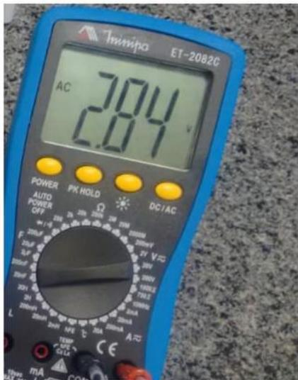
$$I_{rms} = \sqrt{\langle I^2 \rangle} = \sqrt{\frac{1}{T} \int_0^T I_p^2 \cos^2(\omega t) dt} = \frac{I_p}{\sqrt{2}}$$
