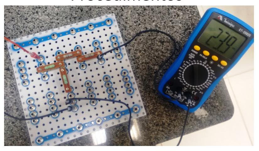
Item 8:  $R_c = 47 \Omega$   $i_c = 23.9 \text{ mA}$   $V_c = 1.13 \text{ V}$
