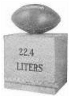
Fig. 19--The gram-molecular volume for an ideal gas under standard conditions.
