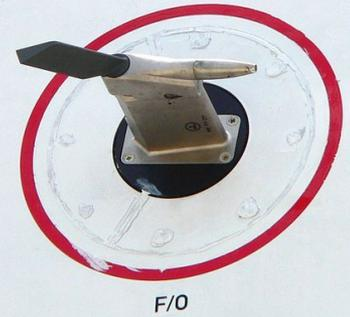
Pitot tube for Airbus A380, together with an angle-of-attack vane (left). Air-flow is right to left.
