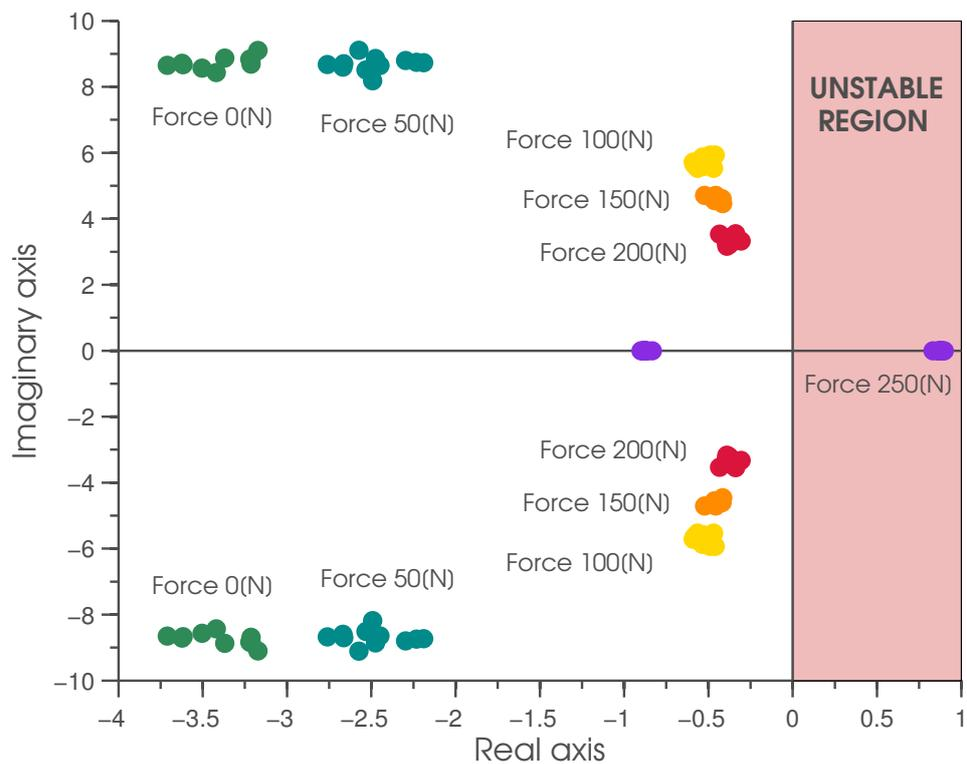
Figure 4.10: Estimation of poles of the Roll dynamics with RCP. For each lateral force applied to the robot, the poles estimated in several experiments are shown.
