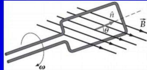
$$B = \frac{24 \text{ V}}{2\pi(300)(2.00 \times 10^{-2} \text{ m})(1.50 \times 10^{-2} \text{ m})(60 \text{ rev/s})} = \boxed{0.71 \text{ T}}$$
