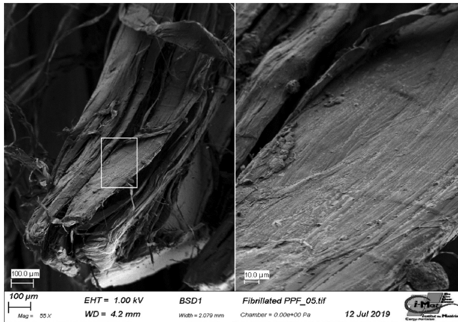
Fig. 3. SEM images of fibrillated twist PPF.
