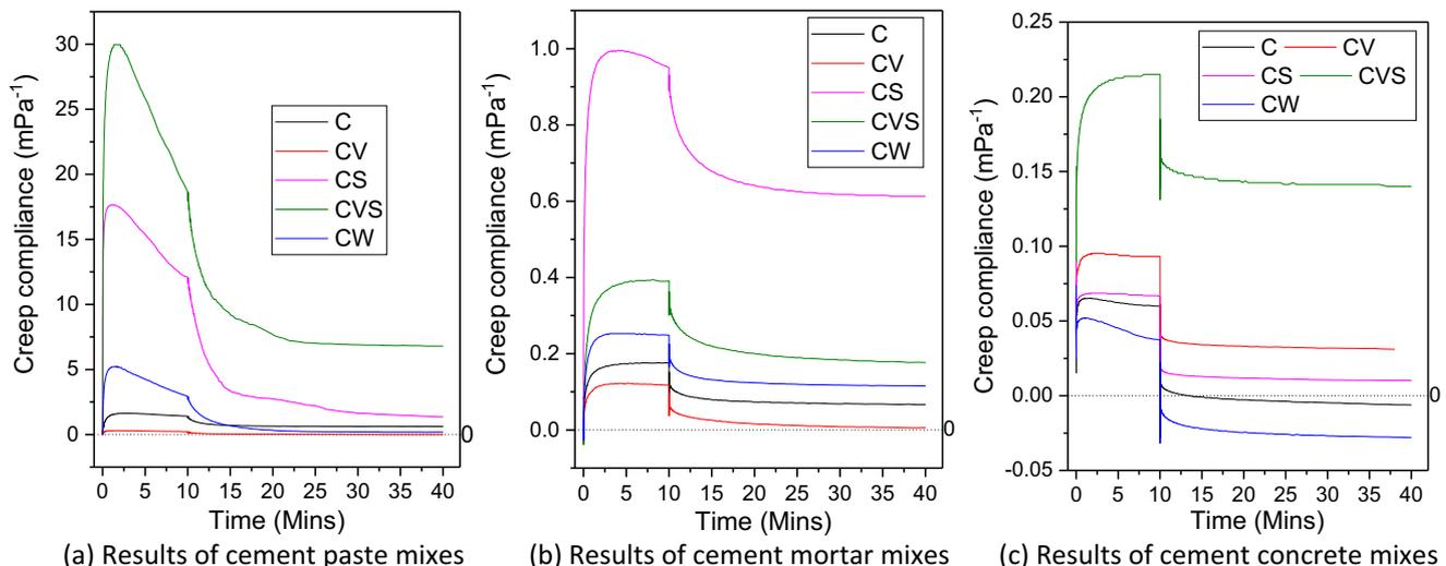
Fig. 10. Creep and creep recovery test results for the cement-based materials.
