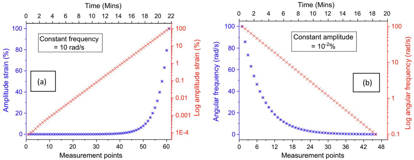
Fig. 5. Test protocol for the (a) amplitude sweep (b) frequency sweep.
