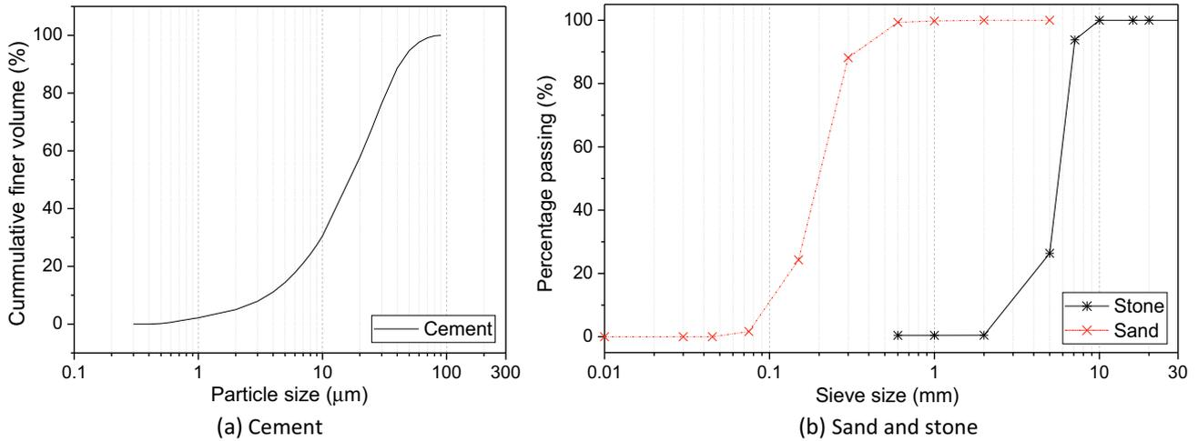
Fig. 3. Particle size distribution of the dry constituents.
