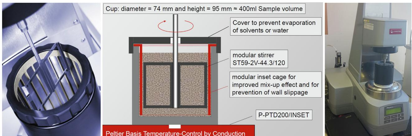
Fig. 2. Special building material cell (BMC 90) [46] and MCR 501 rheometer.
