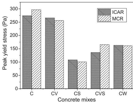
Fig. 4. Comparative results between the Germann ICiAR rheometer and Physical MCR501 rheometer [59].
