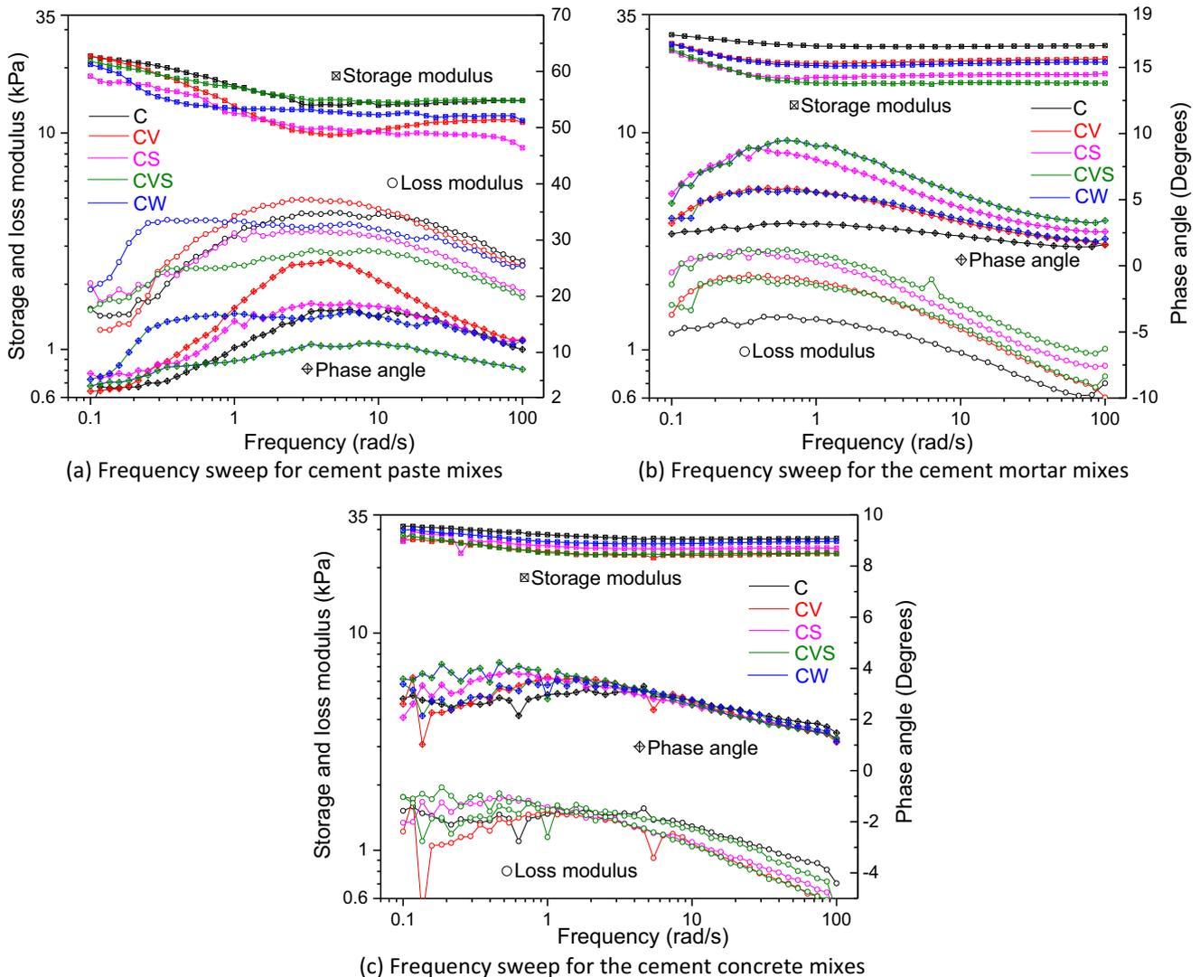
Fig. 9. Frequency sweep results of the cement-based materials.
