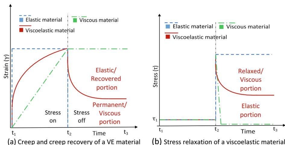
Fig. 1. Viscoelastic behaviour/response to a sustained shear strain and stress.
