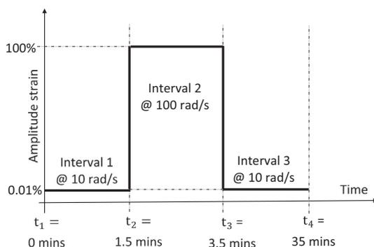
**Fig. 7.** Schematic test protocol for the 3ITT thixotropy test.
