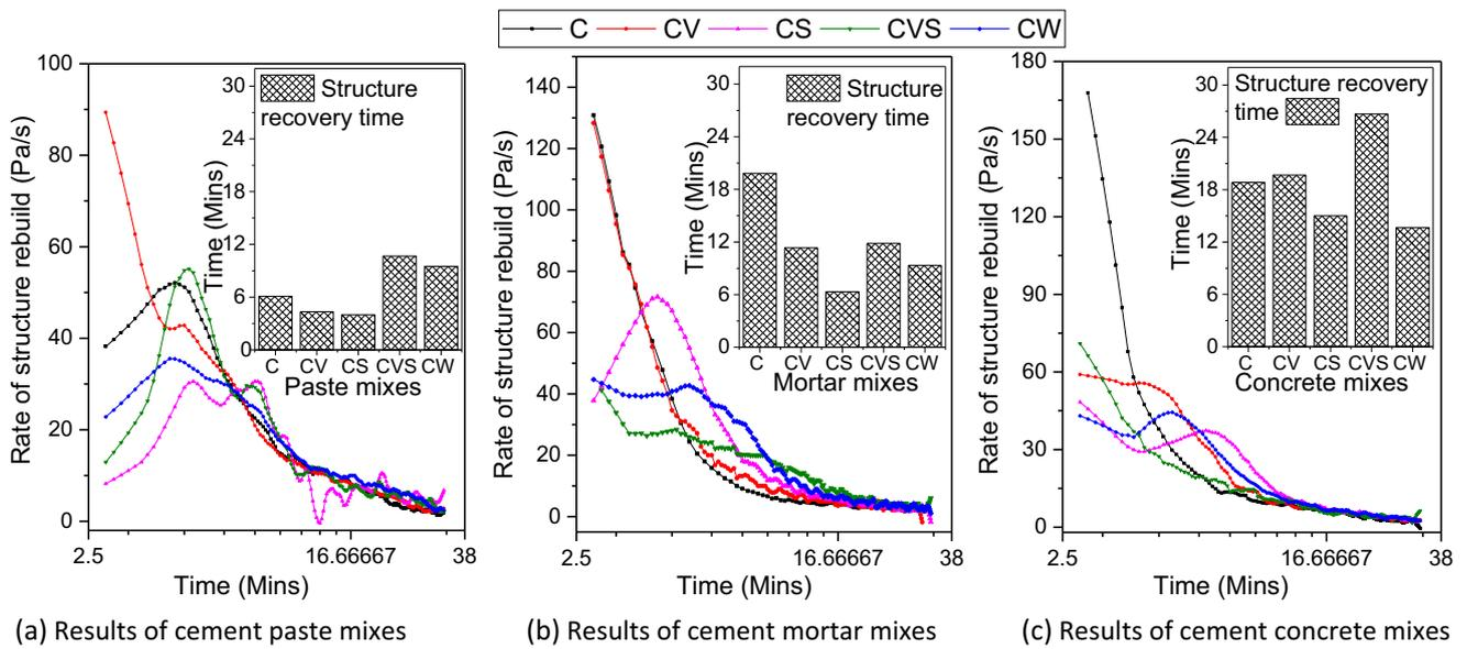
Fig. 15. Rate of restructuring and structure recovery time.
