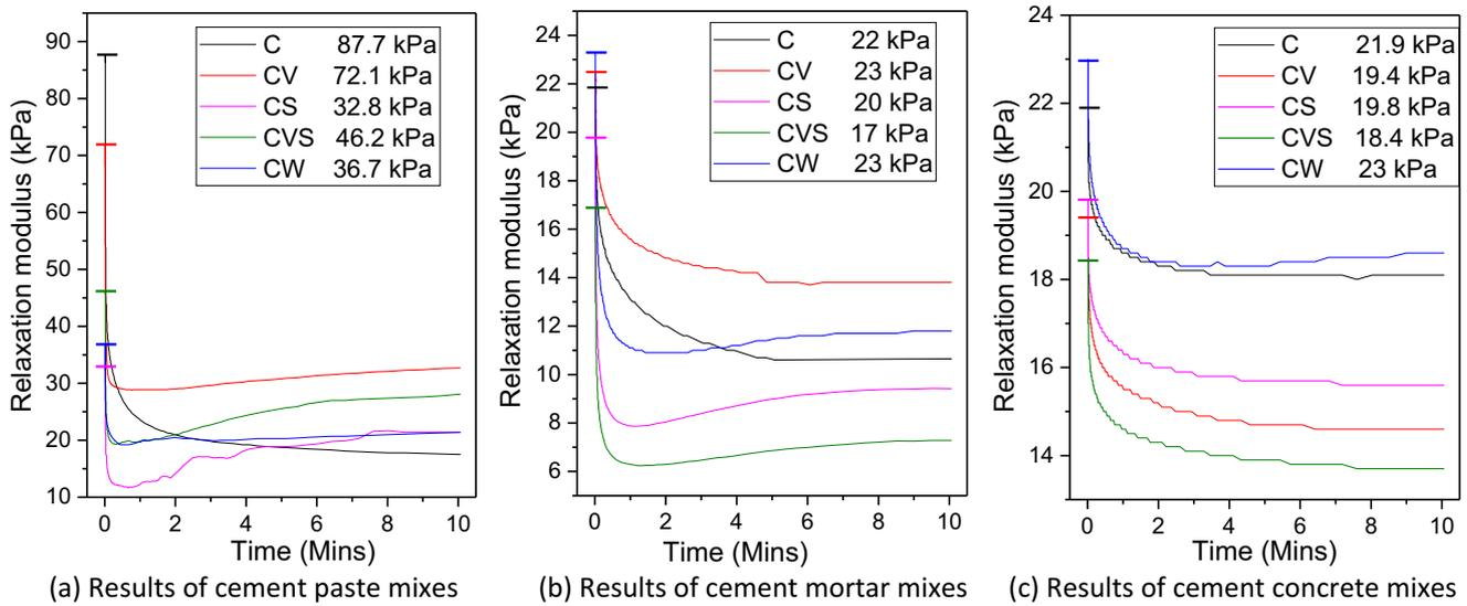
Fig. 12. Stress relaxation test results for the cement-based materials.
