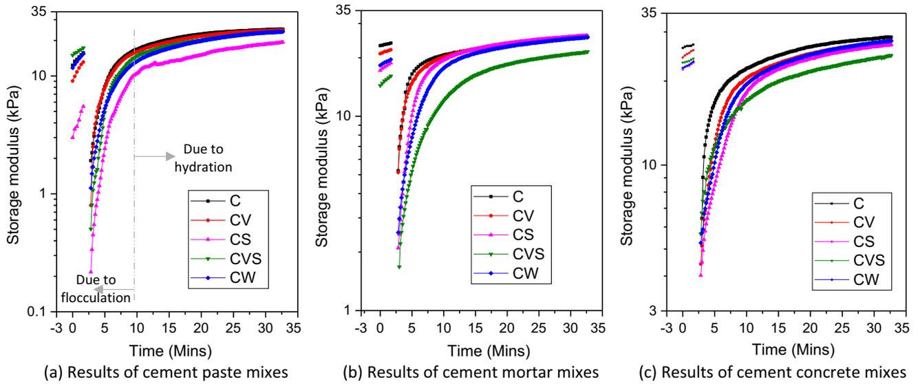
Fig. 14. Three interval thixotropy test results for the cement-based materials.
