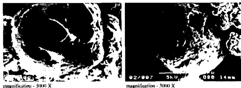
FIGURE 4 - SEM Micrographs of Sodium Alginate Spray Dried Microcapsules containing Allylguaiacol (from Silva and Ré (58))
