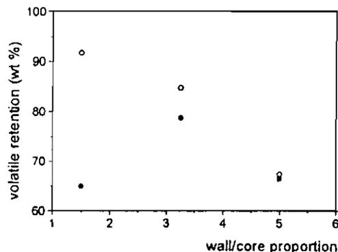
FIGURE 1 - Retention of Allylguaiacol by a Combined Matrix during Spray Drying Microencapsulation, as a Function of the Wall to Core Ratio. (o) - total oil retention; (●)-inner oil retention.: (Emulsion Composition: Maltodextrin/Modified Starch Matrix (3:1); 40% solids w/w . Drying Inlet Air Temperature: 130°C; data from Onimaru et al (40)).
