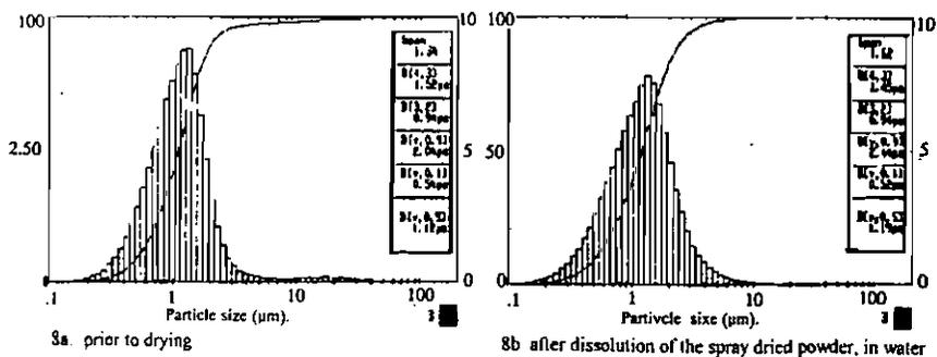
FIGURE 8 - Droplets Size Distribution of the Core Material, Before and after Drying (Emulsion Composition: Maltodextrin/Modified Starch Matrix - 3:1; Core Material (Allylguaiacol) Load - 24% w/w of wall solids; Total Solids Content - 40 % w/w. Drying Inlet Air Temperature: 130°C)
