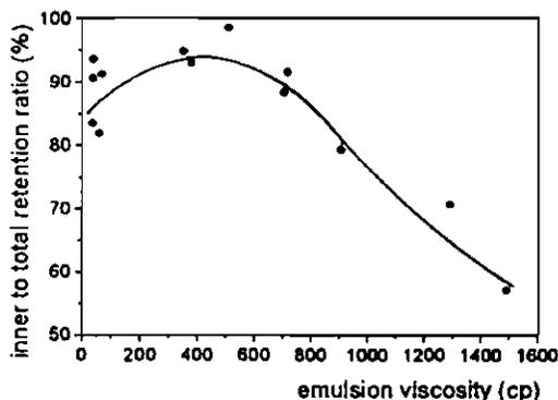
FIGURE 5 - Effect of the Emulsion Viscosity on the True Ability (Inner To Total Retention) of a Combined Matrix to encapsulate Allylguaiacol during Spray Drying.: (Emulsion Composition: Maltodextrin/Modified Starch Ratio - from 1.5:1 to 5:1; Core Material Load - from 15 to 40% w/w of wall solids; Total Solids Content - from 30 to 50% w/w. Drying Inlet Air Temperature: 130°C; data from Onimaru et al (40))
