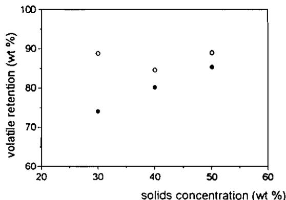
FIGURE 2 - Retention of Allylguaiacol by a Combined Matrix during Spray Drying Microencapsulation, as a Function of the Solids Content in the Emulsion. (o) - total oil retention; (•) - inner oil retention; (Emulsion Composition: Maltodextrin/Modified Starch Matrix (3:1); Wall to core material (3.2:1) . Drying Inlet Air Temperature: 130°C; data from Onimaru et al (40)
