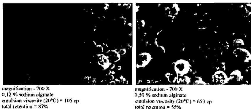
FIGURE 3 - SEM Micrographs of Spray Dried Microcapsules containing Allylguaiacol prepared from different Emulsion Viscosities (modified by adding a thickener)
