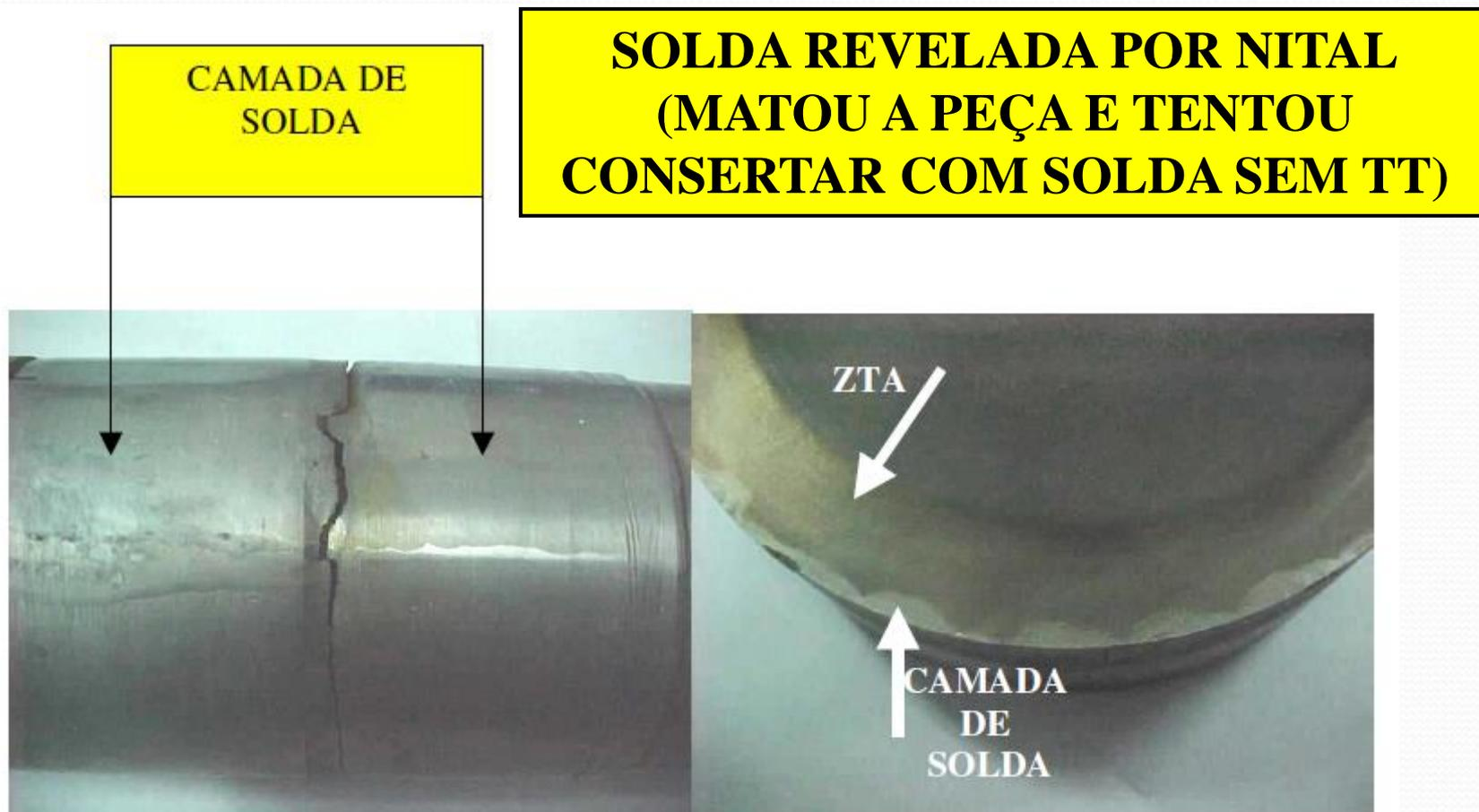
**ANÁLISE DE FALHAS – EIXO – AÇO SAE4140 – T+R -
