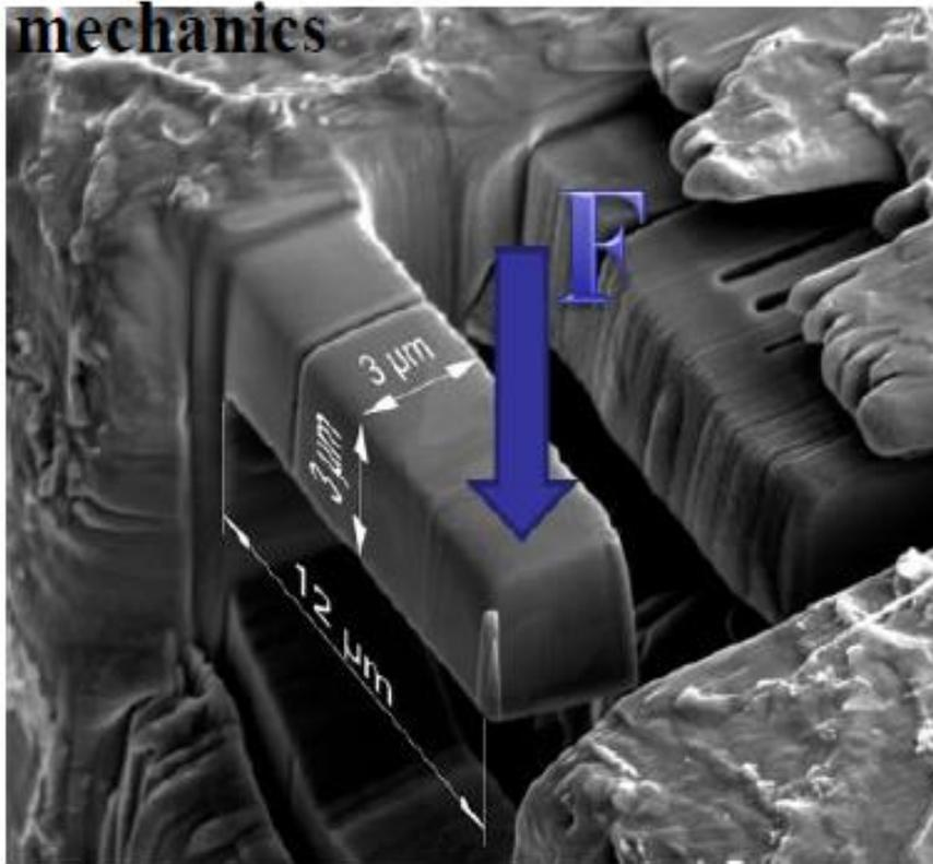
→ Fracture toughness ( $K_{Ic}$ )
