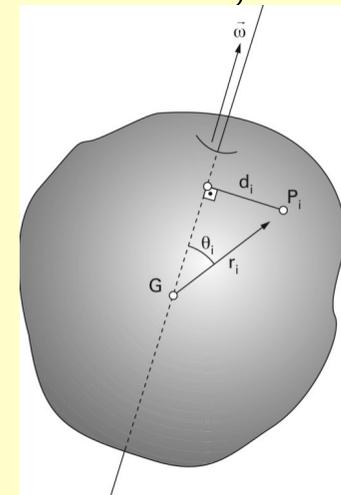
$$E = \frac{1}{2} m v_G^2 + \frac{1}{2} \omega^2 J_{G\omega} = \frac{1}{2} m \omega^2 d^2 + \frac{1}{2} \omega^2 J_{G\omega} = \frac{1}{2} \omega^2 (m d^2 + J_{G\omega}) = \frac{1}{2} \omega^2 J_{C\omega}$$
