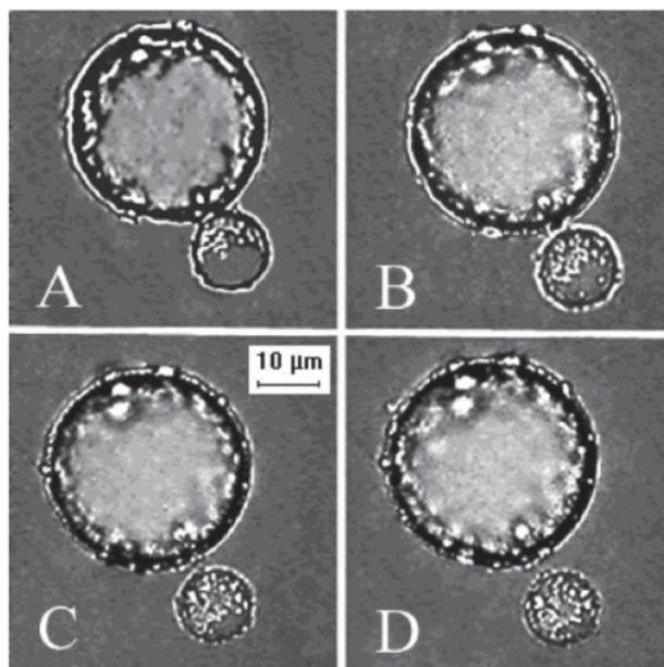
**Figure 2.** The redistribution of silica particles at the octanol droplet surface over time (in order from A to D). Brighter regions on the smaller droplet indicate trapped-particle locations. Reproduced with permission.<sup>[46]</sup> Copyright 2003, American Chemical Society.
