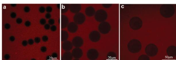
**Figure 6.** Confocal microscopy images of Pickering emulsions (o/w) prepared by DME using different membrane pore sizes. The pore sizes of the membrane were: a) 2.5, b) 5.2, and c) 9.2  $\mu\text{m}$ . The pH of the aqueous phase was 5.7, and PNIPAM-co-MAA microgels were labeled with rhodamine B molecules. Reproduced with permission.<sup>[74]</sup> Copyright 2014, American Chemical Society.
