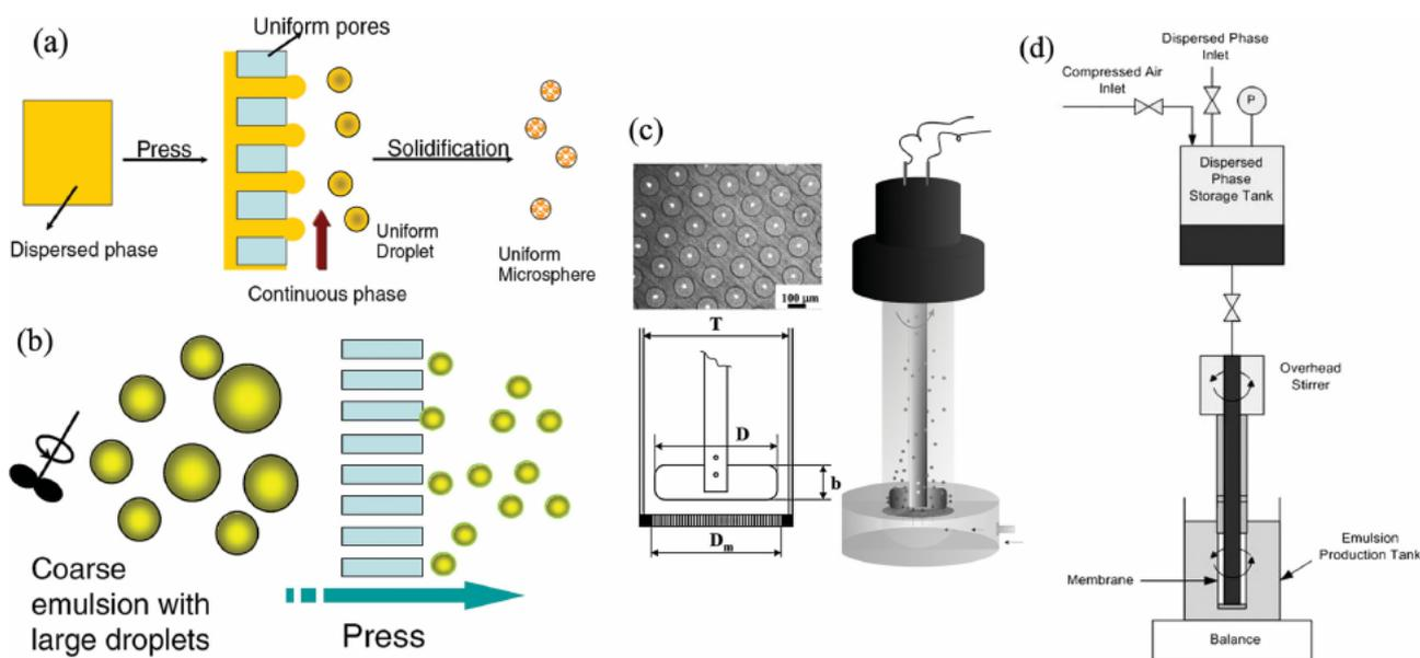
Figure 5. Schematic illustrations of DME (a), PME (b), SCME (c) and RME (d). a,b) Reproduced with permission.<sup>[66]</sup> Copyright 2014, Elsevier. c) Reproduced with permission.<sup>[67]</sup> Copyright 2012, Elsevier. Reproduced with permission.<sup>[68]</sup> Copyright 2014, Elsevier.
