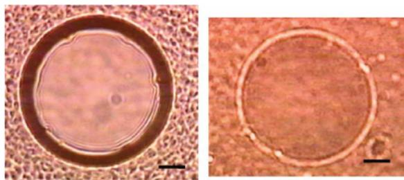
Figure 4. Light microscopy images of the cross-section of droplets prepared by (left) MC emulsification technique and (right) homogenization. Scale bar = 10  $\mu\text{m}$ . Reproduced with permission.<sup>[60]</sup> Copyright 2005, Elsevier.
