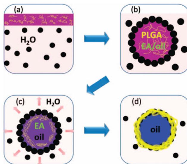
**Figure 8.** Schematic showing the principle of the polymer deposition method for preparation of capsules. Reproduced with permission.<sup>[96]</sup> Copyright 2009, American Chemical Society.
