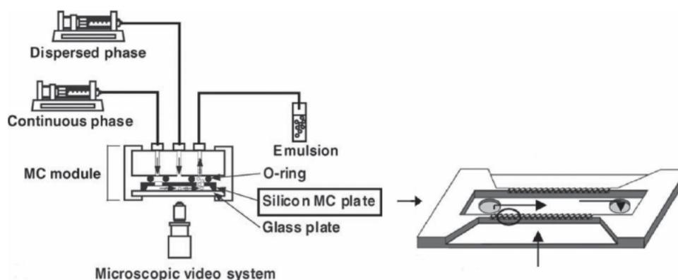
Figure 3. Experimental setup of microchannel (MC) emulsification. Reproduced with permission.<sup>[60]</sup> Copyright 2005, Elsevier.
