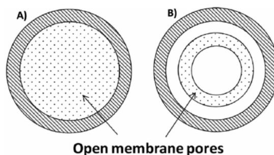
**Figure 7.** A) Standard membrane, B) annular radial ring membrane. Reproduced with permission.<sup>[71]</sup> Copyright 2011, American Chemical Society.
