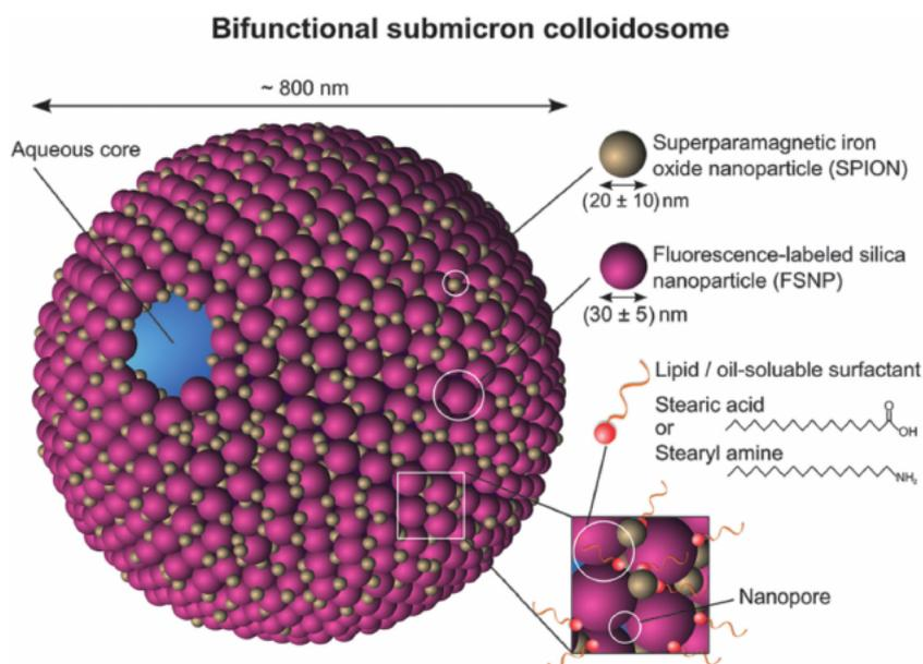
**Figure 12.** Schematic illustration of colloidosomes with fluorescence-labeled silica nanoparticles and superparamagnetic iron oxide nanoparticles on the shell. Reproduced with permission.<sup>[153]</sup> Copyright 2015, Wiley-VCH Verlag GmbH & Co. KGaA.
