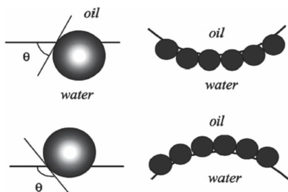
**Figure 1.** Contact angle (left) and corresponding probable positioning (right) of spherical particles at the oil-water interface. Reproduced with permission.<sup>[15]</sup> Copyright 2002, Elsevier.
