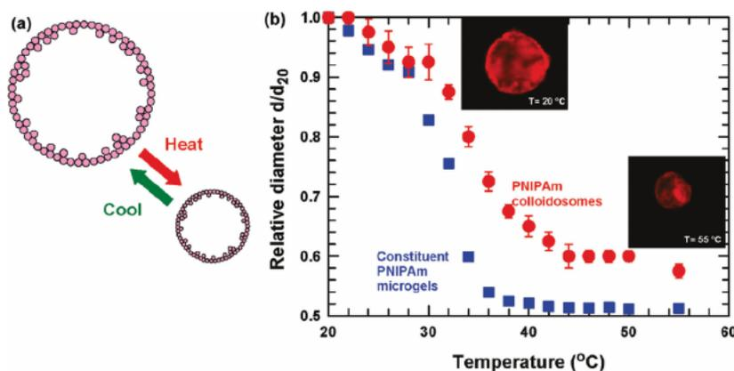
**Figure 11.** a) Schematic representation of the thermoresponsive behavior of a colloidosome-PNIPAm nanoparticle shell. b) Equilibrium size change of PNIPAm colloidosomes and their constituent PNIPAm microgels. Size data of three different colloidosomes were averaged for better statistics. Reproduced with permission.<sup>[64]</sup> Copyright 2010, American Chemical Society.
