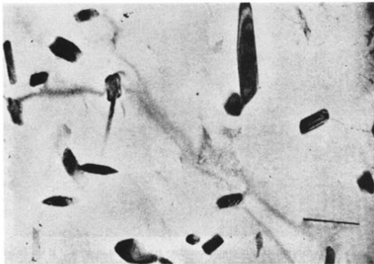
Fig. 3.44 Electron micrograph showing incoherent particles of  $\theta$  in an Al–Cu alloy.
