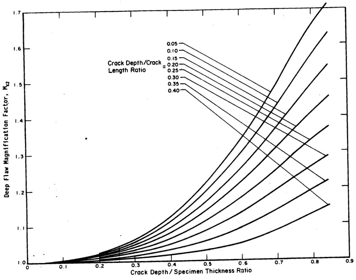
Figure 2-44. Deep flaw magnification factor curves.
