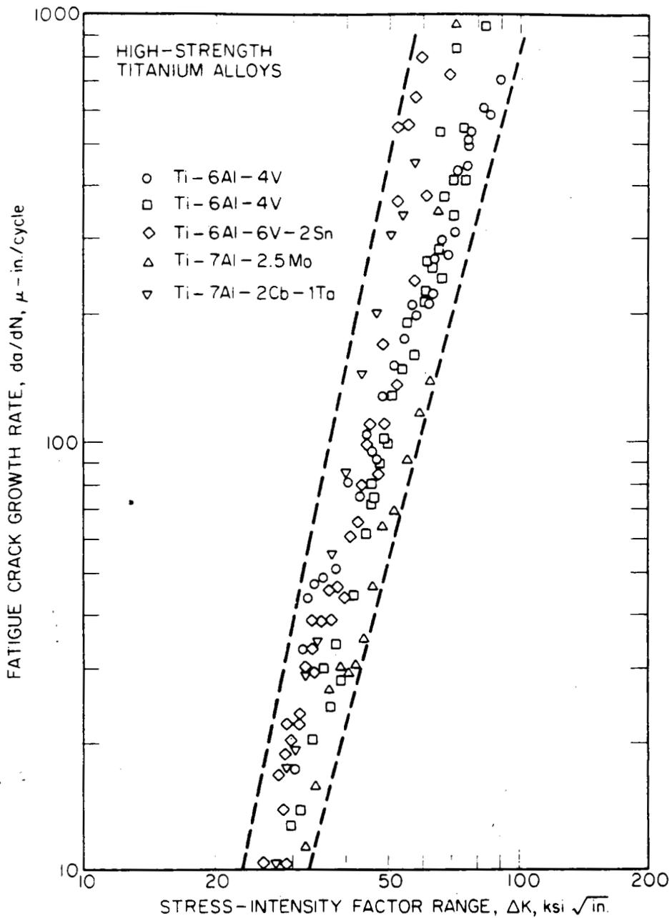
Figure 3-8. Summary plot of  $da/dN$  versus  $\Delta K$  for five titanium alloys.
