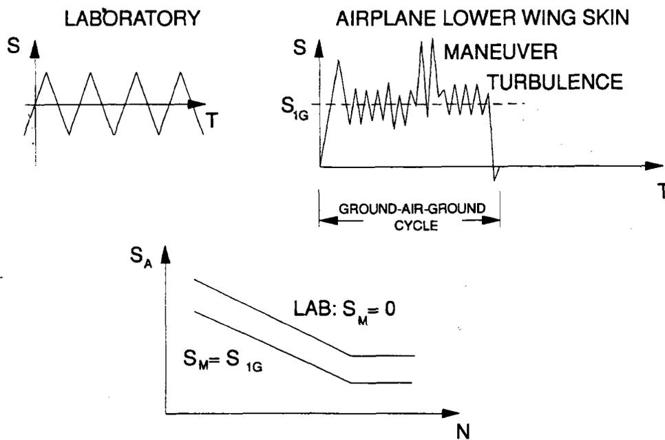
Figure 1-10. Effect of mean stress.
