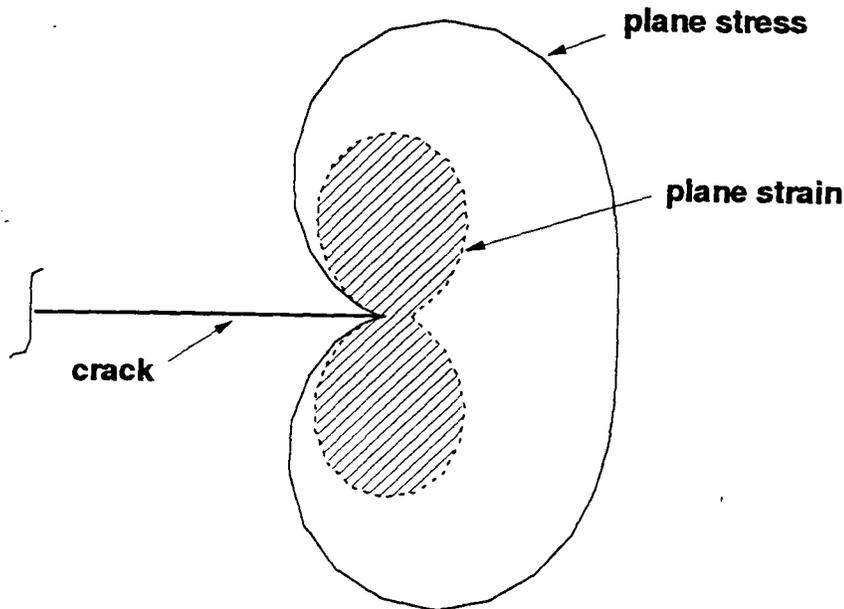
Figure 2-11. Plastic zone approximations based on von Mises criterion
