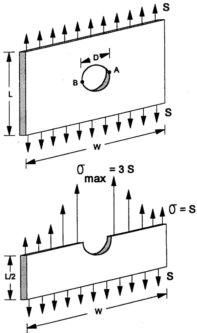
Figure 2-1. Circular hole in a large plate.
