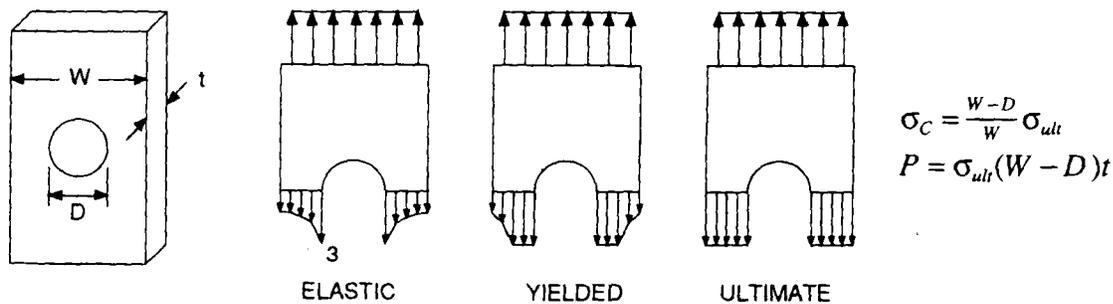
Figure 2-34. Net section failure criterion.
