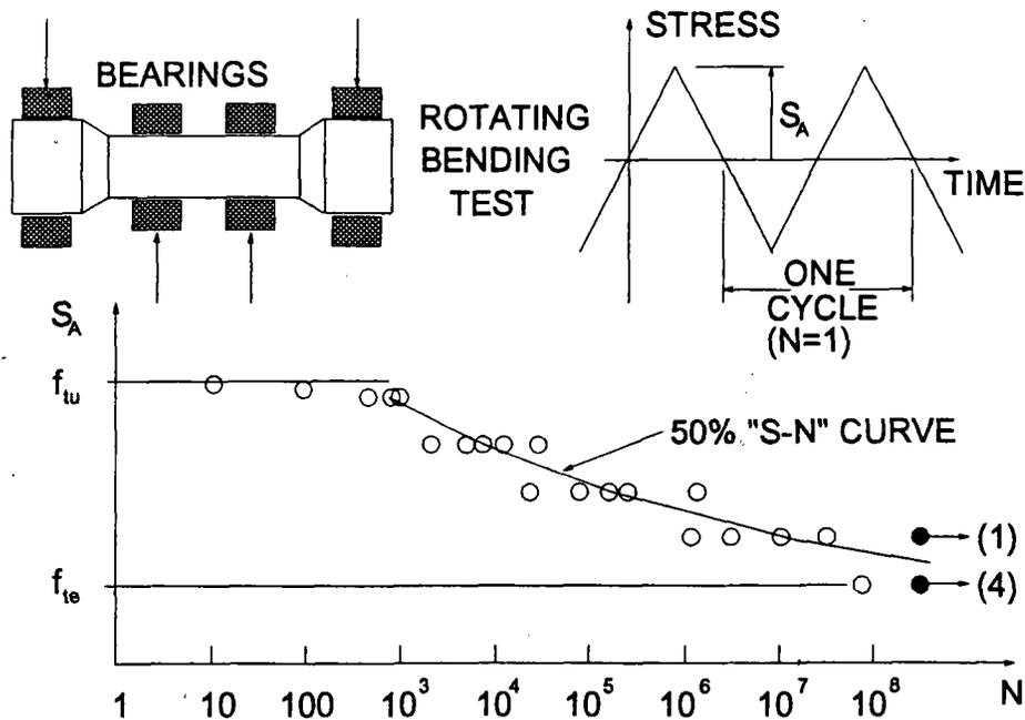
Figure 1-9. Results of a typical fatigue experiment.
