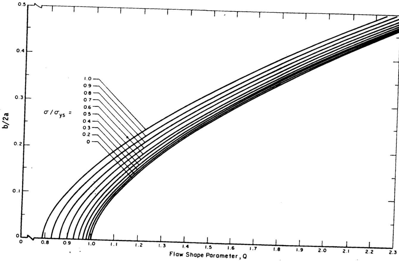
Figure 2-43. Stress intensity factors for surface and corner cracks.
