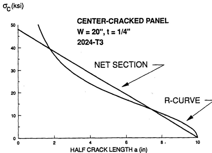
Figure 2-35. Net section and R-curve strength curves.
