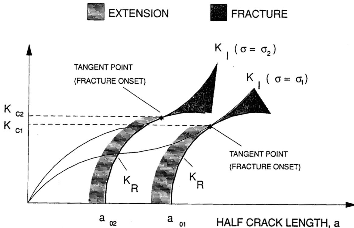
Figure 2-24. Dependence of  $K_c$  on crack length.
