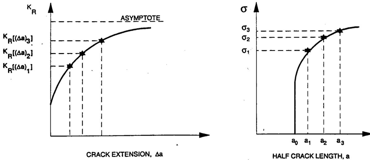
Figure 2-23. Experimental determination of R-curve.
