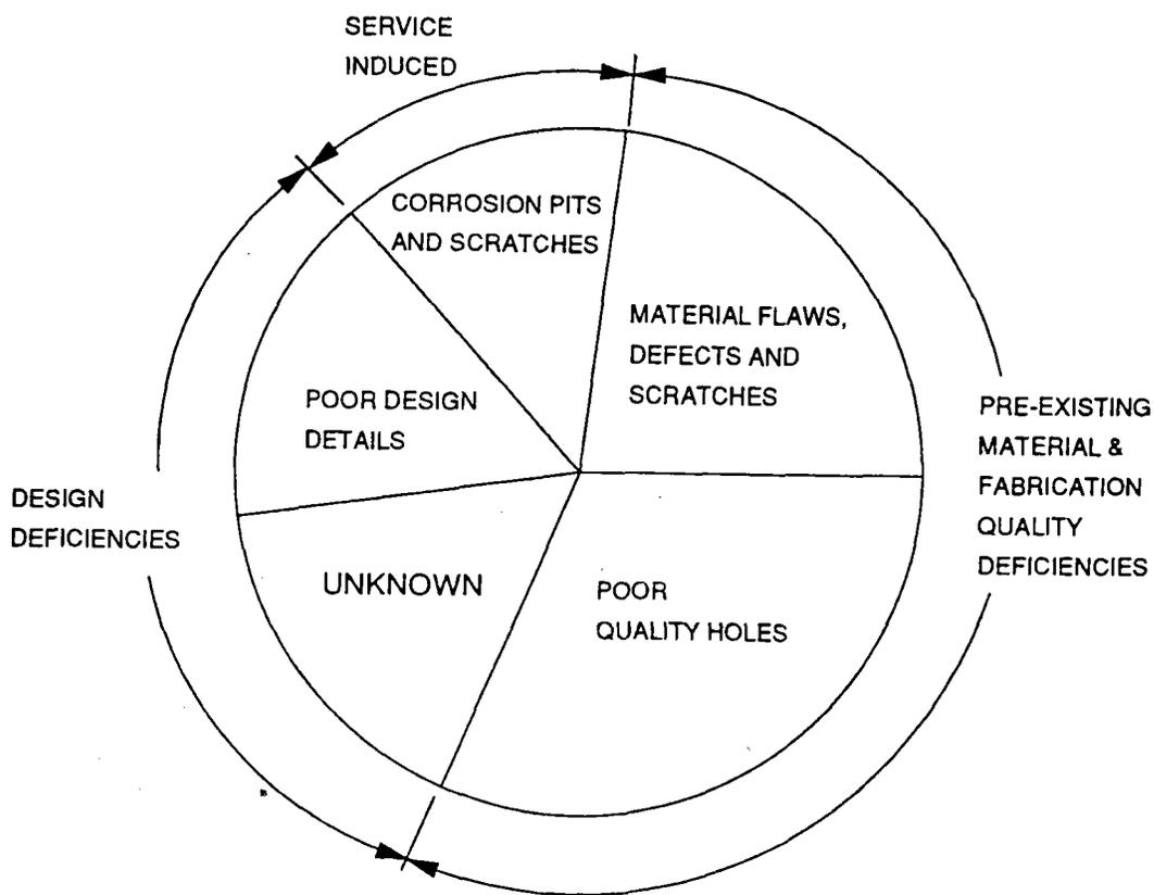
Figure 1-8. Cracking and failure origins.
