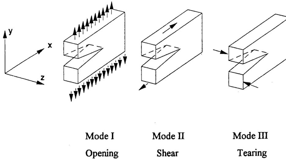
Figure 2-8. Fracture modes
