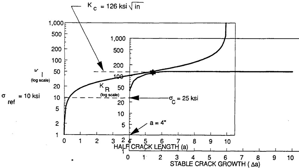
Figure 2-31. Critical stress determinations with  $K_I$  and  $K_R$  curves.
