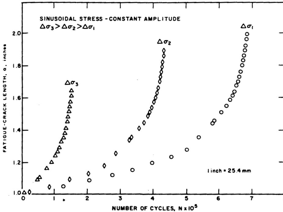
Figure 3-2. Effect of cyclic load range on crack growth in Ni-Mo-V alloy steel for released tension loading.
