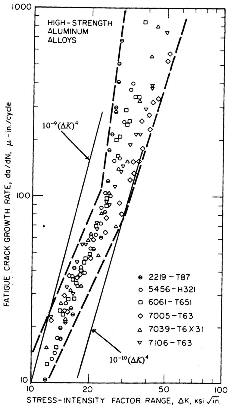
Figure 3-6. Summary plot of  $da/dN$  versus  $\Delta K$  for six aluminum alloys.
