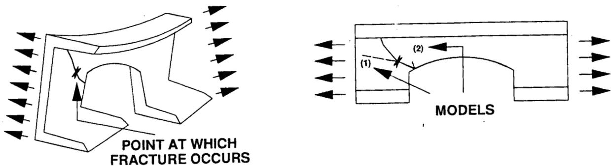
(c) Through-crack at a fuselage frame corner detail.
