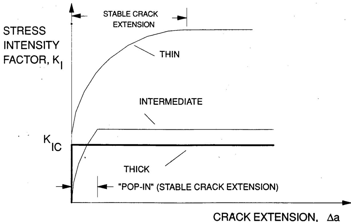
Figure 2-22. Load versus crack extension for different thicknesses.
