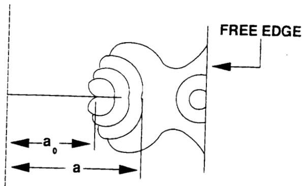
(c) One crack tip near edge of a panel.
