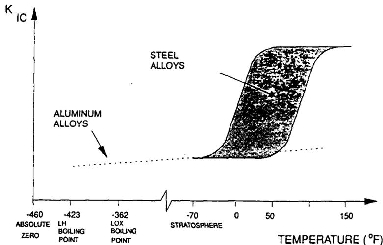
Figure 2-21. Fracture toughness versus temperature.
