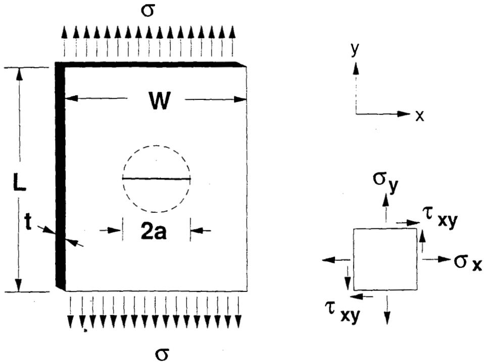
Figure 2-5. Plate with a center crack.
