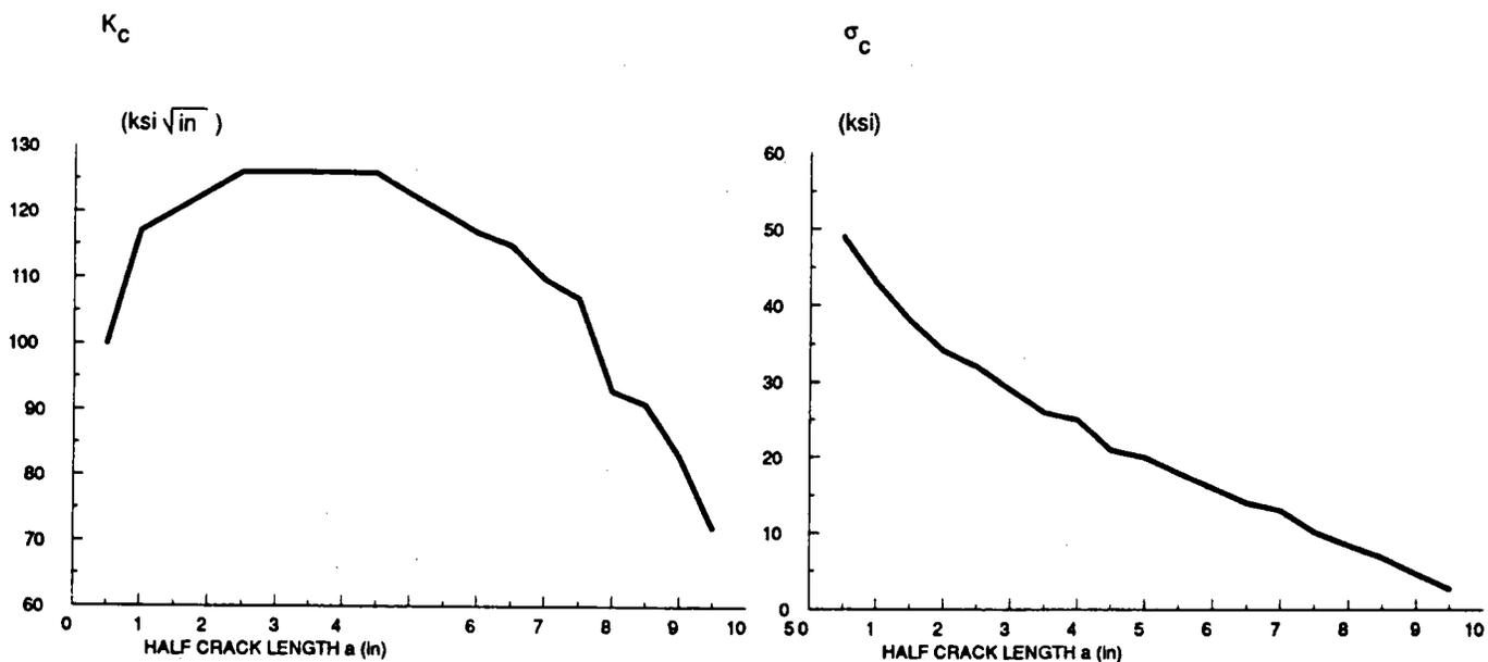
Figure 2-32.  $K_c$  and  $\sigma_c$  vs.  $a$  for a 20-inch aluminum panel.
