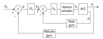
Figure 4.6-12 A roll angle control system.
