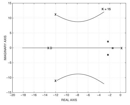
Figure 4.6-13 Root-locus plot for roll-angle-hold controller.
