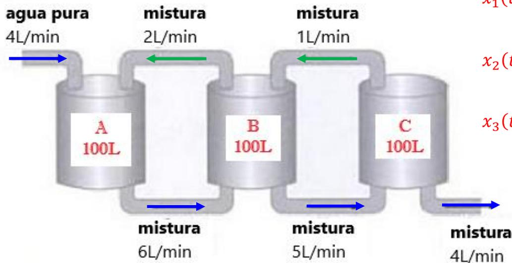
$$x_1(t) = \frac{48}{100}c_1e^{-\frac{1}{10}t} + \frac{18}{100}c_2e^{-\frac{5}{100}t} + \frac{29}{100}c_3e^{-\frac{2}{100}t};$$
