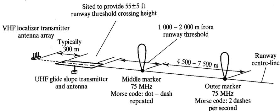
Figure 11.36 Location of ILS ground transmitters and antennas.
