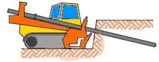
STEP 2. DRILL NAIL HOLE
