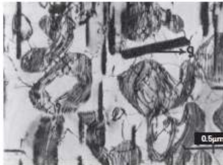
Fig. 10.16 Interfacial dislocations formed in a semicoherent precipitate. (From G. C. Weatherly and R. B. Nicholson, Phil. Mag. , 17 (1968), 901.)
