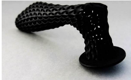
Figure 16: Example of a part produced with MJF technology (image courtesy of Sculpteo)
