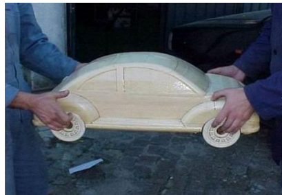
Figure 34: Example of a part produced with LOM technology (image courtesy of INEGI, Institute of Science and Innovation in Mechanical and Industrial Engineering)
