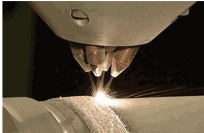
Figure 20: Part being manufactured using LENS AM technology (image courtesy of OPTOMECC)
