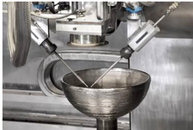
Figure 22: Example of a part produced with EBAM technology (image courtesy of Sciaky, Inc.)
