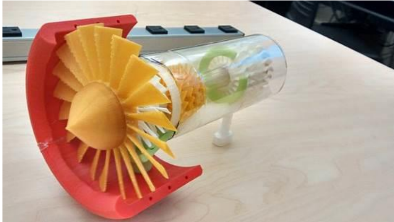
Figure 18: Example of a part produced with FDM technology (Image by C Michelle under Creative Commons CCBY-SA 4.0. licence, via Wikimedia Commons)
