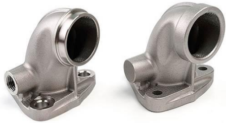
Figure 10: Speedboat engine exhaust flanges manufactured by DMLS (Direct Metal Laser Sintering). The flange on the left is CNC machined using Ti-6Al4V - Courtesy of CRP Technology SRL.
