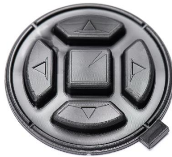
Figure 28: Example of a part produced with CDLP technology (image courtesy of Carbon3D)
