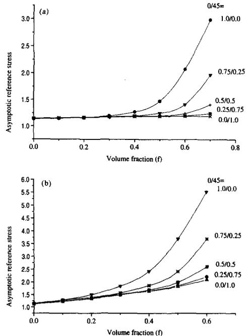
Fig. 11. Mixture of 0 and  $45^\circ$  loading, asymptotic reference stress,  $\bar{\sigma}_N$ , for (a) hardening exponent  $N = 0.0$ ; (b) hardening exponent  $N = 0.5$ .
