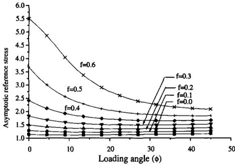
Fig. 12. Asymptotic reference stress,  $\bar{\sigma}_N$ , for various loading angles and varying volume fraction, hardening exponent  $N = 0.0$ .
