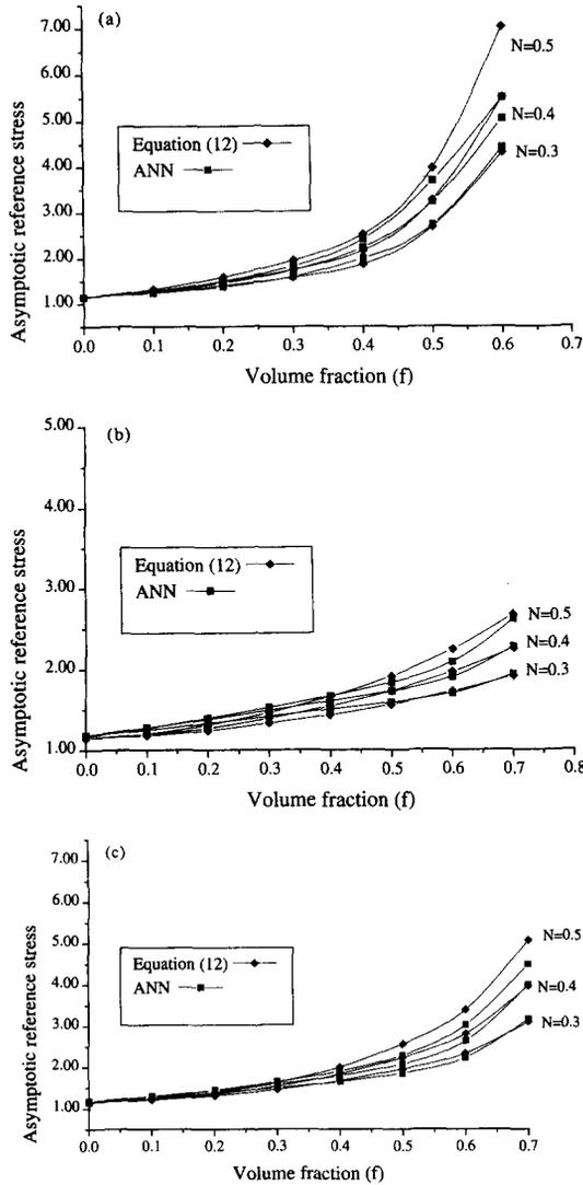
Fig. 10. New hardening exponents, asymptotic reference stress,  $\bar{\sigma}_N$ , for (a) square arrangement for loading at  $0^\circ$ ; (b) square arrangement for loading at  $45^\circ$ ; (c) hexagonal arrangement.
