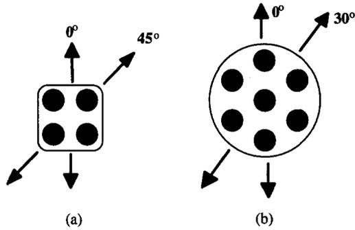
Fig. 4. Arrangements of fiber with primary loading directions: (a) rectangular arrangement; (b) hexagonal arrangement.
