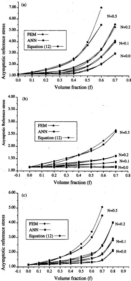
Fig. 7. Asymptotic reference stress,  $\bar{\sigma}_N$ , for (a) square arrangement for loading at  $0^\circ$ ; (b) square arrangement for loading at  $45^\circ$ ; (c) hexagonal arrangement.
