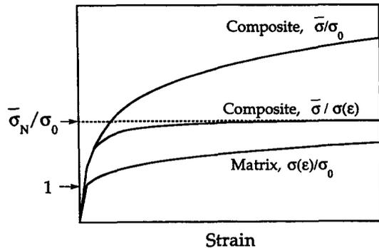
Fig. 5. Asymptotic reference stress  $\bar{\sigma}_N$ , for work hardening matrices.
