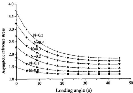
Fig. 13. Asymptotic reference stress,  $\bar{\sigma}_N$ , for various loading angles and varying hardening exponent, volume fraction  $f = 0.5$ .
