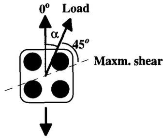
Fig. 14. Critical angle for strengthening for arbitrary loading direction.
