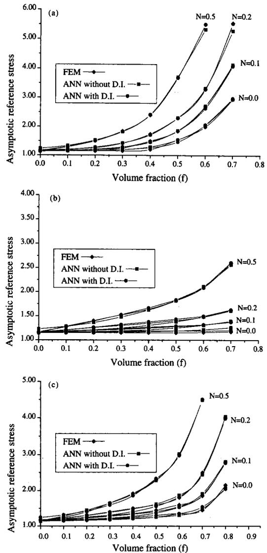
Fig. 9. Performance of derived input, asymptotic reference stress,  $\bar{\sigma}_N$ , for (a) square arrangement for loading at  $0^\circ$ ; (b) square arrangement for loading at  $45^\circ$ ; (c) hexagonal arrangement.
