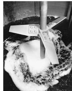
FIG. 18-2 An A310 impeller.
