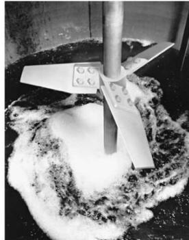
FIG. 18-2 An A310 impeller.
