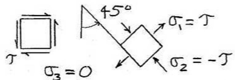
$$\begin{aligned}\bar{\sigma}_{\text{ef}} &= \max(|\sigma_1 - \sigma_2|, |\sigma_2 - \sigma_3|, |\sigma_3 - \sigma_1|) \\ &= \max(|\tau - (-\tau)|, |\tau - 0|, |0 - \tau|) \\ &= \max(2|\tau|, \tau, |\tau|)\end{aligned}$$
