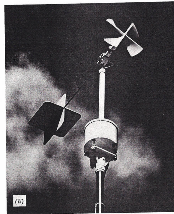
Fig. 4.13 (h) The Gill anemometer bivane measures wind speed plus simultaneous azimuth and elevation angles of the wind (courtesy of R. M. Young Co., Ann Arbor, Michigan).
