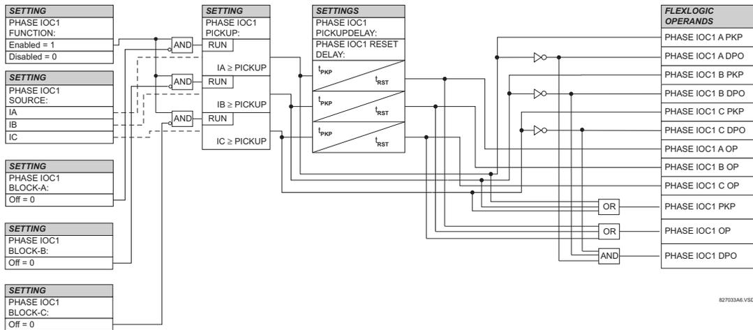
Figure 5-60: PHASE INSTANTANEOUS OVERCURRENT 1 SCHEME LOGIC
