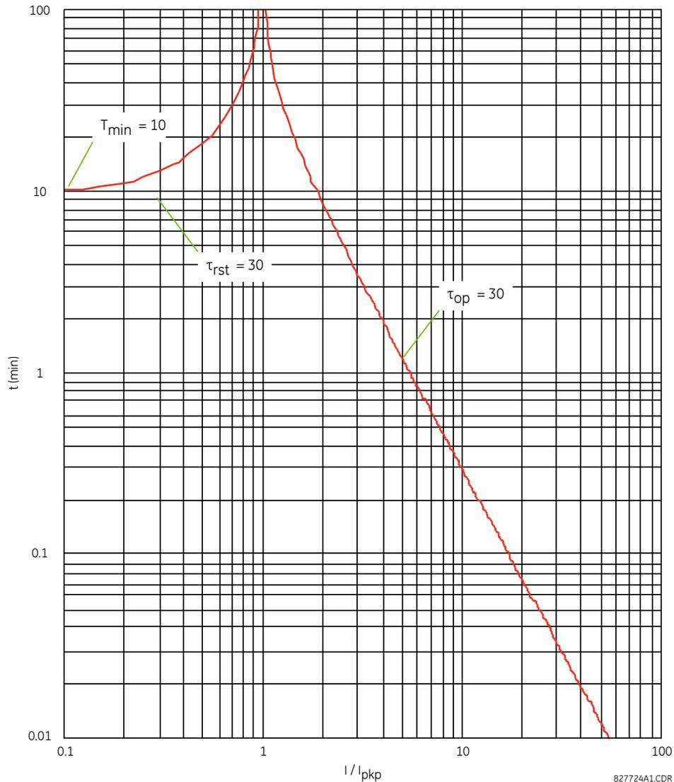
**Figure 5-119: IEC 255-8 SAMPLE OPERATE AND RESET CURVES**
