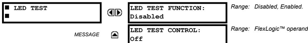
When enabled, the LED test can be initiated from any digital input or user-programmable condition such as user-programmable pushbutton. The control operand is configured under the **LED TEST CONTROL** setting. The test covers all LEDs, including the LEDs of the optional user-programmable pushbuttons.
