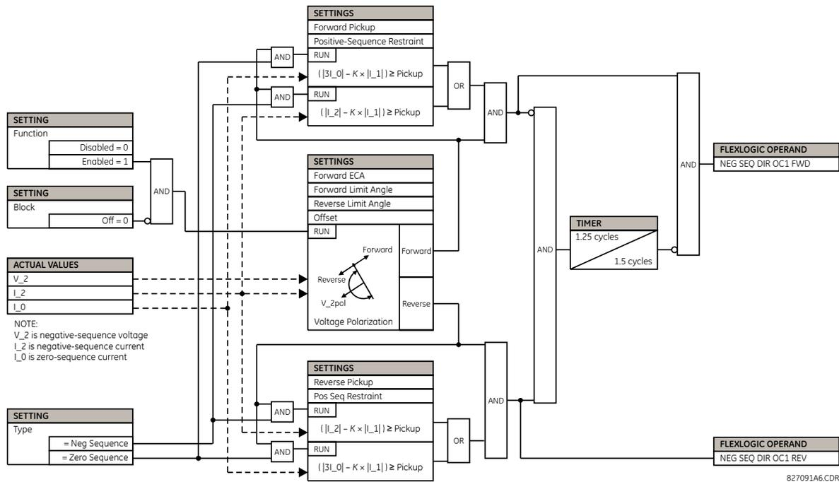
Figure 5-74: NEGATIVE SEQUENCE DIRECTIONAL OC1 SCHEME LOGIC
