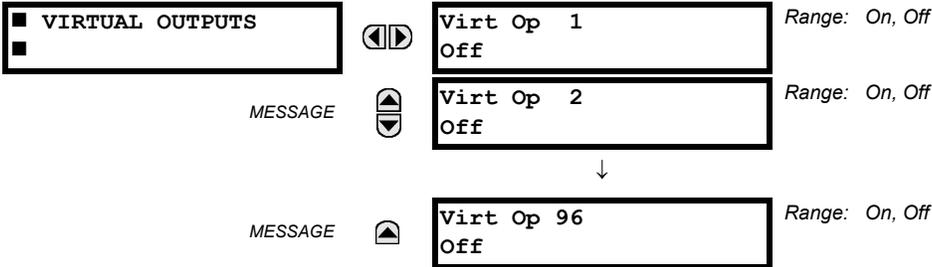
The present state of up to 96 virtual outputs is shown here. The first line of a message display indicates the ID of the virtual output. For example, 'Virt Op 1' refers to the virtual output in terms of the default name-array index. The second line of the display indicates the logic state of the virtual output, as calculated by the FlexLogic™ equation for that output.
