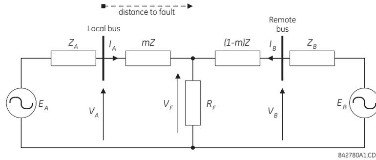
Figure 9-1: EQUIVALENT SYSTEM FOR FAULT LOCATION
