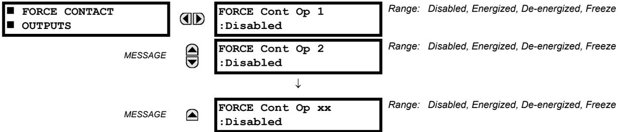
The relay contact outputs can be pre-programmed to respond to the test mode.
