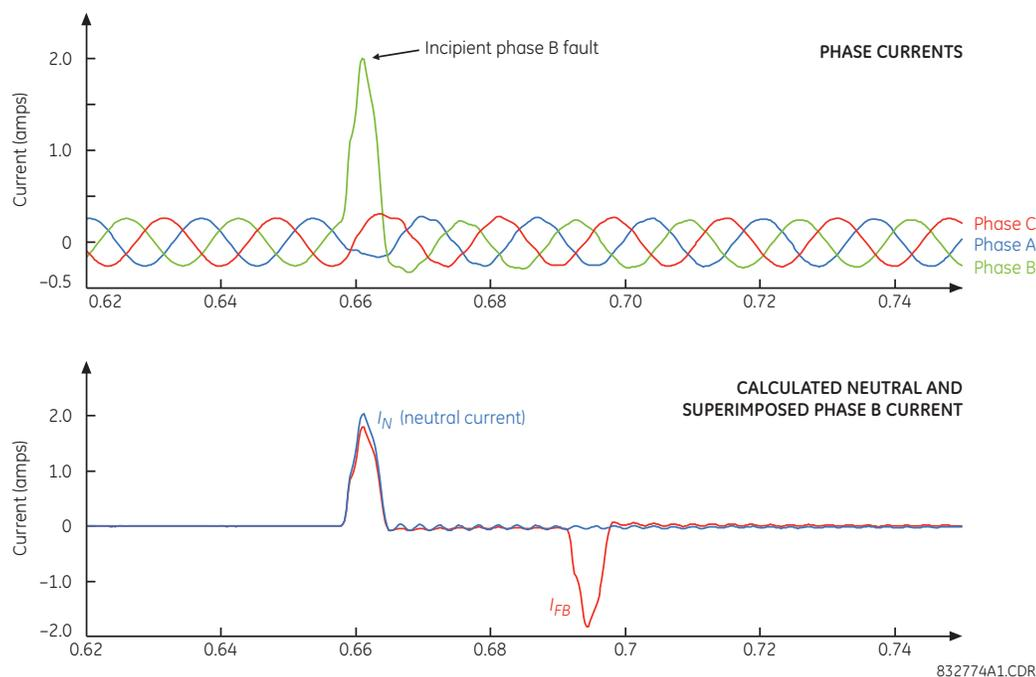
**Figure 5-115: ILLUSTRATION OF THE INCIPIENT FAULT DETECTOR ALGORITHM**
