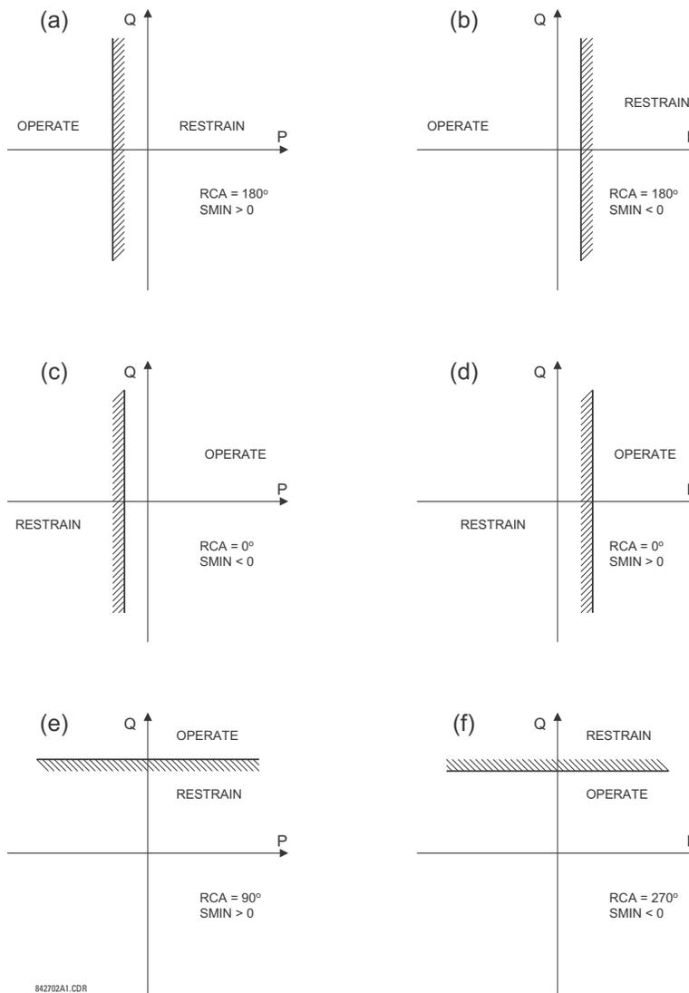
Figure 5-89: DIRECTIONAL POWER ELEMENT SAMPLE APPLICATIONS
