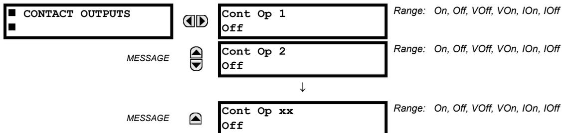
The present state of the contact outputs is shown here. The first line of a message display indicates the ID of the contact output. For example, 'Cont Op 1' refers to the contact output in terms of the default name-array index. The second line of the display indicates the logic state of the contact output.
