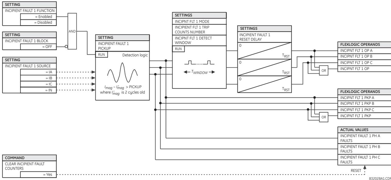
Figure 5-116: INCIPIENT CABLE FAULT DETECTOR SCHEME LOGIC
