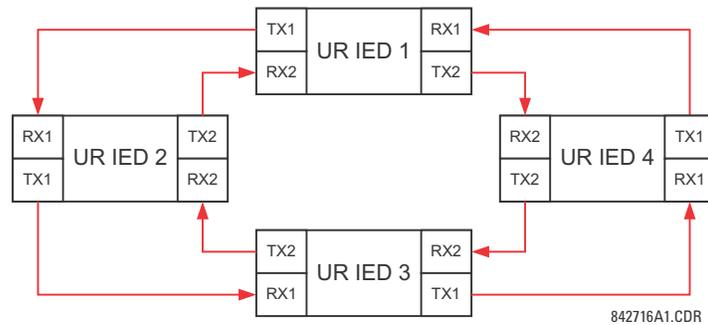
**Figure 5–14: INTERLOCKING BUS PROTECTION SCHEME VIA DIRECT INPUTS/OUTPUTS**
