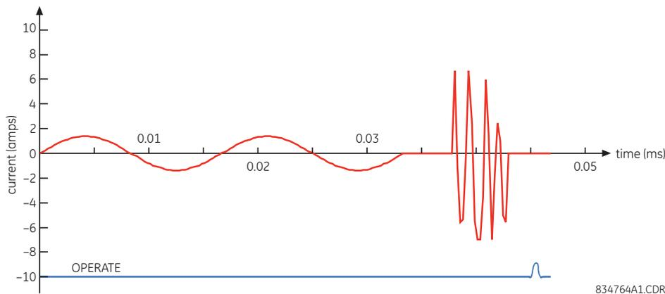
Figure 5-112: TYPICAL RESTRIKE WAVEFORM AND DETECTION FLAG
