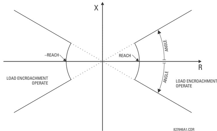
Figure 5-54: LOAD ENCROACHMENT CHARACTERISTIC
