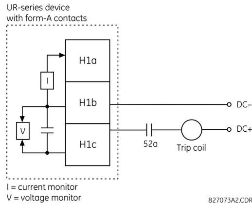
Figure 5–105: TRIP CIRCUIT EXAMPLE 1
