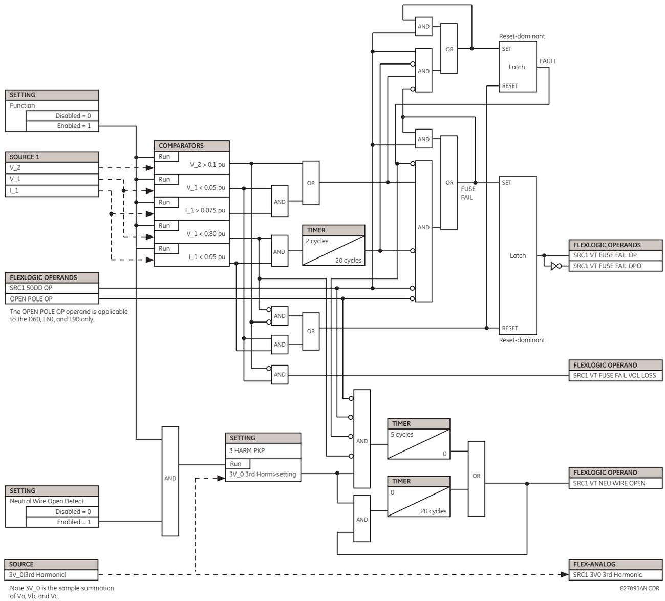
Figure 5-117: VT FUSE FAIL SCHEME LOGIC
