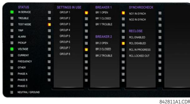
Figure 4-18: TYPICAL LED INDICATOR PANEL FOR ENHANCED FACEPLATE
