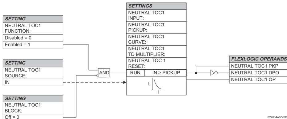
Figure 5-63: NEUTRAL TIME OVERCURRENT 1 SCHEME LOGIC
