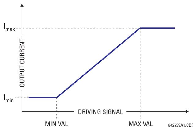
Figure 5–131: DCMA OUTPUT CHARACTERISTIC
