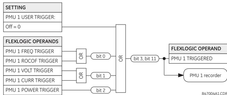
**Figure 5-36: STAT BITS LOGIC**
