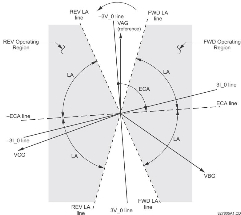
Figure 5-65: NEUTRAL DIRECTIONAL VOLTAGE-POLARIZED CHARACTERISTICS
