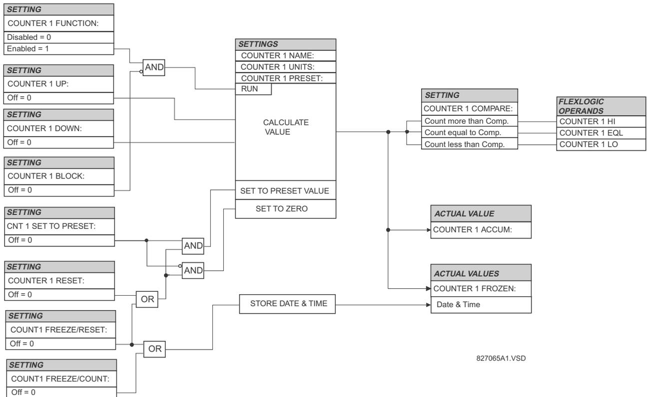
Figure 5-107: DIGITAL COUNTER SCHEME LOGIC
