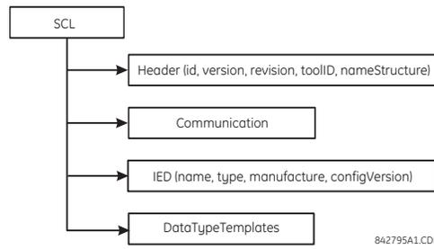
Figure 0-2: ICD FILE STRUCTURE, SCL (ROOT) NODE
