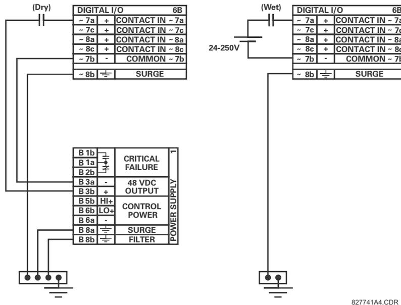
**Figure 3-21: DRY AND WET CONTACT INPUT CONNECTIONS**
