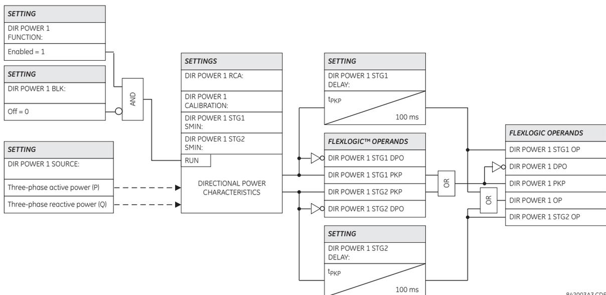
Figure 5-90: SENSITIVE DIRECTIONAL POWER SCHEME LOGIC
