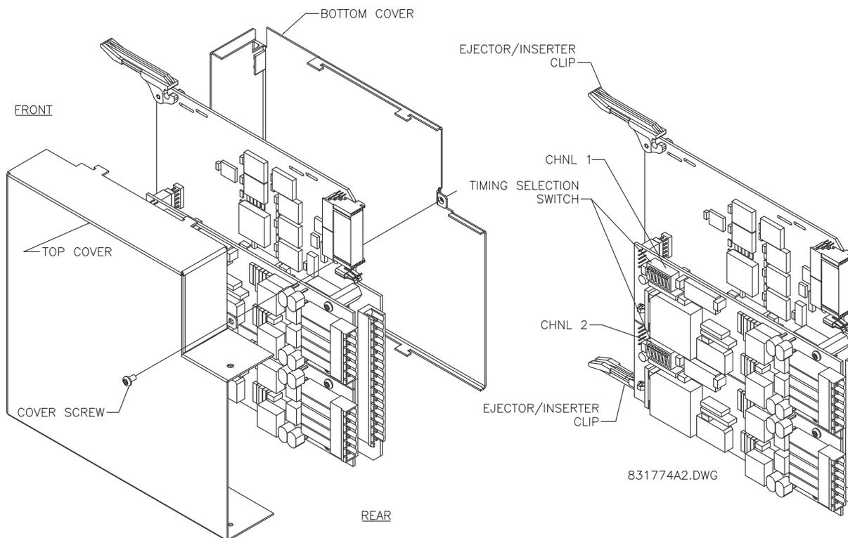
Figure 3-46: IEEE C37.94 TIMING SELECTION SWITCH SETTING
