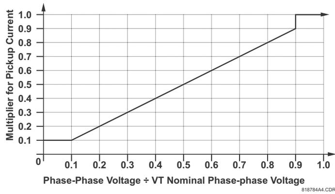
Figure 5-57: PHASE TIME OVERCURRENT VOLTAGE RESTRAINT CHARACTERISTIC
