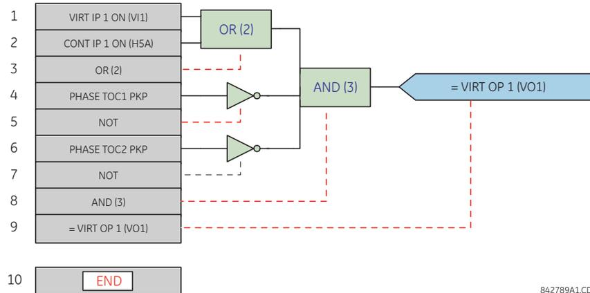
Figure 5-93: EXAMPLE FLEXLOGIC™ CONTROL OF A SETTINGS GROUP
