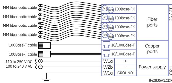
Figure 3–49: MANAGED ETHERNET SWITCH MODULE WIRING
