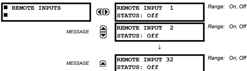
The present state of the 32 remote inputs is shown here.
