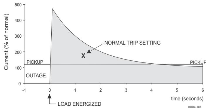
Figure 5-121: TYPICAL COLD LOAD PICKUP CHARACTERISTIC
