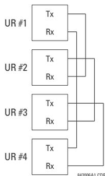
Figure 3–30: DIRECT INPUT AND OUTPUT SINGLE CHANNEL CONNECTION
