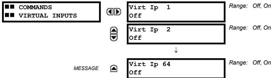
The states of up to 64 virtual inputs are changed here. The first line of the display indicates the ID of the virtual input. The second line indicates the current or selected status of the virtual input. This status will be a state off (logic 0) or on (logic 1).
