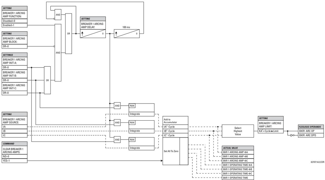
Figure 5-110: BREAKER ARCING CURRENT SCHEME LOGIC
