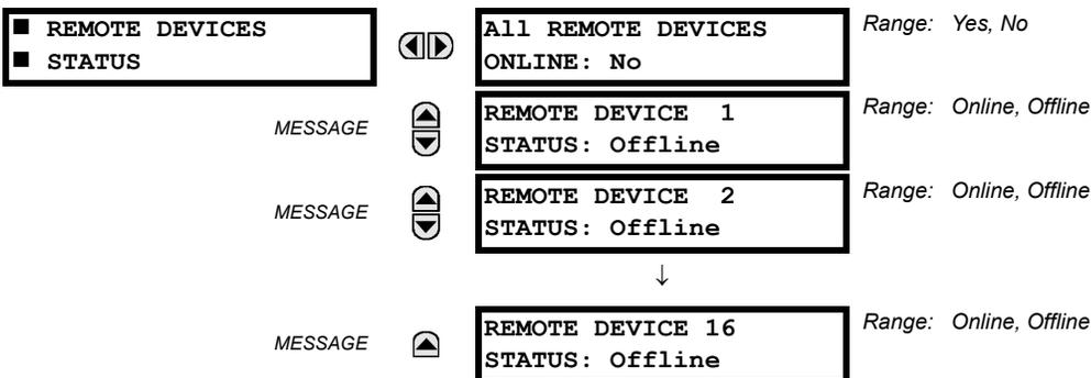
The present state of the programmed remote devices is shown here. The **ALL REMOTE DEVICES ONLINE** message indicates whether or not all programmed remote devices are online. If the corresponding state is "No", then at least one required remote device is not online.
