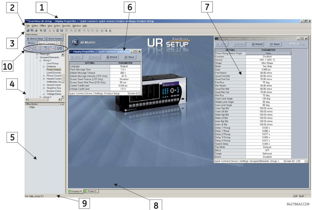
Figure 4-1: ENERVISTA UR SETUP SOFTWARE MAIN WINDOW
