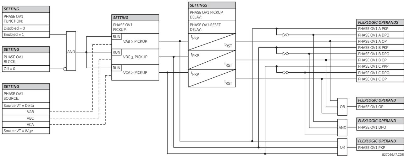
Figure 5-83: PHASE OVERVOLTAGE SCHEME LOGIC
