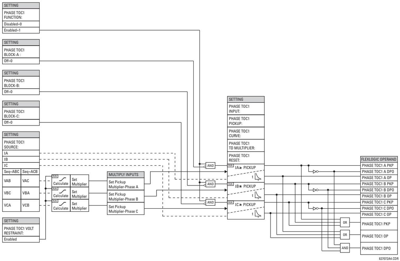
Figure 5-58: PHASE TIME OVERCURRENT 1 SCHEME LOGIC
