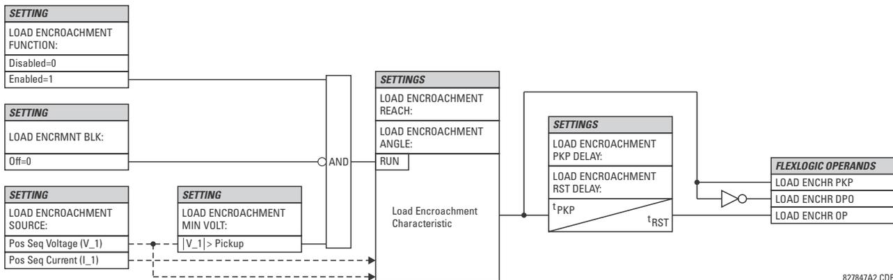
Figure 5-56: LOAD ENCROACHMENT SCHEME LOGIC
