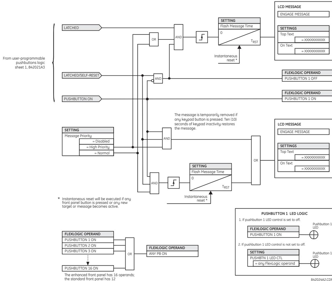
Figure 5-11: USER-PROGRAMMABLE PUSHBUTTON LOGIC (Sheet 2 of 2)
