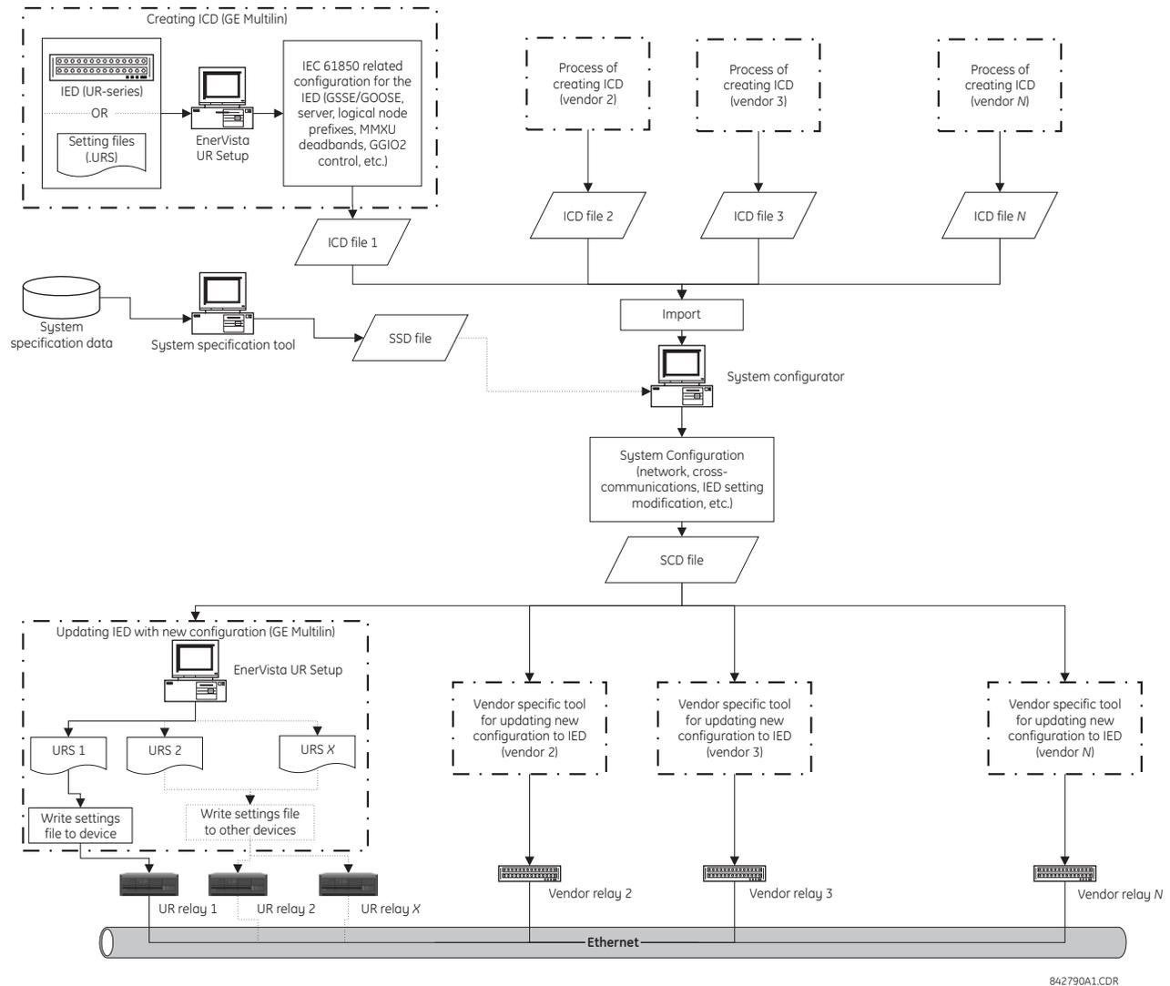
**Figure 0-1: IED CONFIGURATION PROCESS**
