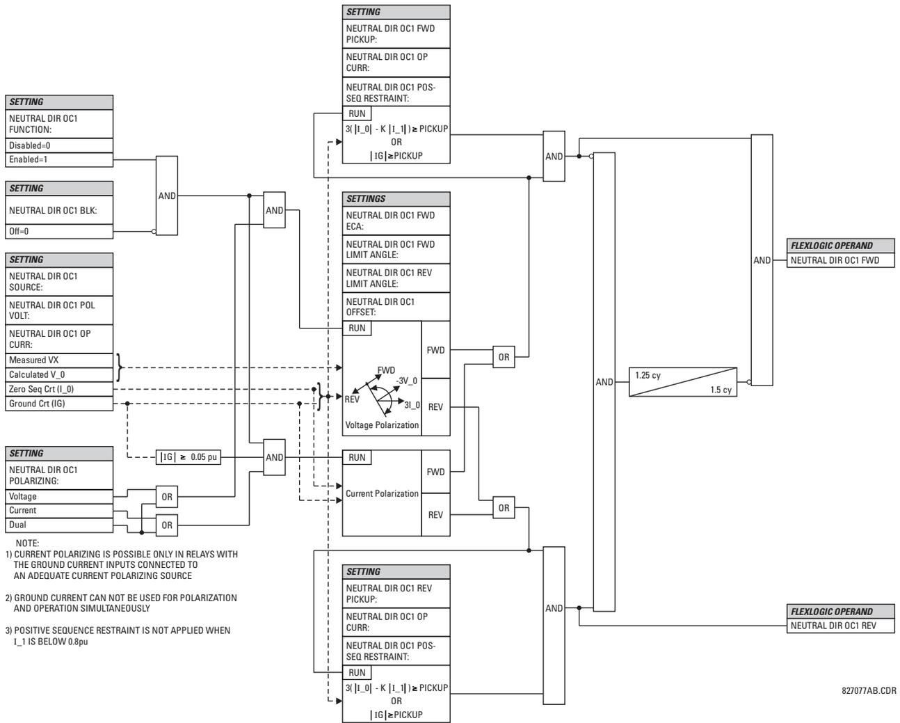
Figure 5–66: NEUTRAL DIRECTIONAL OVERCURRENT LOGIC
