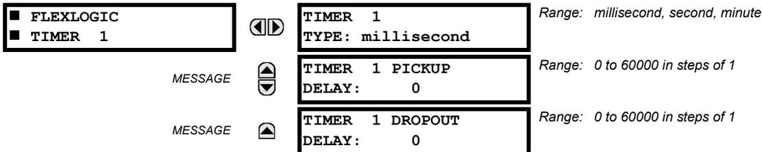
There are 32 identical FlexLogic™ timers available. These timers can be used as operators for FlexLogic™ equations.
