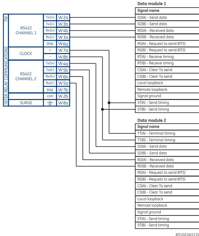
Figure 3–42: TIMING CONFIGURATION FOR RS422 TWO-CHANNEL, 3-TERMINAL APPLICATION
