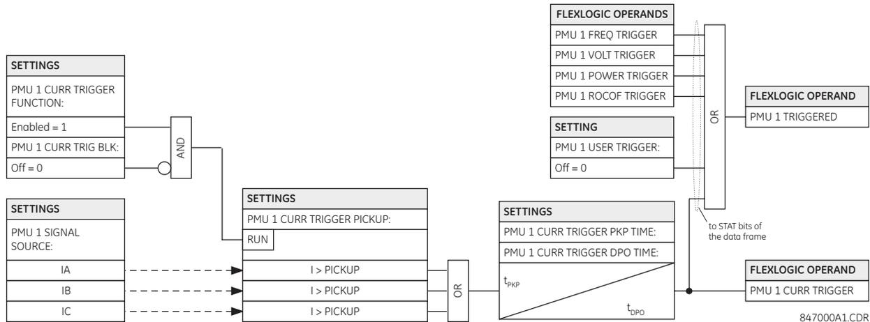
Figure 5-39: CURRENT TRIGGER SCHEME LOGIC
