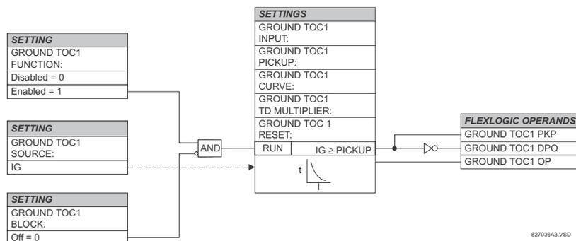
Figure 5–69: GROUND TOC1 SCHEME LOGIC
