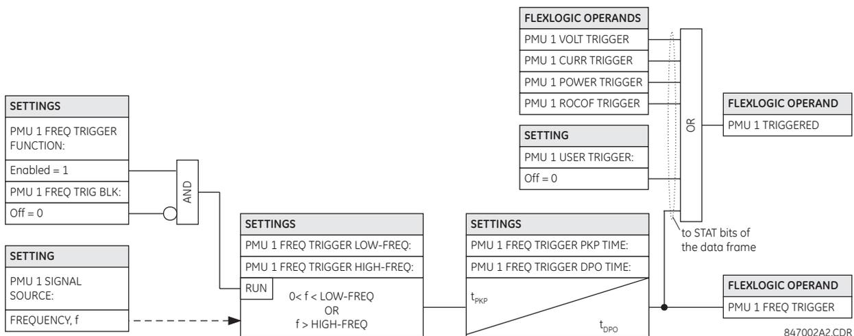
Figure 5-37: FREQUENCY TRIGGER SCHEME LOGIC
