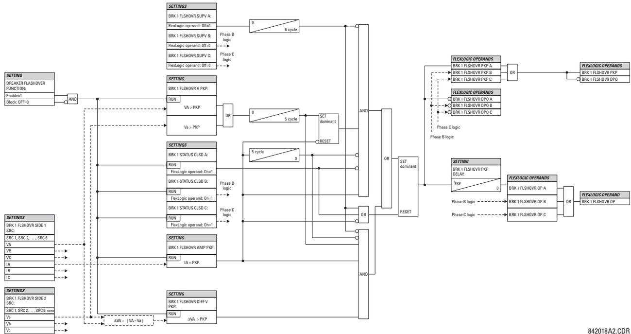
Figure 5-111: BREAKER FLASHOVER SCHEME LOGIC
