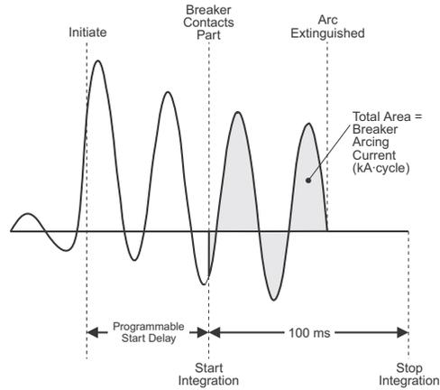
Figure 5-109: ARCING CURRENT MEASUREMENT
