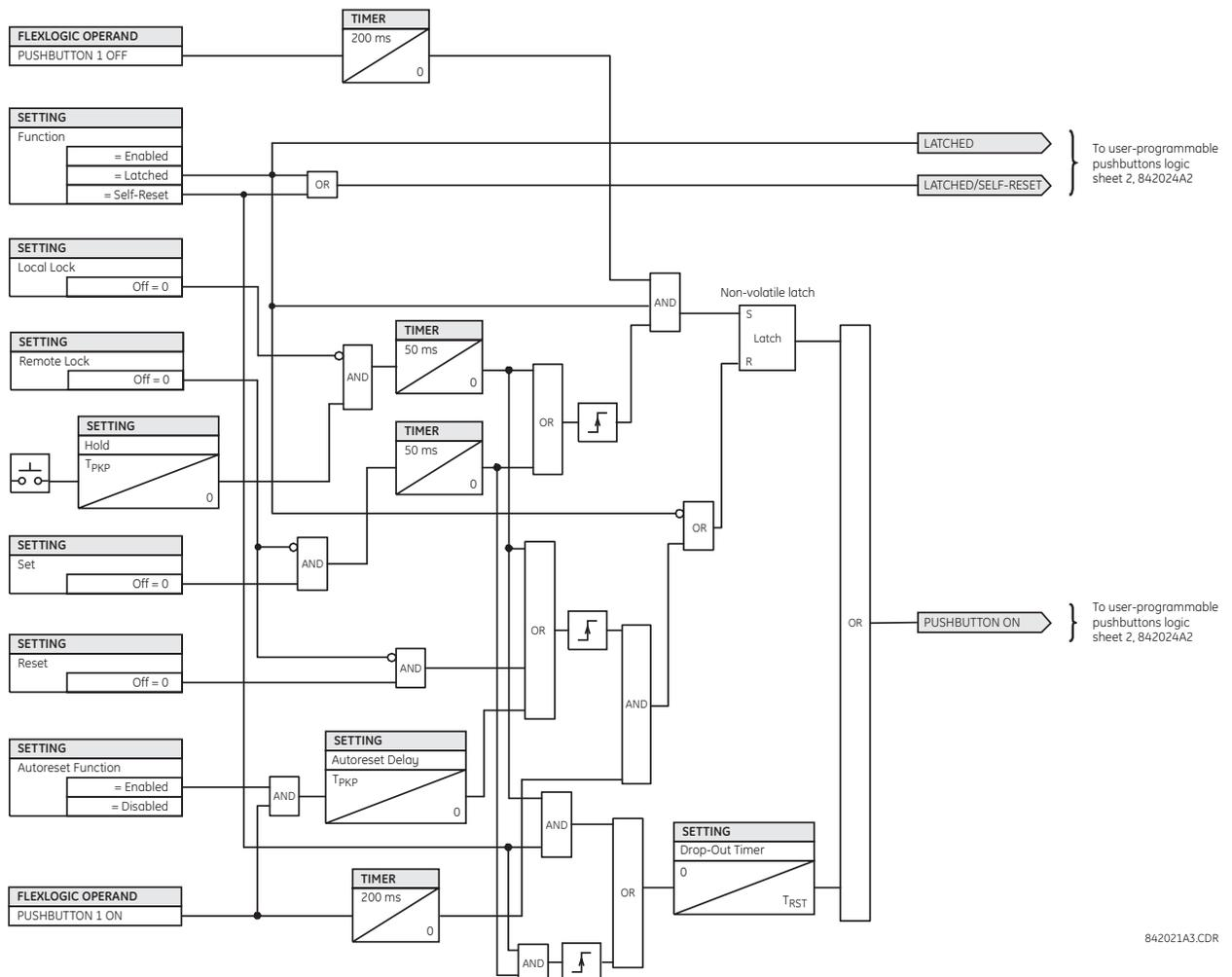
Figure 5-10: USER-PROGRAMMABLE PUSHBUTTON LOGIC (Sheet 1 of 2)
