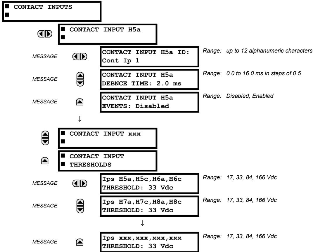
The contact inputs menu contains configuration settings for each contact input as well as voltage thresholds for each group of four contact inputs. Upon startup, the relay processor determines (from an assessment of the installed modules) which contact inputs are available and then display settings for only those inputs.
