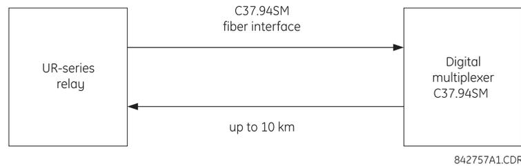
It can also be connected **directly** to any other UR-series relay with a C37.94SM module as shown below.
