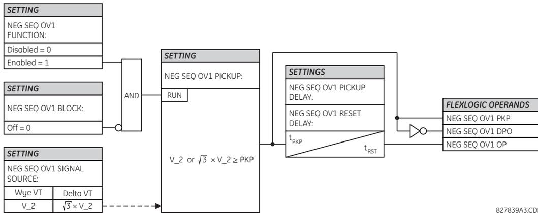
Figure 5-85: NEGATIVE-SEQUENCE OVERVOLTAGE SCHEME LOGIC
