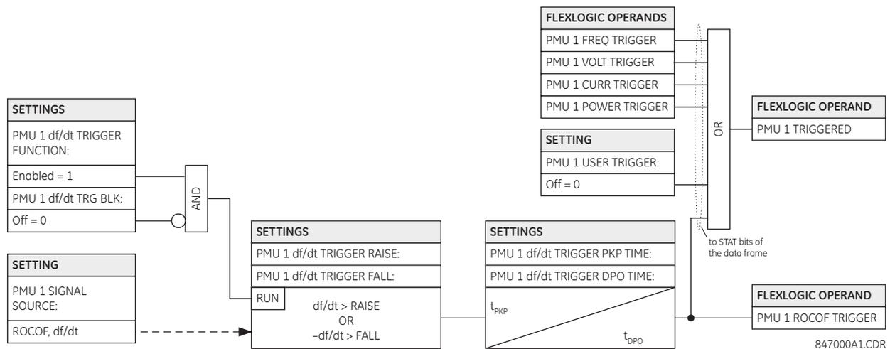
Figure 5-41: RATE OF CHANGE OF FREQUENCY TRIGGER SCHEME LOGIC
