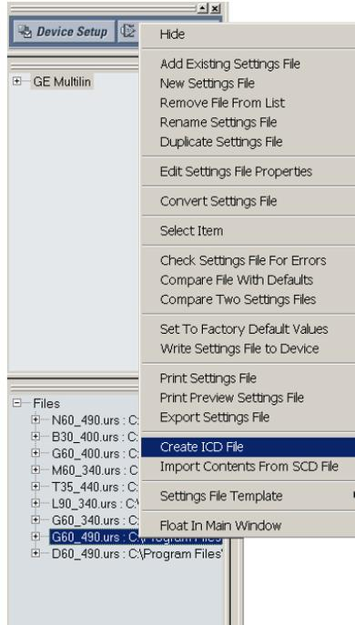
2. The EnerVista UR Setup will prompt to save the file. Select the file path and enter the name for the ICD file, then click **OK** to generate the file.
