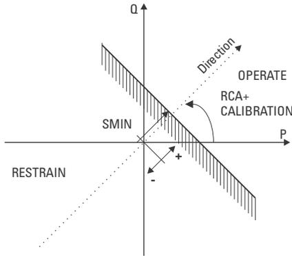
Figure 5-88: DIRECTIONAL POWER CHARACTERISTIC
