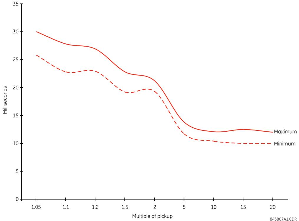
Figure 5-59: PHASE INSTANTANEOUS OVERCURRENT TIMING CURVES
