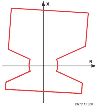
Figure 5-55: LOAD ENCROACHMENT APPLIED TO DISTANCE ELEMENT
