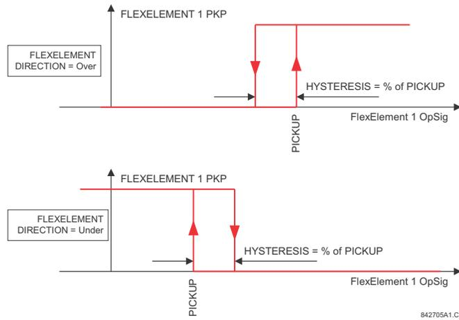
**Figure 5–51: FLEXELEMENT™ DIRECTION, PICKUP, AND HYSTERESIS**
