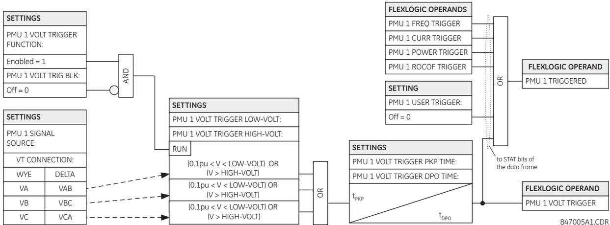
Figure 5-38: VOLTAGE TRIGGER SCHEME LOGIC
