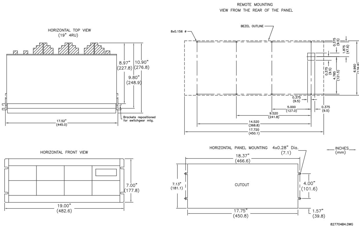
Figure 3-3: F60 HORIZONTAL MOUNTING AND DIMENSIONS (STANDARD PANEL)
