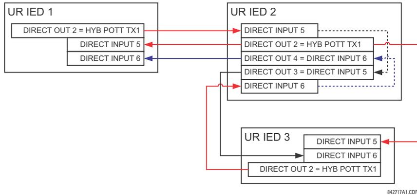
**Figure 5-129: SIGNAL FLOW FOR DIRECT INPUT AND OUTPUT – EXAMPLE 3**
