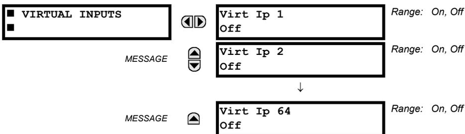
The present status of the 64 virtual inputs is shown here. The first line of a message display indicates the ID of the virtual input. For example, 'Virt Ip 1' refers to the virtual input in terms of the default name. The second line of the display indicates the logic state of the virtual input.
