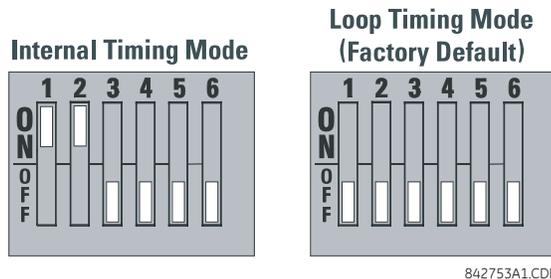
For the internal timing mode, the system clock is generated internally. therefore, the timing switch selection should be internal timing for relay 1 and loop timed for relay 2. There must be only one timing source configured.
