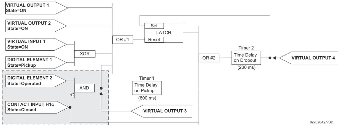
Figure 5-44: LOGIC EXAMPLE WITH VIRTUAL OUTPUTS
