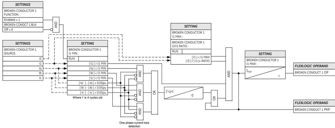
Figure 5-118: BROKEN CONDUCTOR DETECTION LOGIC
