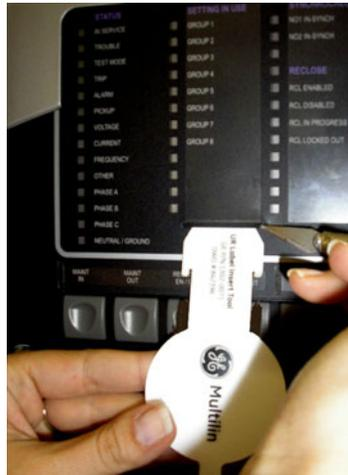
2. Slide the label tool under the LED label until the tabs snap out as shown below. This will attach the label tool to the LED label.
