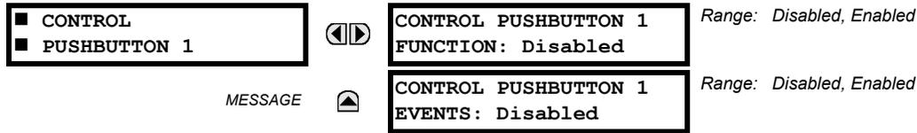
There are three standard control pushbuttons, labeled USER 1, USER 2, and USER 3, on the standard and enhanced front panels. These are user-programmable and can be used for various applications such as performing an LED test, switching setting groups, and invoking and scrolling through user-programmable displays.
