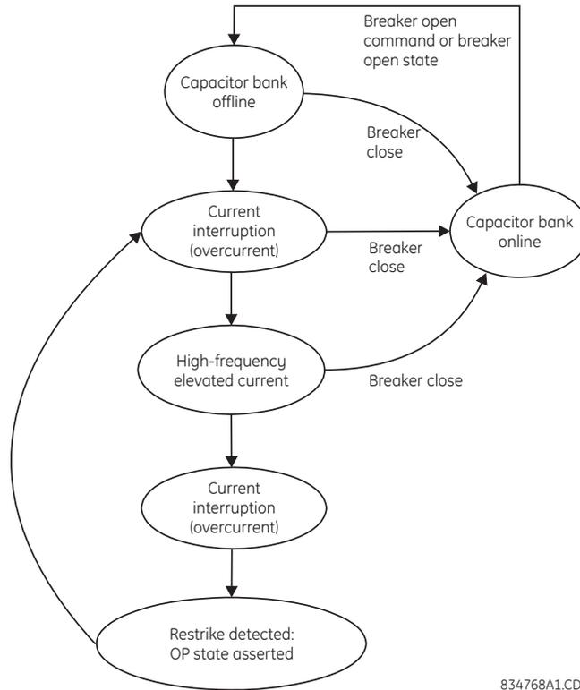
**Figure 5–113: ALGORITHM ILLUSTRATION – STATE MACHINE TO DETECT RESTRIKE**
