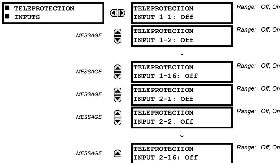
The present state of teleprotection inputs from communication channels 1 and 2 are shown here. The state displayed will be that of corresponding remote output unless the channel is declared failed.
