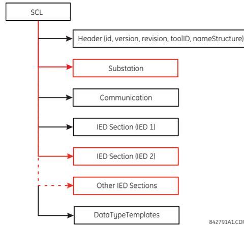
Figure 0-6: SCD FILE STRUCTURE, SCL (ROOT) NODE
