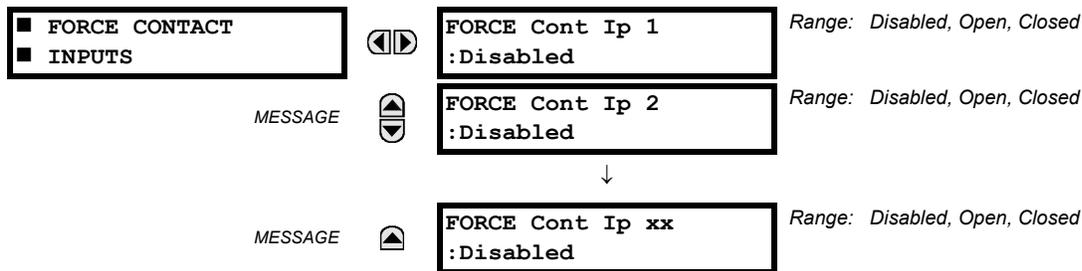
The relay digital inputs (contact inputs) could be pre-programmed to respond to the test mode in the following ways:
