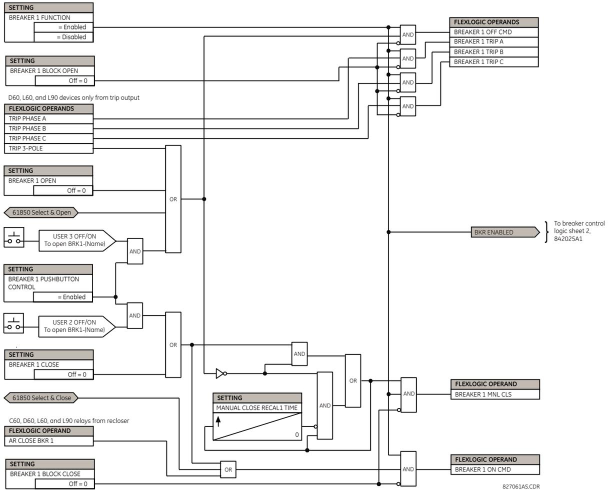
Figure 5-21: DUAL BREAKER CONTROL SCHEME LOGIC (Sheet 1 of 2)
