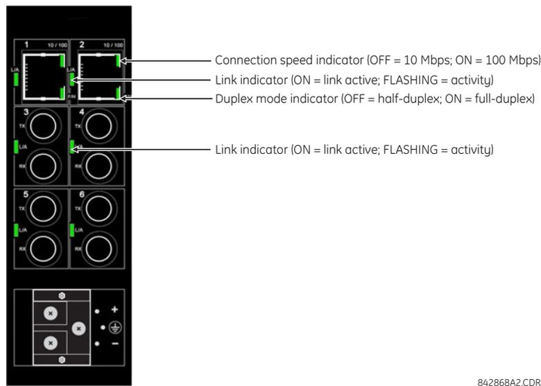
Figure 3–50: ETHERNET SWITCH LED INDICATORS
