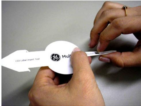
The following procedure describes how to remove the LED labels from the F60 enhanced front panel and insert the custom labels.
