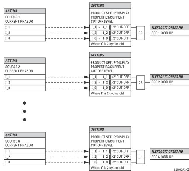
**Figure 5–19: DISTURBANCE DETECTOR LOGIC DIAGRAM**
