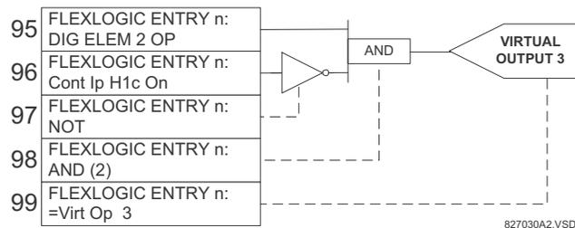
**Figure 5-48: FLEXLOGIC™ EQUATION FOR VIRTUAL OUTPUT 3**
