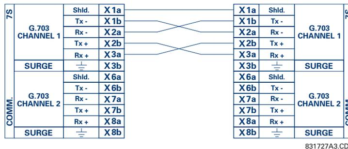
Figure 3–36: TYPICAL PIN INTERCONNECTION BETWEEN TWO G.703 INTERFACES
