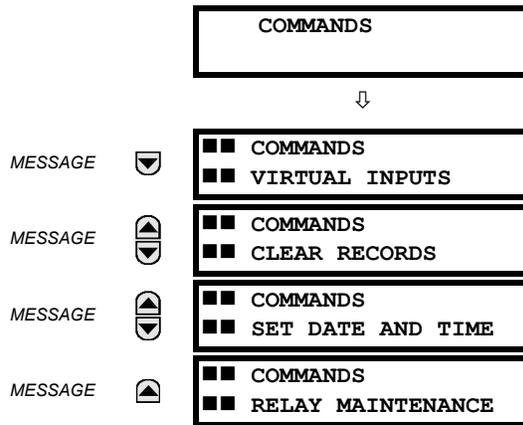
The commands menu contains relay directives intended for operations personnel. All commands can be protected from unauthorized access via the command password; see the *Security* section of chapter 5 for details. The following flash message appears after successfully command entry:
