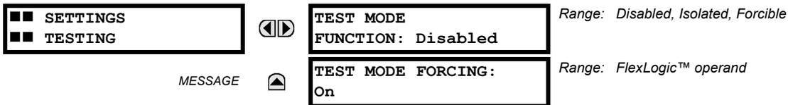
The F60 provides a test facility to verify the functionality of contact inputs and outputs, some communication channels and the phasor measurement unit (where applicable), using simulated conditions. The test mode is indicated on the relay faceplate by a Test Mode LED indicator.
