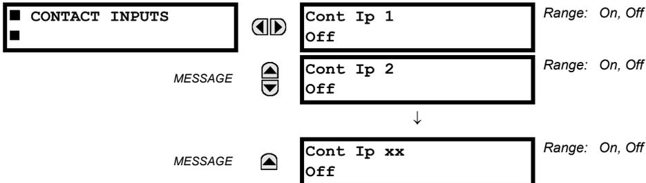
The present status of the contact inputs is shown here. The first line of a message display indicates the ID of the contact input. For example, 'Cont Ip 1' refers to the contact input in terms of the default name-array index. The second line of the display indicates the logic state of the contact input.
