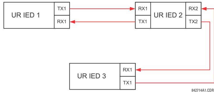
**Figure 5-128: SINGLE-CHANNEL OPEN-LOOP CONFIGURATION**
