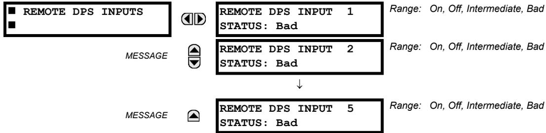
The present state of the remote double-point status inputs is shown here. The actual values indicate if the remote double-point status inputs are in the on (close), off (open), intermediate, or bad state.
