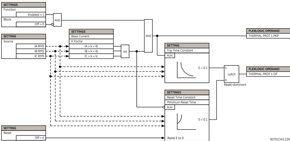
**Figure 5-120: THERMAL OVERLOAD PROTECTION SCHEME LOGIC**
