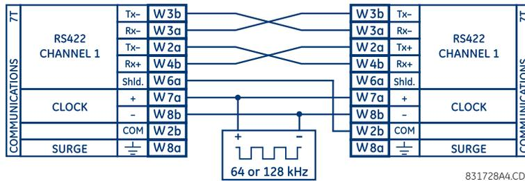
Figure 3-41: TYPICAL PIN INTERCONNECTION BETWEEN TWO RS422 INTERFACES
