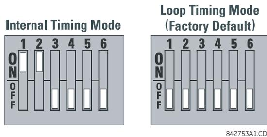
For the internal timing mode, the system clock is generated internally. Therefore, the timing switch selection should be internal timing for relay 1 and loop timed for relay 2. There must be only one timing source configured.
