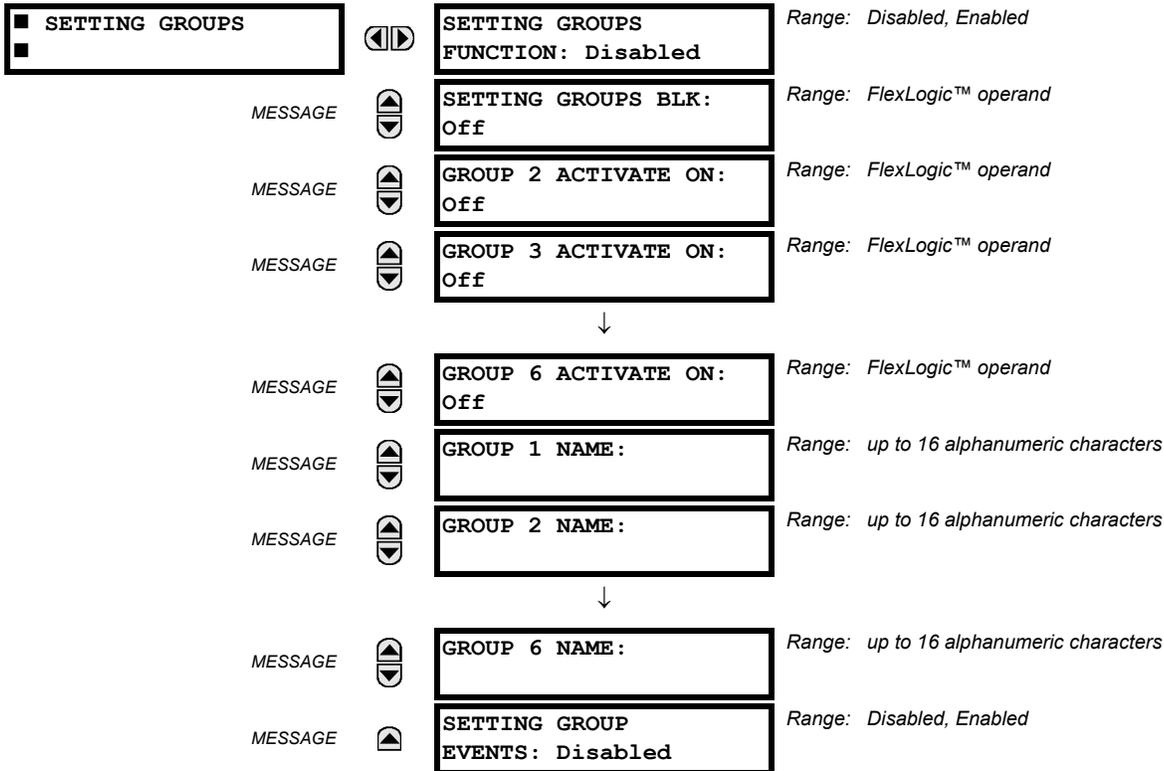
The setting groups menu controls the activation and deactivation of up to six possible groups of settings in the **GROUPED ELEMENTS** settings menu. The faceplate Settings In Use LEDs indicate which active group (with a non-flashing energized LED) is in service.
