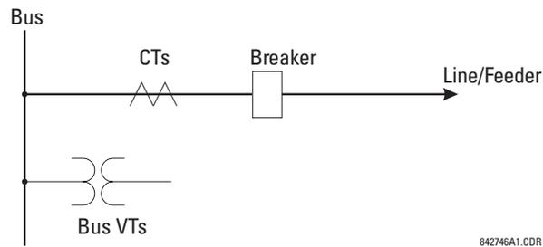
The source 1 (SRC1) phase currents are feeder CTs and phase voltages are bus VTs, and Contact Input 1 is set as Breaker 52a contact. The conditions prior to flashover detection are:
