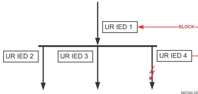
**Figure 5–126: SAMPLE INTERLOCKING BUSBAR PROTECTION SCHEME**
