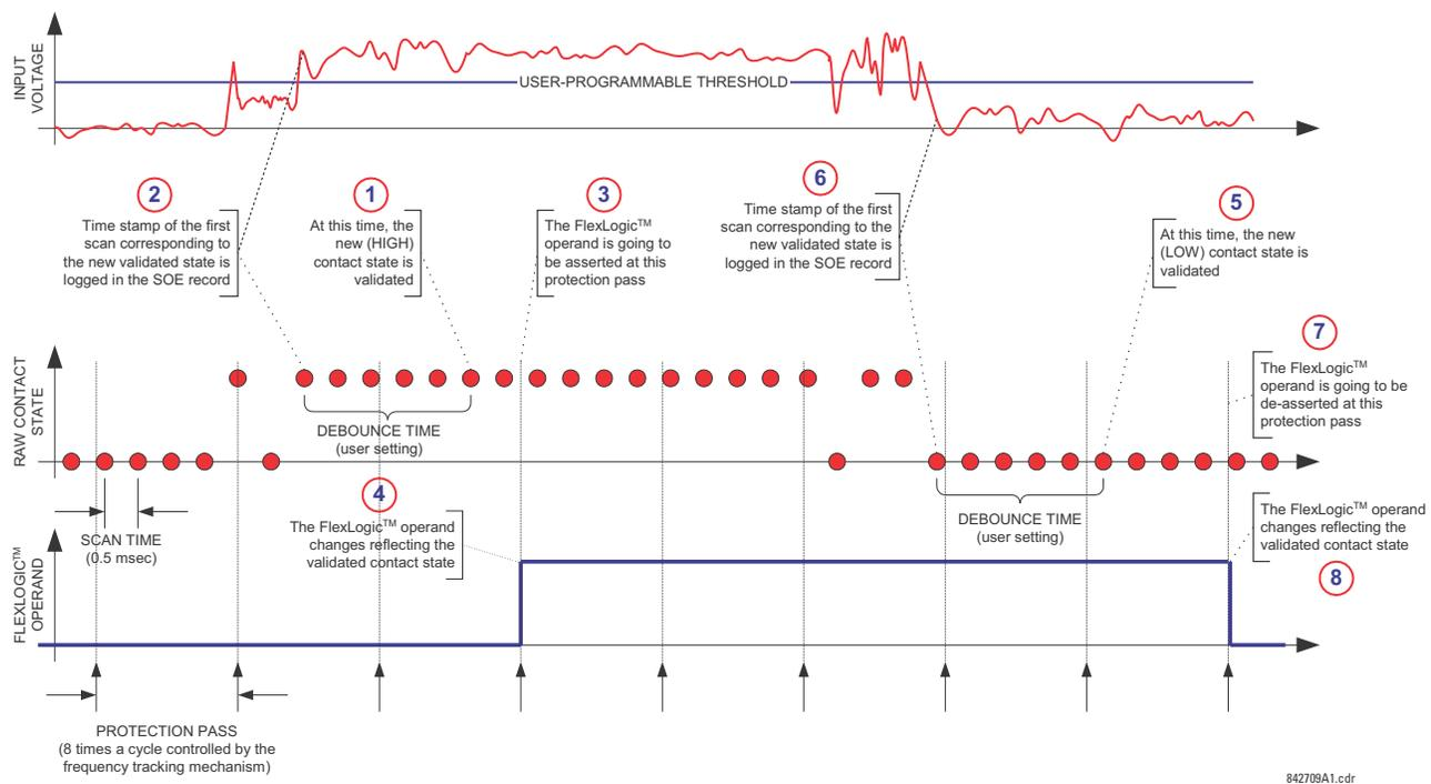
**Figure 5–123: INPUT CONTACT DEBOUNCING MECHANISM AND TIME-STAMPING SAMPLE TIMING**
