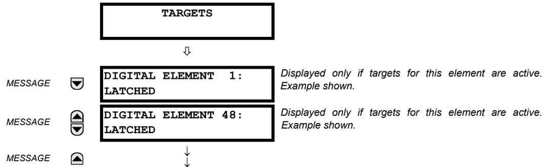
The status of any active targets will be displayed in the targets menu. If no targets are active, the display will read **NO ACTIVE TARGETS**:
