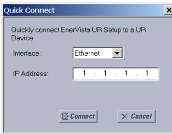
5. Select the **Ethernet** interface and enter the IP address assigned to the F60, then click **Connect**.
