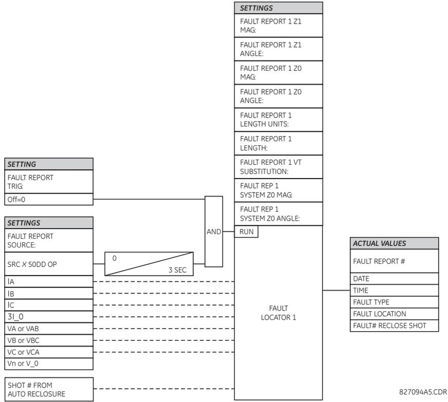
Figure 9-2: FAULT LOCATOR SCHEME
