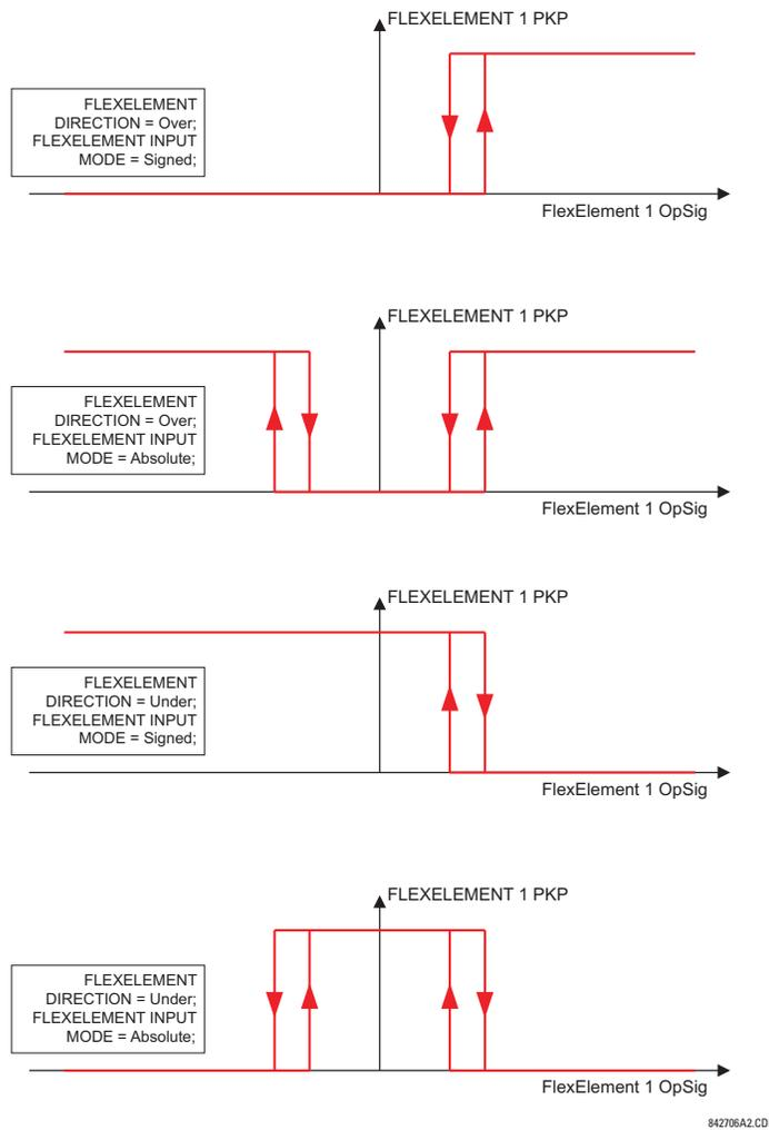
**Figure 5–52: FLEXELEMENT™ INPUT MODE SETTING**
