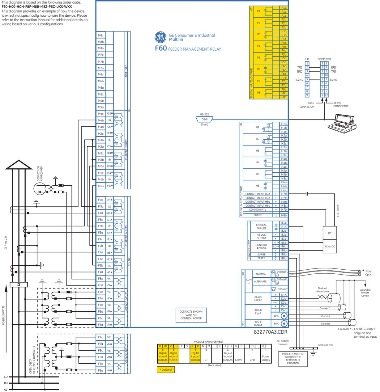
Figure 3-13: TYPICAL WIRING DIAGRAM WITH HIGH-IMPEDANCE DETECTION
