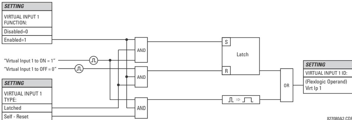
Figure 5–124: VIRTUAL INPUTS SCHEME LOGIC
