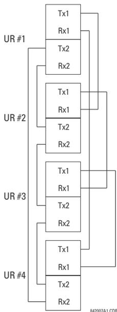
Figure 3–31: DIRECT INPUT AND OUTPUT DUAL CHANNEL CONNECTION
