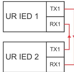
**Figure 5–125: INPUT AND OUTPUT EXTENSION VIA DIRECT INPUTS AND OUTPUTS**
