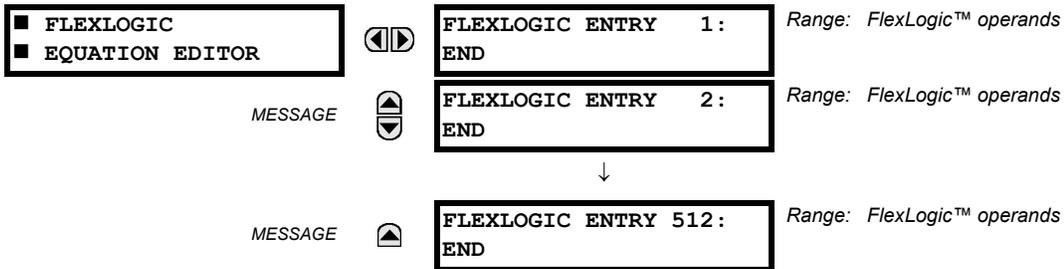
There are 512 FlexLogic™ entries available, numbered from 1 to 512, with default END entry settings. If a "Disabled" Element is selected as a FlexLogic™ entry, the associated state flag will never be set to '1'. The '+/-' key may be used when editing FlexLogic™ equations from the keypad to quickly scan through the major parameter types.
