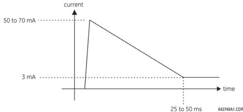
**Figure 3-22: CURRENT THROUGH CONTACT INPUTS WITH AUTO-BURNISHING**
