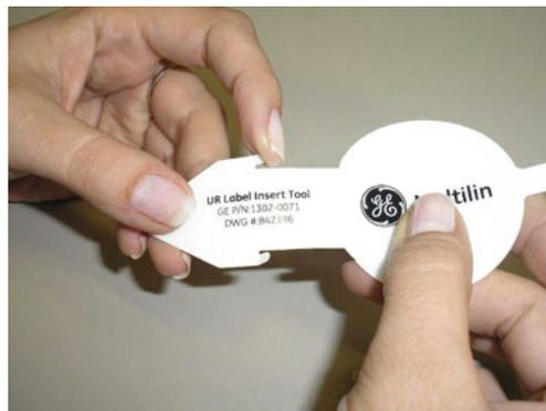
2. Bend the tab at the center of the tool tail as shown below.
