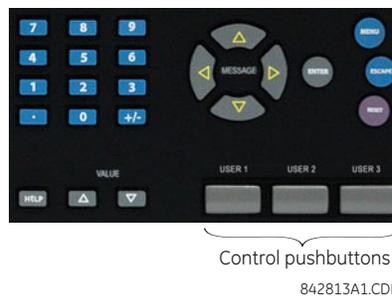
Figure 5-5: CONTROL PUSHBUTTONS (ENHANCED FACEPLATE)
