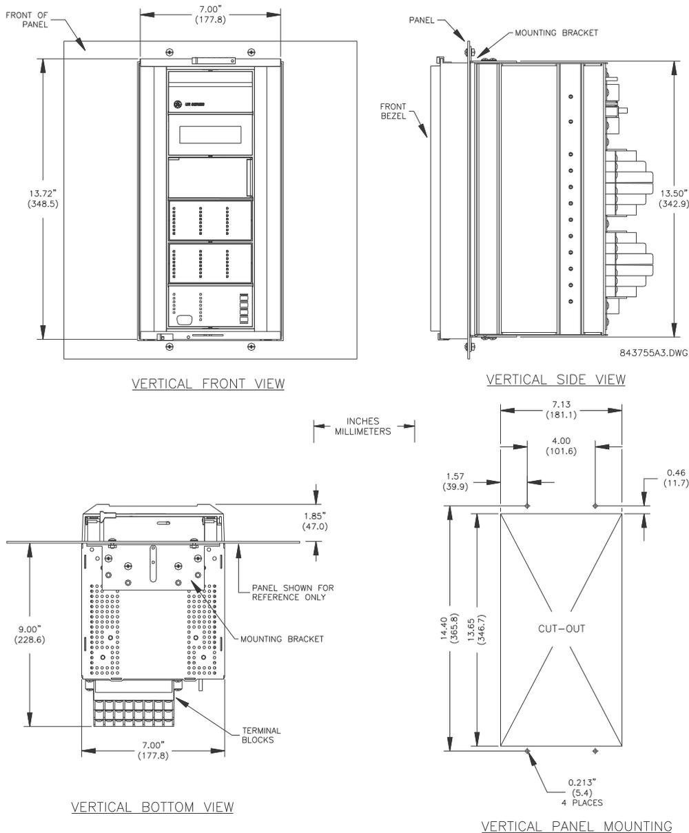
**Figure 3-5: F60 VERTICAL MOUNTING AND DIMENSIONS (STANDARD PANEL)**
