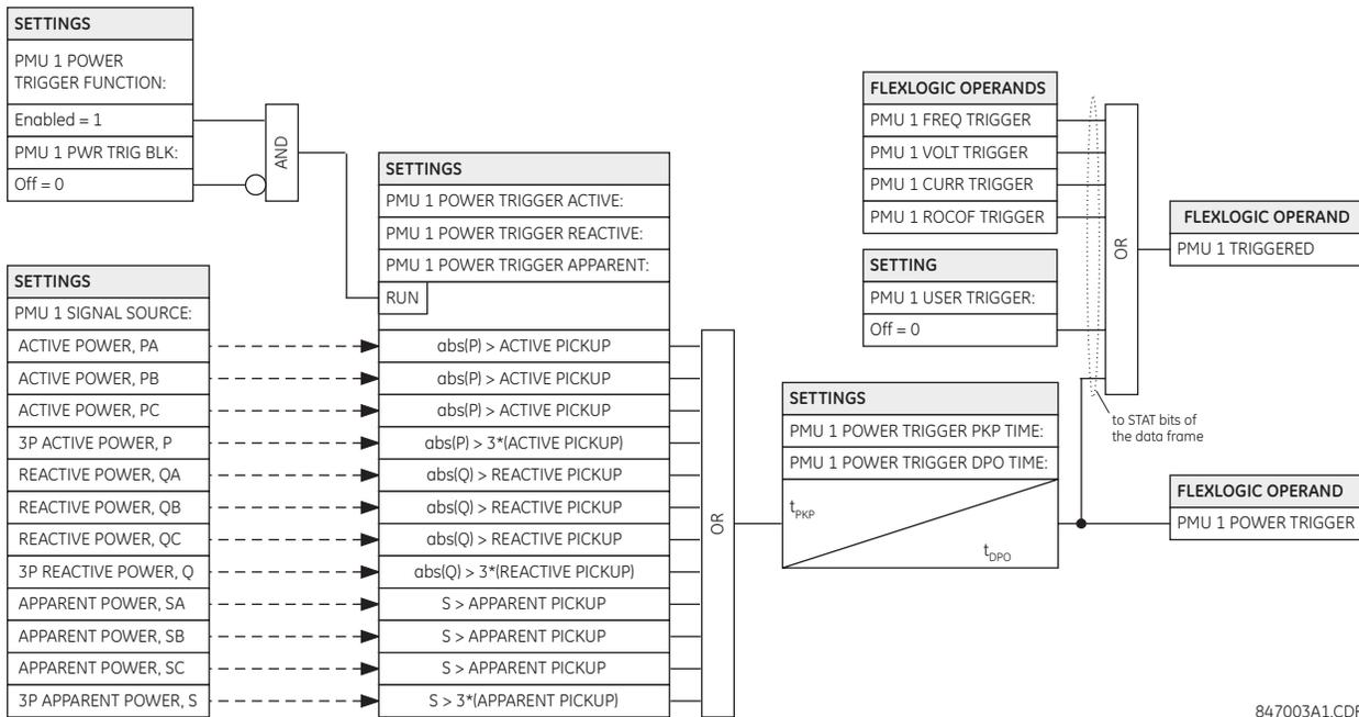
Figure 5-40: POWER TRIGGER SCHEME LOGIC
