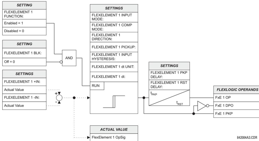
Figure 5-50: FLEXELEMENT™ SCHEME LOGIC
