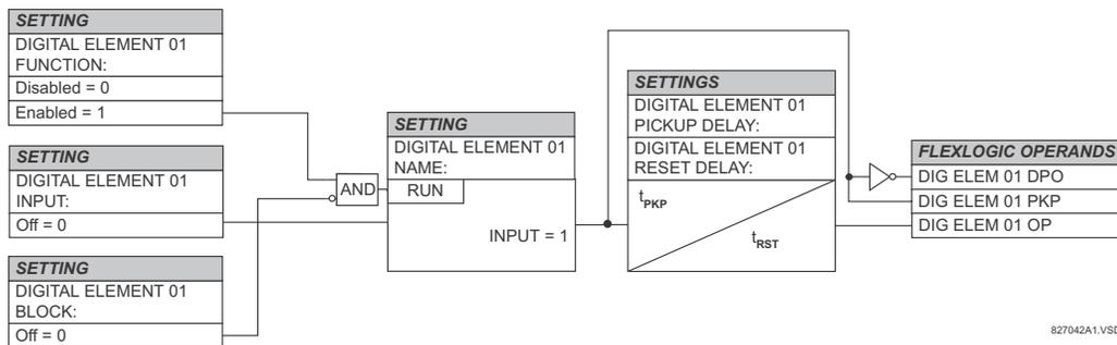
Figure 5-104: DIGITAL ELEMENT SCHEME LOGIC
