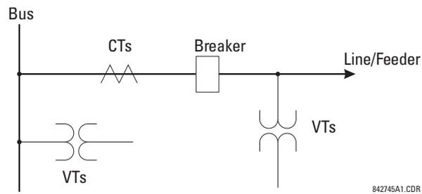
The source 1 (SRC1) phase currents are CTs and phase voltages are bus VTs. The source 2 (SRC2) phase voltages are line VTs. Contact input 1 is set as the breaker 52a contact (optional).
