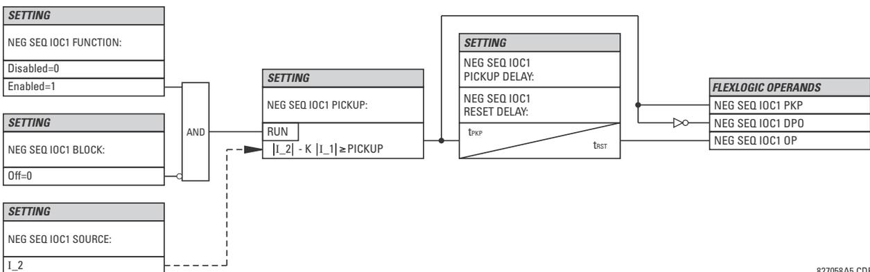
Figure 5-72: NEGATIVE SEQUENCE IOC1 SCHEME LOGIC
