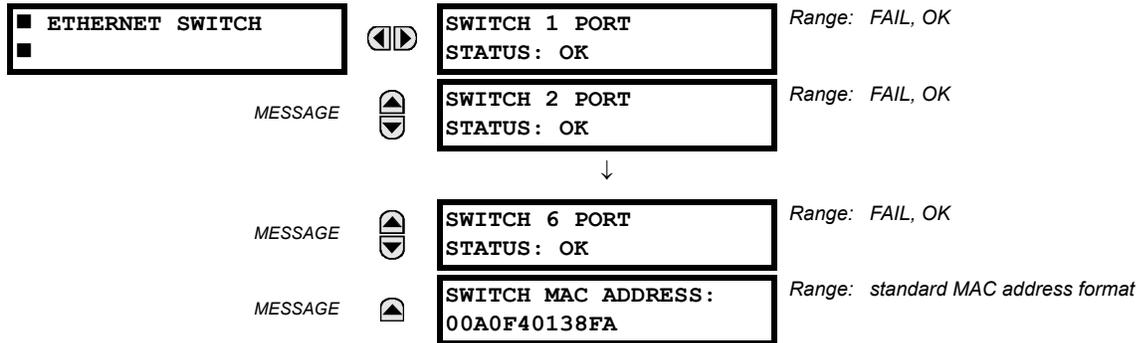
These actual values appear only if the F60 is ordered with an Ethernet switch module (type 2S or 2T). The status information for the Ethernet switch is shown in this menu.
