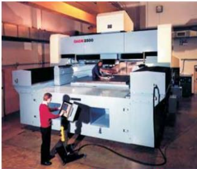
26 Tonne Bridge Driven by Friction Drives
