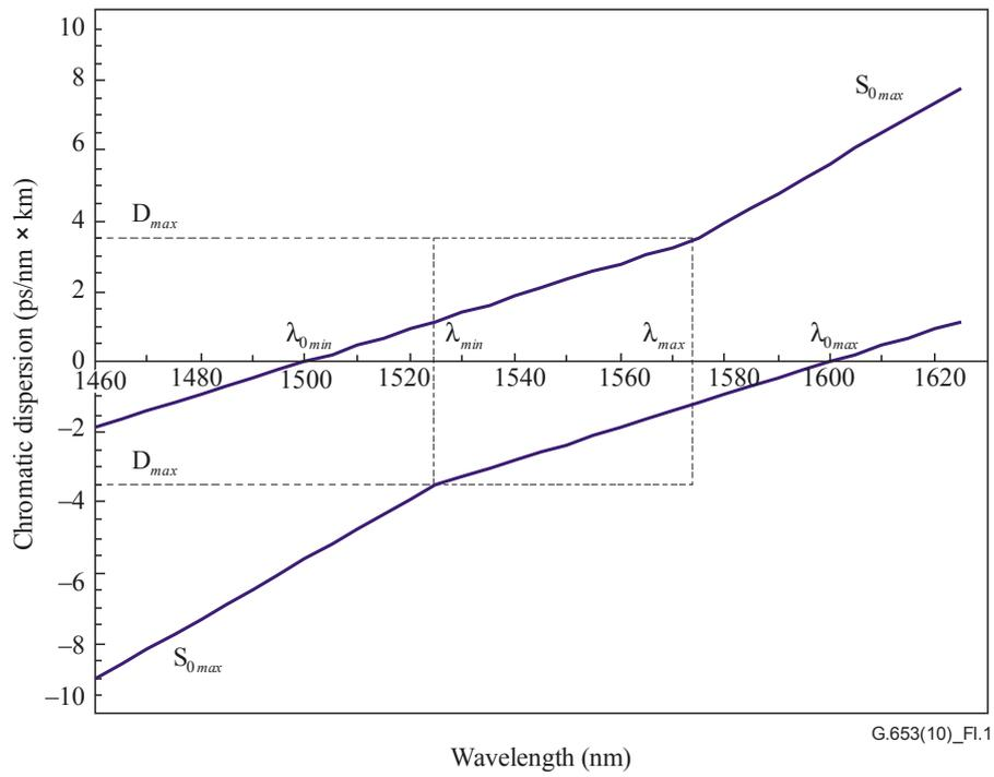
**Figure I.1 – Table 2 fibre dispersion boundary**
