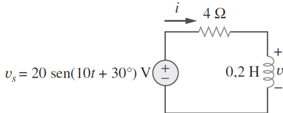
Resposta:  $v(t) = 8,94 \text{ sen}(10t + 93,43^\circ) \text{ V}$
