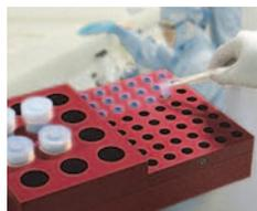
Sample preparation by metal-free heating plates
