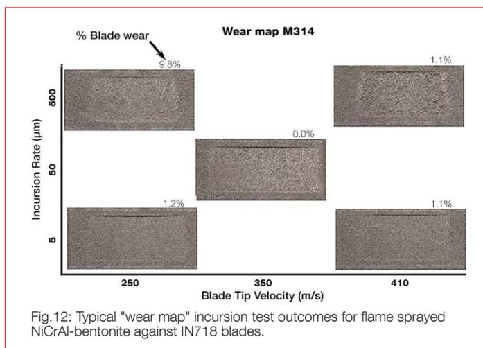
Fig. 12: Typical "wear map" incursion test outcomes for flame sprayed NiCrAl-bentonite against IN718 blades.
