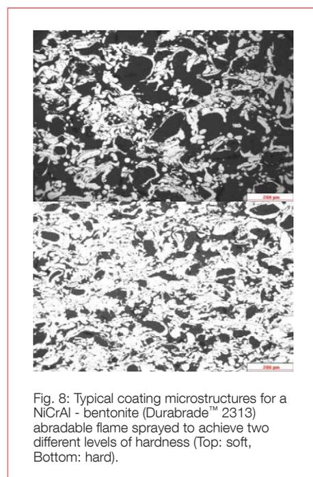
Fig. 8: Typical coating microstructures for a NiCrAl - bentonite (Durabrade™ 2313) abrasible flame sprayed to achieve two different levels of hardness (Top: soft, Bottom: hard).
