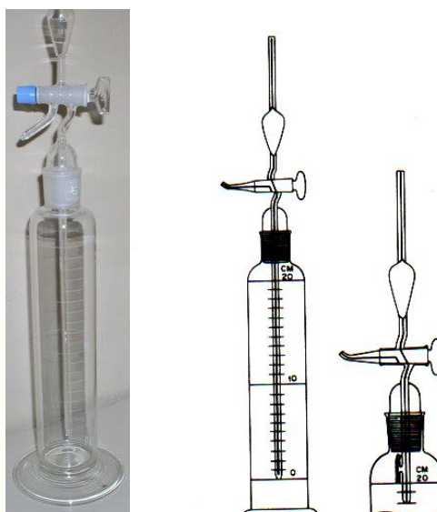
Figure 9.1 Andreasen's fixed-position apparatus (Gallenkamp).
