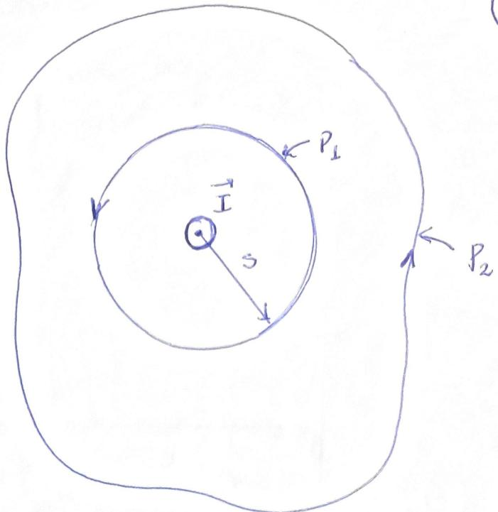
$$\oint_{P_1} \vec{B} \cdot d\vec{l} = \int_0^{2\pi} \left( \frac{\mu_0 I}{2\pi s} \hat{\phi} \right) \cdot (s d\phi \hat{\phi}) = \frac{\mu_0 I}{2\pi} \int_0^{2\pi} d\phi = \mu_0 I$$
