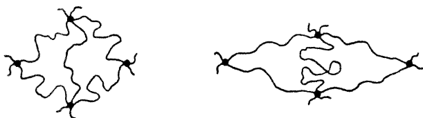
Figure 9.8 The stretching of rubber
