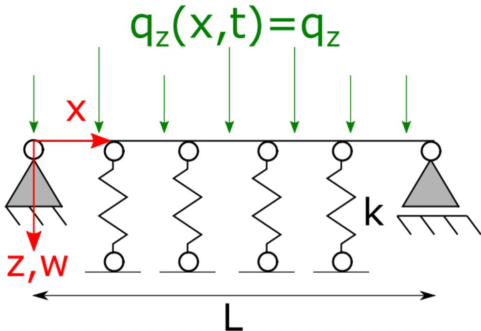
Transverse vibration of a pinned-pinned beam on elastic (Winkler) foundation.
