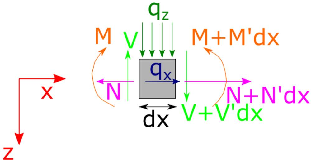
The beam has mass *per* unit length  $\mu$ , bending stiffness  $EI$  and is subjected to transverse and longitudinal loads  $q_z$  and  $q_x$ . The second Newton's law applied to the differential element reads (see figure above):
