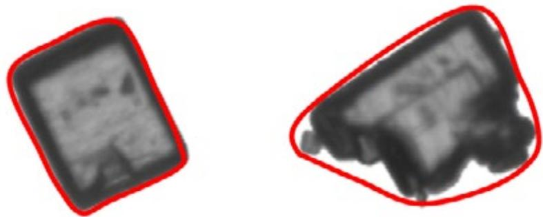
Illustration of the convex hull for two different shapes of particle.
