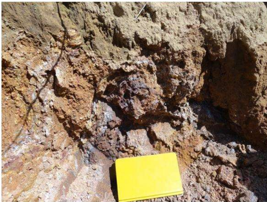
Figure 14 - Typical Mineralization São Rubens and São Manuel - Graphite layers in Dark Colors and Disseminated Graphite in Lighter Colors
