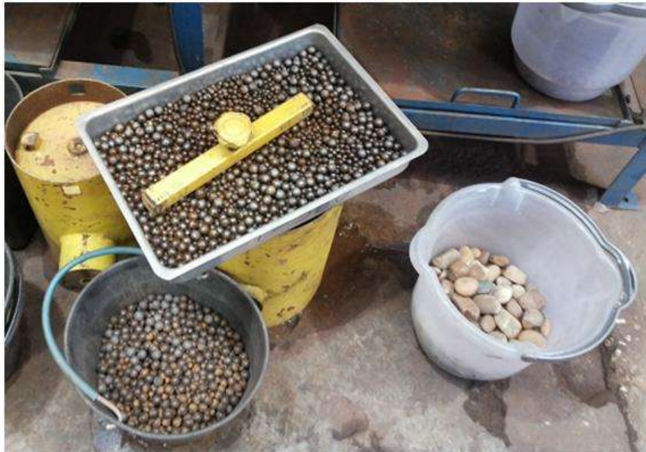
Figure 22 - Grinding Media Steel Shot (“granalha”) on Left and Pebbles on Right
