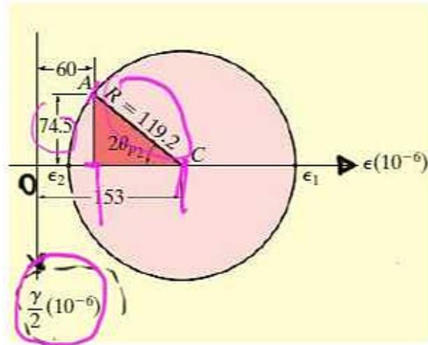
$$\begin{aligned}\epsilon_x &= 60 \times 10^{-6} \\ \epsilon_y &= 246 \times 10^{-6} \\ \gamma_{xy} &= -149 \times 10^{-6}\end{aligned}$$
