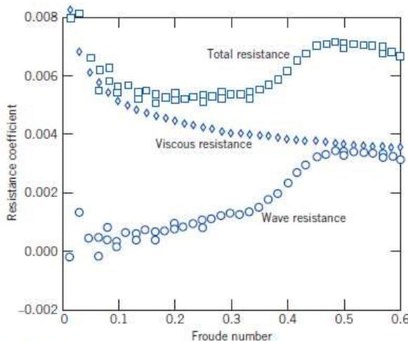
**Fig. 7.2** Data from test of 1:80 scale model of U.S. Navy guided missile frigate *Oliver Hazard Perry* (FFG-7). (Data from U.S. Naval Academy Hydromechanics Laboratory, courtesy of Professor Bruce Johnson.)
