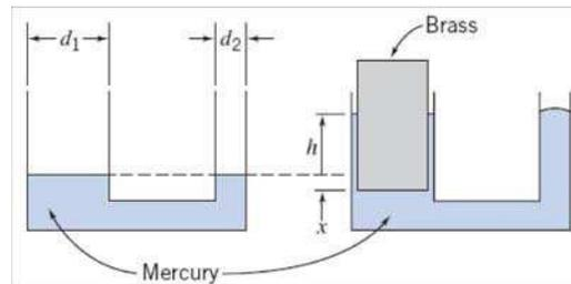
**Given:** Container of mercury with vertical tubes of known diameter, brass cylinder of known dimensions introduced into larger tube, where it floats.
