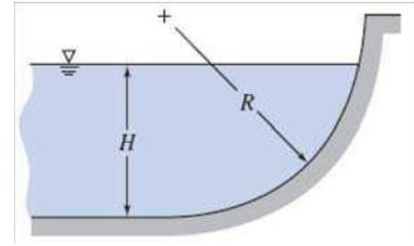
**Given:** Curved surface, in shape of quarter cylinder, with given radius  $R$  and width  $w$ ; liquid concrete stands to depth  $H$ .
