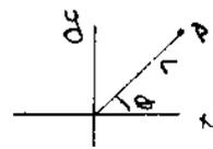
$$\psi = \psi_{\text{unif}} + \psi_{\text{sink}} = Uy - \frac{q\theta}{2\pi} = U r \sin\theta - \frac{q\theta}{2\pi} \quad \dots (1)$$
