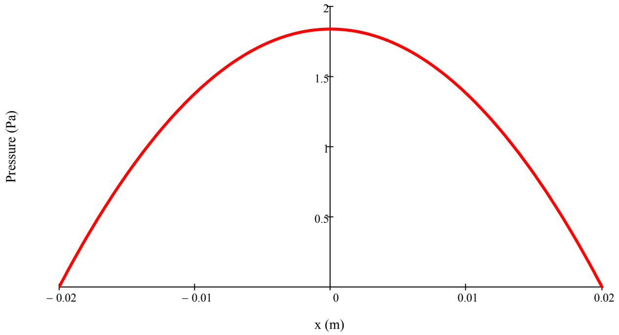
The net force is such that the chip is floating on air due to a Bernoulli effect: the speed is maximum at the edges and zero at the center; pressure has the opposite trend - pressure is minimum ( $p_{\text{atm}}$ ) at the edges and maximum at the center.
