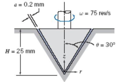
**Given:** Conical bearing geometry
