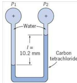
**Given:** Two-fluid manometer as shown
