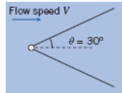
**Given:** Sharp object causing waves
