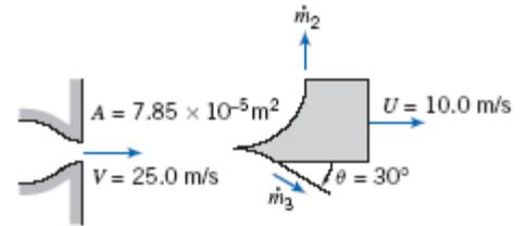
**Given:** Jet impacting a splitter vane
