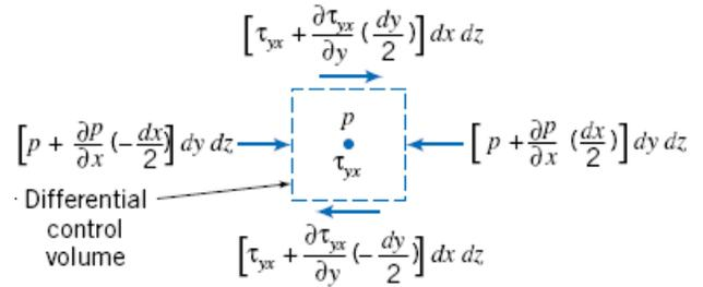
Using the analysis of Section 8.2, the sum of forces in the x direction is
