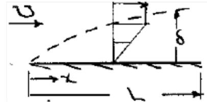
$$\frac{\theta}{\delta} = \int_0^1 \frac{u}{U} \cdot \left( 1 - \frac{u}{U} \right) d\eta \quad \text{(Momentum thickness)}$$
