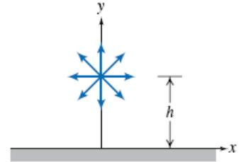
where  $q = 2 \text{ m}^3/\text{s}$ . The fluid density is  $1000 \text{ kg/m}^3$  and body forces are negligible. Derive expressions for the velocity and acceleration of a fluid particle that moves along the wall, and plot from  $x=0$  to  $x=+10h$ . Verify that the velocity and acceleration normal to the wall are zero. Plot the pressure gradient  $\partial p/\partial x$  along the wall. Is the pressure gradient along the wall adverse (does it oppose fluid motion) or not?
