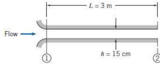
**Given:** Channel flow with laminar boundary layers
