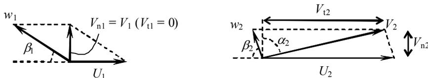
From continuity  $V_n = \frac{Q}{2 \cdot \pi \cdot r \cdot b} = w \cdot \sin(\beta)$   $w = \frac{V_n}{\sin(\beta)}$   $\frac{V_{n1}}{V_{n2}} = \frac{A_2}{A_1} = \frac{r_2 \cdot b_2}{r_1 \cdot b_1}$
