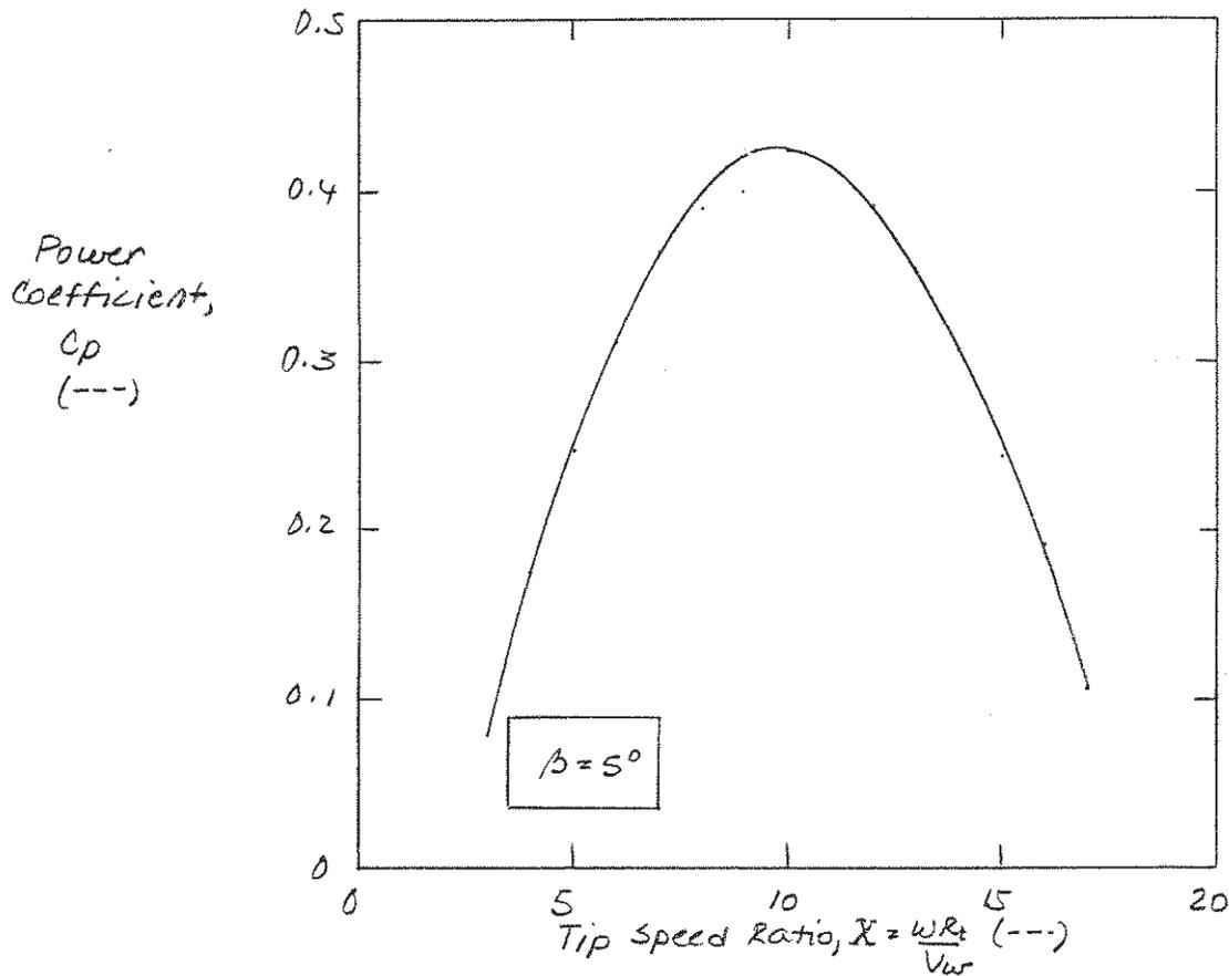
Trends shown are similar to Fig. 10.45. At small  $X$ , the blade is entirely stalled so useful output is low. At large  $X$ ,  $\alpha$  becomes negative near the tips, reducing output.
