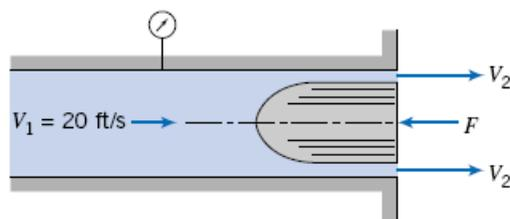
**Given:** Water flow out of tube
