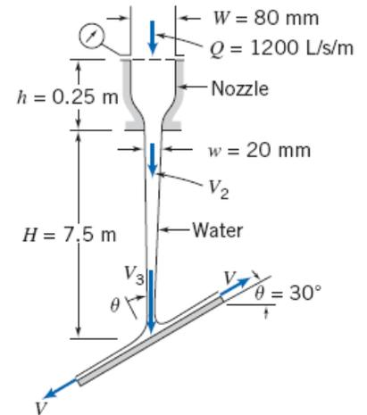
**Given:** Nozzle flow striking inclined plate
