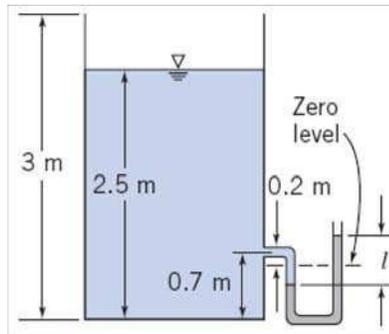
**Given:** A U-tube manometer is connected to the open tank filled with water as shown (manometer fluid is Meriam blue)
