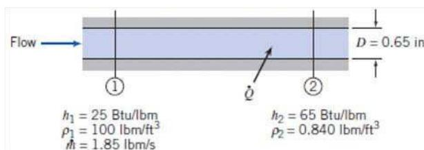
**Given:** Frictionless flow of Freon in a tube
