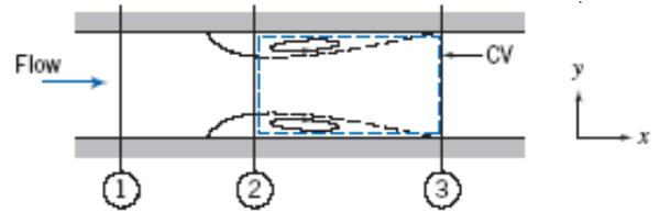
Solution: Apply the Bernoulli, continuity, momentum and energy equations, using the CV shown.
