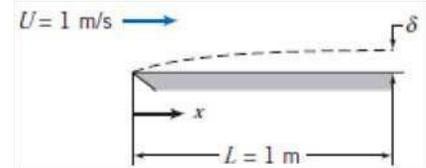
**Given:** Turbulent boundary layer flow of water
