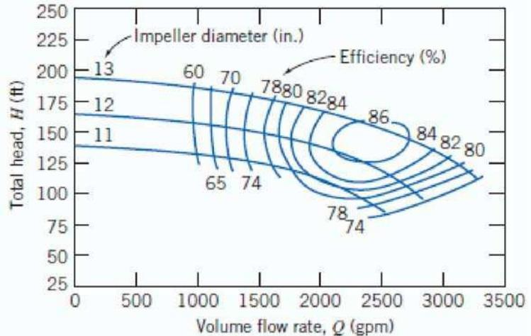
Solution: From the graph, BEP occurs for the 12 in. impeller at
