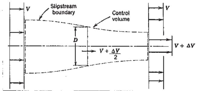
Assumptions: (1) Steady flow, (2) Incompressible flow, (3) Uniform flow, (4) Frictionless flow
