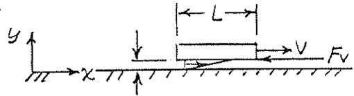
Assume: (1) Newtonian fluid (2) Linear velocity profile in narrow gap (3) Air at STP
