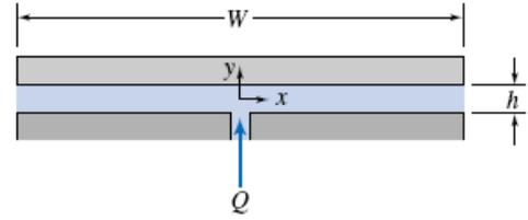
**Given:** Hydrostatic bearing
