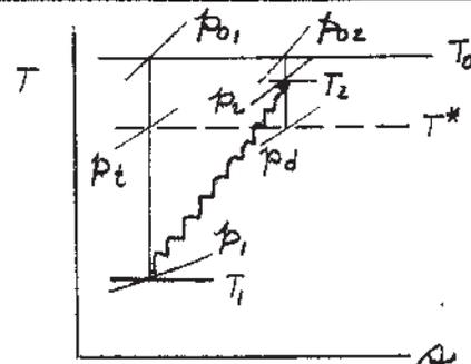
$$\Delta s = -53.3 \frac{\text{ft} \cdot \text{lb}}{\text{lbm} \cdot \text{R}} \times \ln(0.5395) \times \frac{\text{Btu}}{778 \text{ ft} \cdot \text{lb}} = 0.0423 \text{ Btu/lbm} \cdot \text{R}$$
