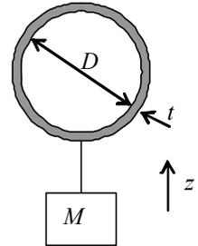
Taking a free body diagram of the balloon and payload:  $\Sigma F_z = F_{buoy} - M_{He} \cdot g - M_s \cdot g - M \cdot g = 0$
