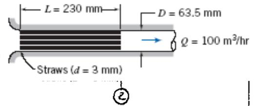
Solution: Apply energy equation for steady, incompressible pipe flow.
