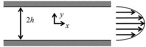
**Given:** Laminar flow between flat plates
