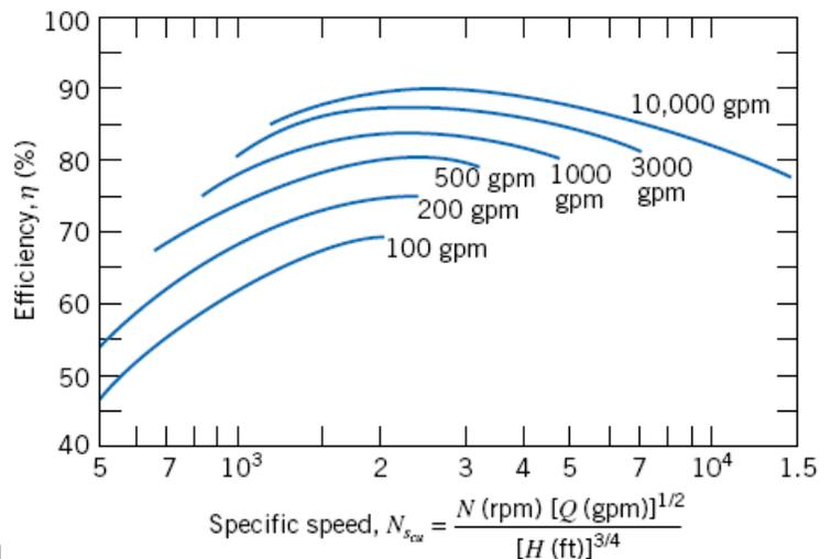
The nearest standard speed to  $N = 2410$  rpm should be used
