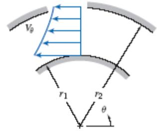
$$k = w \ln\left(\frac{r_2}{r_1}\right) \sqrt{\frac{2r_1^2 r_2^2}{\rho(r_2^2 - r_1^2)}}$$
