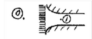
$$\left( \frac{p_0}{\rho} + \frac{U_0^2}{2} \right) - \left( \frac{p_1}{\rho} + \frac{U_1^2}{2} \right) = h_{IT} \quad \text{Since } U_0 = 0 \text{ and } p_0 = p_{\text{atm}} = 0 \text{ we can solve for the pressure at 1:}$$
