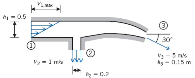
**Given:** Data on flow at inlet and outlet of a reducing elbow
