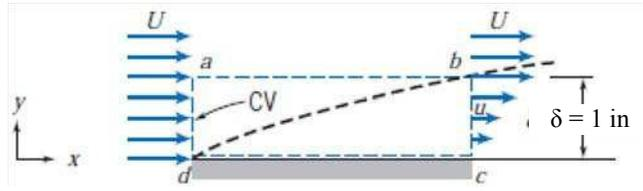
**Given:** Flow over a flat plate with parabolic laminar boundary layer profile
