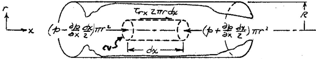
Solution: The forces on a CV of radius  $r$  are shown above.
