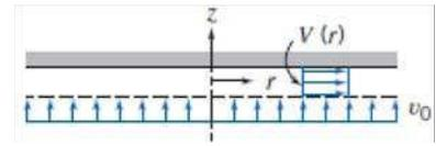
**Given:** Flow between parallel disks through porous surface
