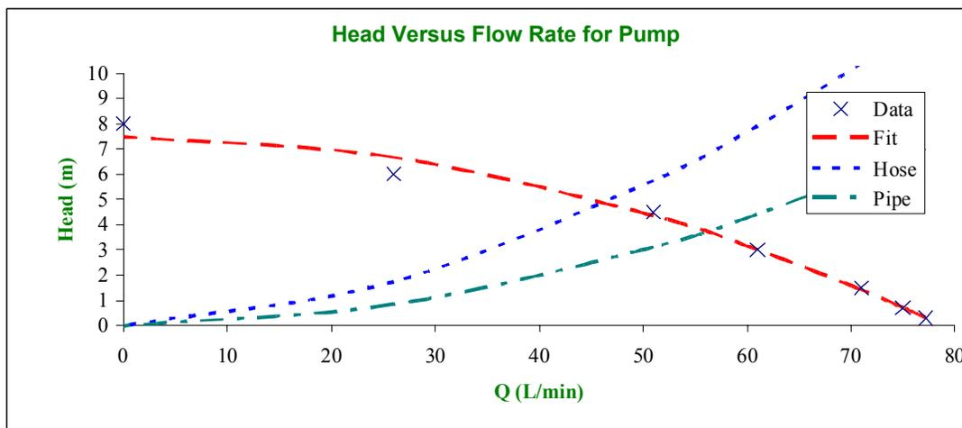
To determine the discharge heights for the hose and the pipe, we subtract the head loss from the head generated by the pump.
