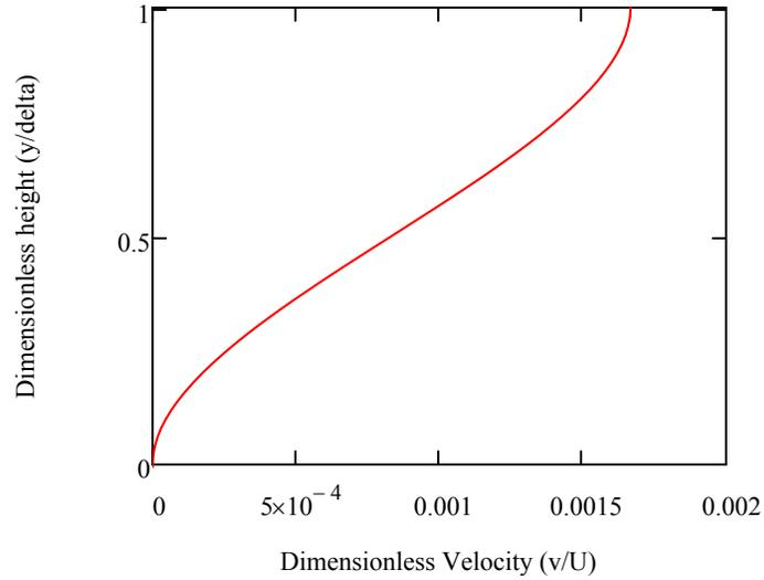
The maximum value of  $v/U$  is where  $y = \delta$ :  $v_{\text{ratmax}} = \frac{v}{U} = \frac{\delta}{x} \cdot \left( \frac{1}{2} - \frac{1}{3} \right) = \frac{\delta}{6 \cdot x} \quad v_{\text{ratmax}} = \frac{5 \times 10^{-3} \cdot \text{m}}{6 \times 0.5 \cdot \text{m}} \quad v_{\text{ratmax}} = 0.00167$
