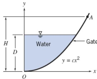
**Given:** Parabolic gate, hinged at  $O$  has a constant width.
