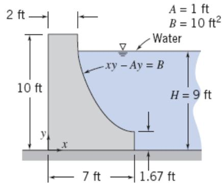
**Given:** Dam with cross-section shown. Width of dam  $b = 160$  ft
