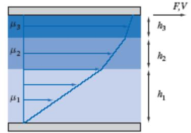
**Given:** Flow of three fluids between two plates
