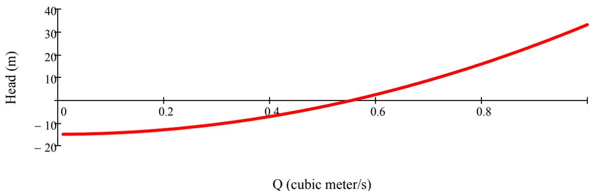
The above graph can be plotted in Excel. In Excel, Solver can be used to find Q for  $H_p = 0$   $Q = 0.557 \frac{\text{m}^3}{\text{s}}$  (Zero power rate)
