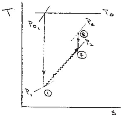
The actual exit Mach number would be higher than the estimate based on isentropic flow downstream from the shock.
