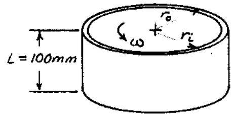
Solution: "Unfold" bearing since gap is small, and consider as flow between parallel plates. Apply Newton's law of viscosity.
