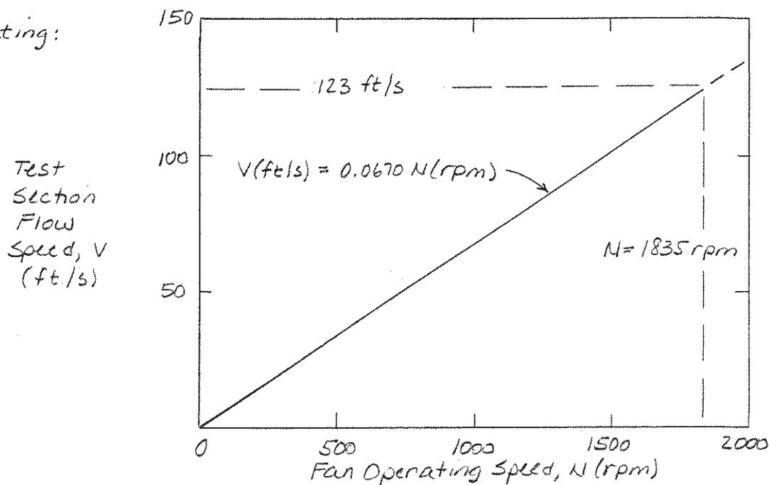
The slope of the linear relationship is  $\frac{V}{N} = 123 \frac{\text{ft}}{\text{s}} \times \frac{1}{1835 \text{ rpm}} = 0.0670 \text{ ft/s/rpm}$ .
