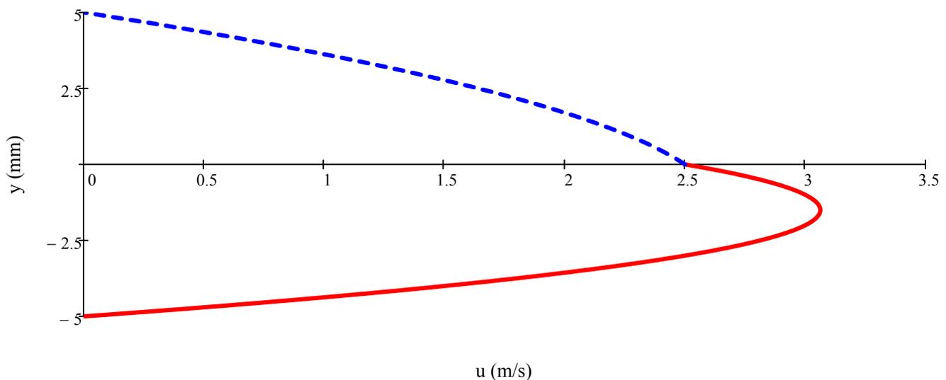
Clearly,  $u_1$  has the maximum velocity, when  $\frac{du_1}{dy} = 0$  or  $2 \cdot y_{\text{max}} + h \cdot \frac{(\mu_2 - \mu_1)}{(\mu_2 + \mu_1)} = 0$
