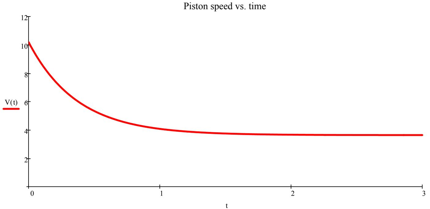
The terminal speed of the piston,  $V_t$ , is evaluated as  $t$  approaches infinity
