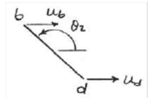
$$u_b = u_d + \frac{\partial}{\partial y} u \cdot (1 \cdot \sin(\theta_2)) \quad -\omega_{bd} = \frac{(u_d - u_b) \cdot \sin(\theta_2)}{l} \quad \text{since the component normal to } l \text{ is } u \cdot \sin(\theta_2)$$
