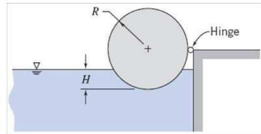
**Given:** Cylinder of mass  $M$ , length  $L$ , and radius  $R$  is hinged along its length and immersed in an incompressible liquid to depth  $H$ .
