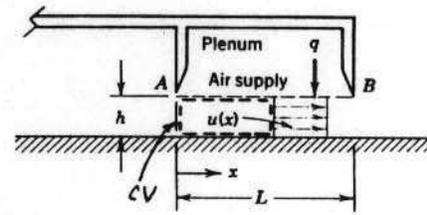
Solution: Choose a CV in the gap, from 0 to  $x$ , as shown.
