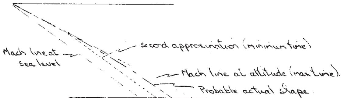
Since  $T$  is constant for  $y > y_0 = 11 \text{ km}$ , the second approximation which assumes the Mach line at sea level for  $0 < y \leq 11 \text{ km}$  gives the minimum time
