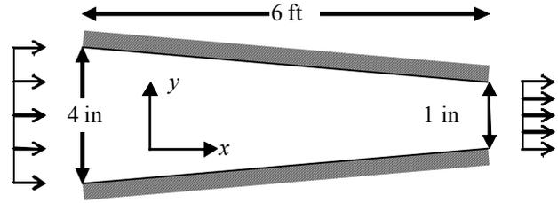
**Given:** Flow in a pipe with variable diameter
