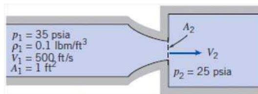
**Given:** Ideal gas flow in a converging nozzle
