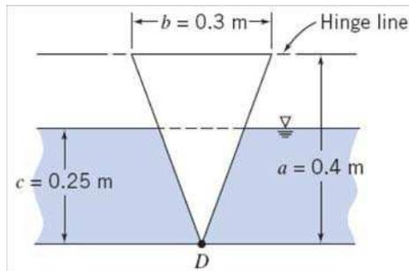
**Given:** Window, in shape of isosceles triangle and hinged at the top is located in the vertical wall of a form that contains concrete.
