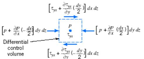
Simplifying  $\frac{d\tau}{dy} = \frac{dp}{dx} = k$  so for each fluid  $\mu \cdot \frac{d^2}{dy^2} u = k$
