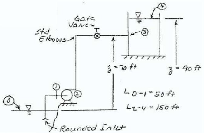
Solution: Apply the energy equation for pipe flow. The pump must overcome the gravity lift plus the head losses in the pipe and fittings.
