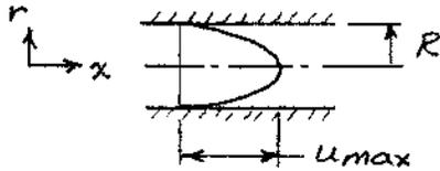
Solution: Apply definition of kinetic energy coefficient,
