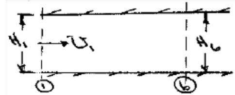
**Given:** Laboratory wind tunnel has flexible wall to accommodate BL growth. BL's are well represented by  $1/7$ -power profile. Information at two stations are known:
