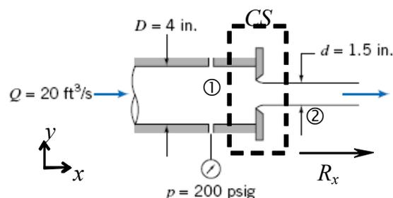
**Given:** Water flow through orifice plate
