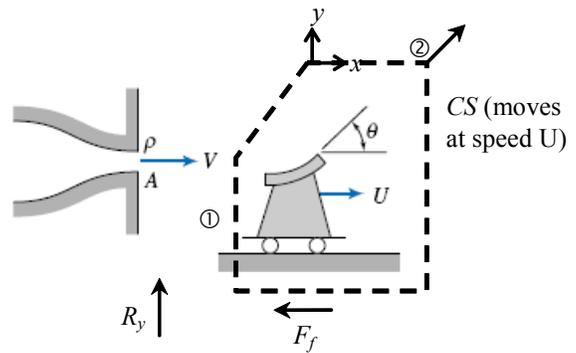
**Given:** Water jet striking moving vane
