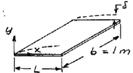
The viscous drag for the two sides of the plate is:  $F_D = 2 \cdot \int_0^L \tau_w \cdot b \, dx$  The wall shear stress  $\tau_w$  is:
