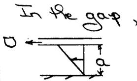
In the gap,  $\tau = \mu \frac{du}{dy} = \mu \frac{u}{a} = \frac{\mu R \omega}{a}$
