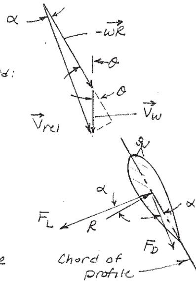
Lift force ( $F_L$ ) is normal to  $\vec{V}_{rel}$  and drag force ( $F_D$ ) is parallel to  $\vec{V}_{rel}$ . Thus
