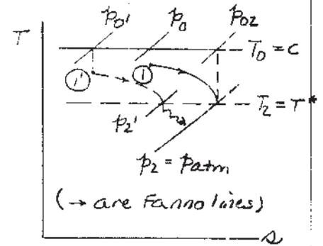
Assume steady, 1-D compressible flow, with constant stagnation temperature,  $T_0 = 15^\circ\text{C}$  (59°F)
