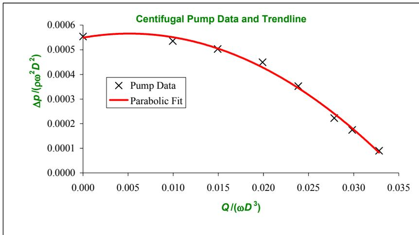
The curve fit result is:  $\Delta p/(\rho \omega^2 D^2) = -0.6302 (Q/(\omega D^3))^2 + 0.006476 (Q/(\omega D^3)) + 0.0005490$
