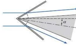
**Given:** Airfoil with included angle of  $60^\circ$
