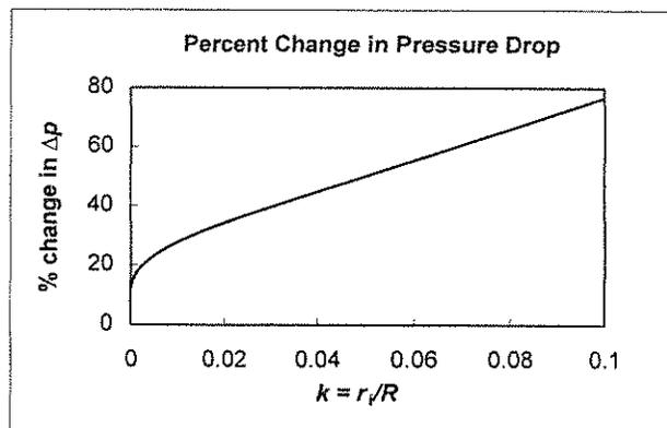
The plot shows that even the smallest of wires causes a significant increase in pressure drop for a given flow rate.
