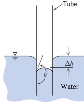
**Given:** Water in a tube or between parallel plates
