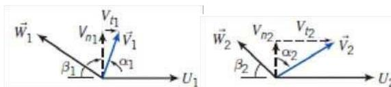
**Given:** Geometry of centrifugal pump
