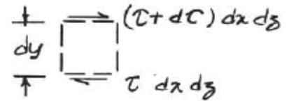
The differential of shear force would be:  $dF_{\text{shear}} = (\tau + d\tau) \cdot dx \cdot dz - \tau \cdot dx \cdot dz = d\tau \cdot dx \cdot dz$  and  $\frac{dF_{\text{sx}}}{dV} = \frac{d\tau}{dy} = \frac{d}{dy} \left( \mu \cdot \frac{du}{dy} \right) = \mu \cdot \frac{d^2}{dy^2} u$
