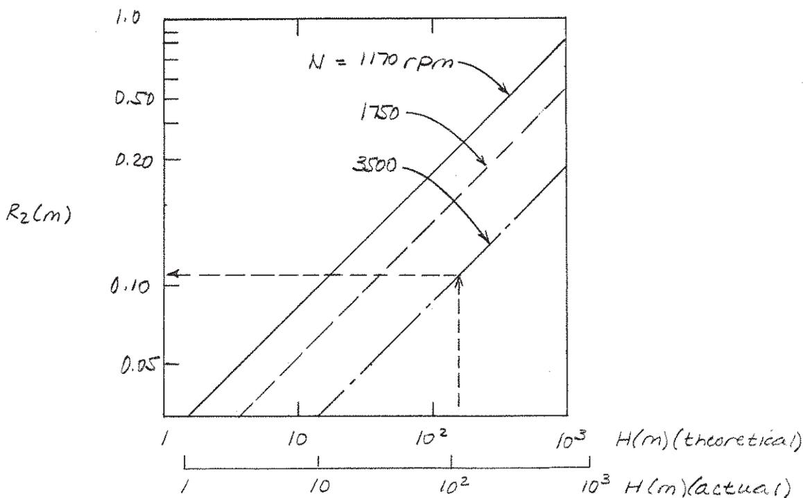
For a given application, enter the abscissa with the desired head, move up to the desired driver speed, then move left to the ordinate and read the required impeller radius. The example (--- line) illustrates.
