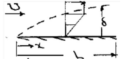
For the linear velocity profile:  $\frac{\theta}{\delta} = \int_0^1 \eta \cdot (1 - \eta) d\eta = \int_0^1 (\eta - \eta^2) d\eta$  Evaluating this integral:  $\frac{\theta}{\delta} = \frac{1}{6} = 0.1667$
