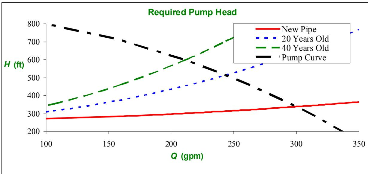
Sizing the pump for 800 L/min for at 40 years would (assuming no change in the pump characteristics) produce 922 L/min at 20 years and 1136 L/min for new pipe.
