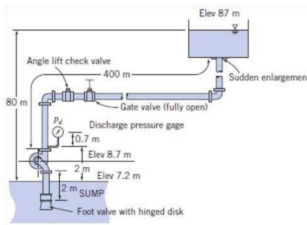
Assumptions: 1)  $p_{ent} = p_{exit} = p_{atm}$  2)  $V_{ent} = V_{exit} = 0$
