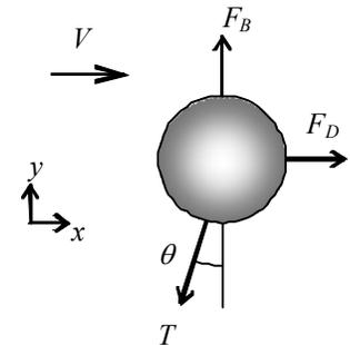
Based on a free body diagram of the balloon,  $F_D = F_B \cdot \tan(90 \cdot \text{deg} - \theta) = 0.2101 \cdot \text{lbf}$
