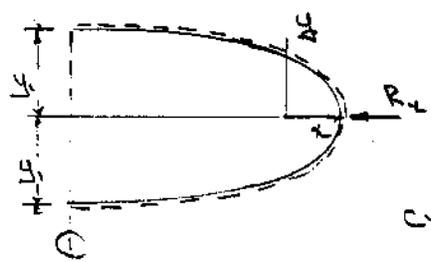
There is no flow across this streamline. The flow in through the left face must be equal to the flow ( $q$ ) which leaves through the sink at the origin.
