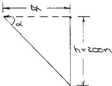
From the instant the aircraft is directly overhead until the Mach cone reaches the ground, the plane travels a distance  $\Delta x$  at speed  $v = 493\text{ m/s}$
