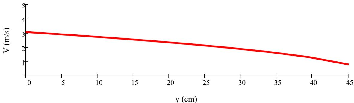
The speed increases as  $y$  decreases because the fluid particles "trade" potential energy for kinetic, just as a falling solid particle does!
