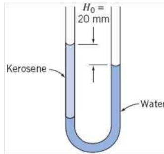
**Given:** Two fluid manometer contains water and kerosene. With both tubes open to atmosphere, the difference in free surface elevations is known
