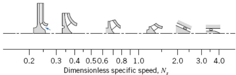
From the figure we see the impeller will be centrifugal
