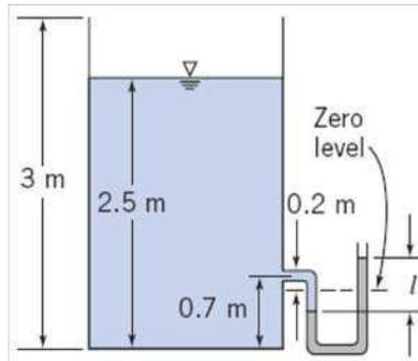
**Given:** A U-tube manometer is connected to the open tank filled with water as shown (manometer fluid is mercury). The tank is sealed and pressurized.
