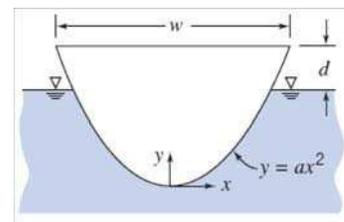
**Given:** Model cross section of canoe as a parabola. Assume constant width  $W$  over entire length  $L$
