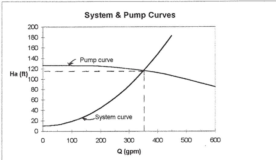
Pump operates at  $Q \approx 350$  gpm.
