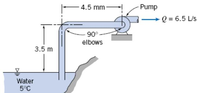
**Given:** Flow out of reservoir by pump
