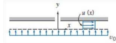
**Given:** Air flow through porous surface into narrow gap
