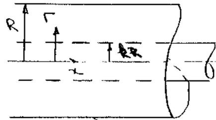
Find an expression for the average velocity. Compare the limiting case,  $k \rightarrow 0$ , with the corresponding expression for flow in a circular pipe.
