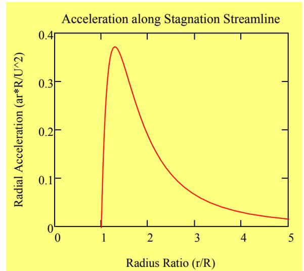
The plots of acceleration along the stagnation streamline and the cylinder surface are shown here. In all cases the accelerations have been normalized by  $U^2/R$
