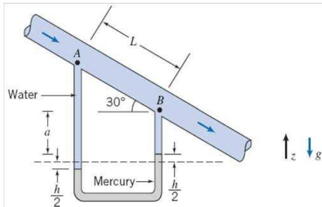
**Given:** Water flow in an inclined pipe as shown. The pressure difference is measured with a two-fluid manometer
