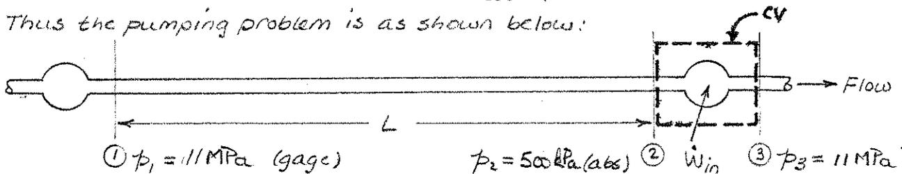
To find  $L$ , apply the energy equation for steady, incompressible flow that is uniform at each section.
