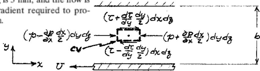
Solution: Apply momentum equation using CV and coordinates shown.
