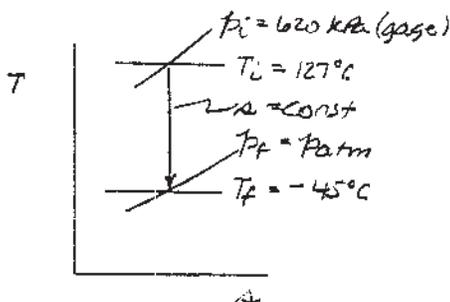
The Ts diagrams for air flowing from the tank are:
