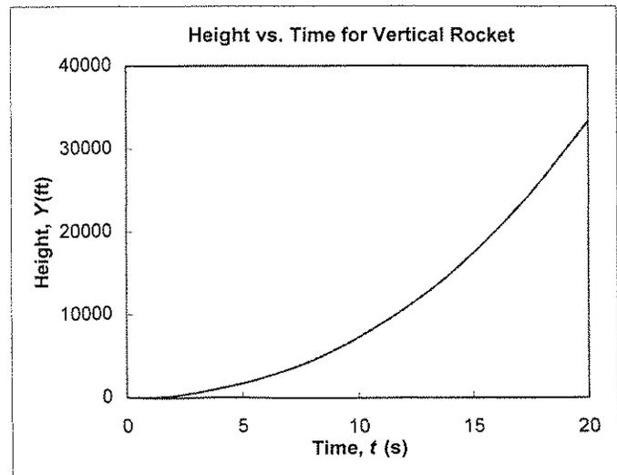
4.169 A large two-stage liquid rocket with mass of 30,000 kg is to be launched from a sea-level launch pad. The main engine burns liquid hydrogen and liquid oxygen in a stoichiometric mixture at 2450 kg/s. The thrust nozzle has an exit diameter of 2.6 m. The exhaust gases exit the nozzle at 2270 m/s and an exit plane pressure of 66 kPa absolute. Calculate the acceleration of the rocket at liftoff. Obtain an expression for speed as a function of time, neglecting air resistance.
