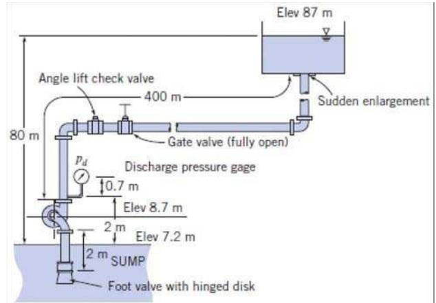
The required pump head is computed and plotted below.
