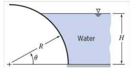
**Given:** Curved surface, in shape of quarter cylinder, with given radius  $R$  and width  $w$ ; water stands to depth  $H$ .
