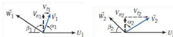
The pump is driven at 1250 rpm while pumping water. Calculate the theoretical head and mechanical power input if the flow rate is 1500 gpm.
