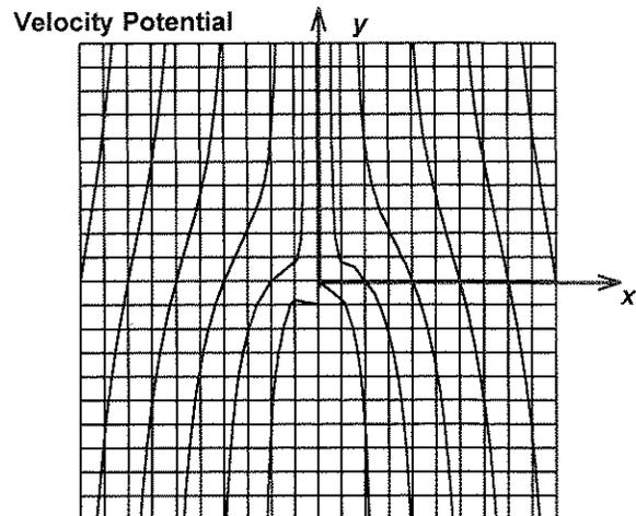
**6.125** Consider the flow field formed by combining a uniform flow in the positive  $x$  direction with a sink located at the origin. Let  $U = 50$  m/s and  $q = 90$  m<sup>2</sup>/s. Use a suitably chosen control volume to evaluate the net force per unit depth needed to hold in place (in standard air) the surface shape formed by the stagnation streamline.
