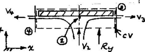
Then  $R_y = V_2 \{ -\rho V_1 A_1 \} + V_3 \{ \rho V_3 A_3 \} + V_4 \{ \rho V_4 A_4 \} = -\rho V_1 A_1 V_2$  and
