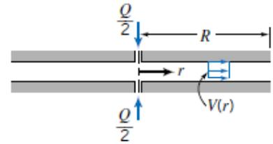
**Given:** Incompressible flow between parallel plates as shown
