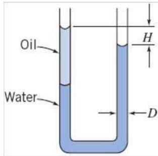
**Given:** U-tube manometer, partially filled with water, then a given volume of Meriam red oil is added to the left side
