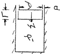
Model the flow as steady, fully developed laminar flow between stationary parallel plates, i.e., neglect motion of the piston.
