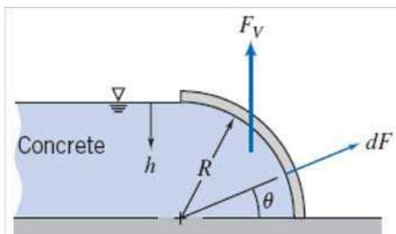
**Given:** Liquid concrete is poured into the form shown
