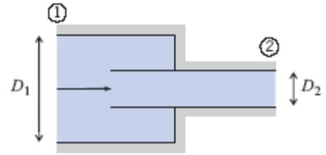
**Given:** Flow through a reentrant device
