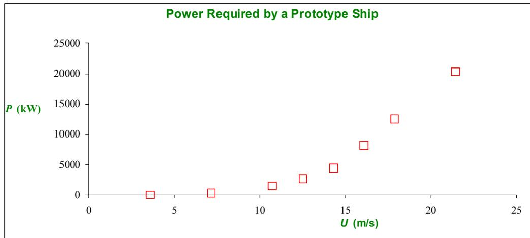
For the prototype wave resistance is a much more significant factor at high speeds! However, note that for both scales, the primary source of drag changes with speed. At low speeds, viscous effects dominate, and so the primary source of drag is viscous drag. At higher speeds, inertial effects dominate, and so the wave drag is the primary source of drag.
