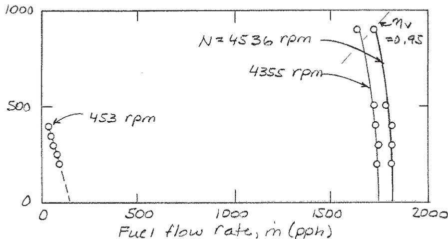
For the pump,  $\dot{m} = \rho \dot{V} N$ , so  $\dot{V} = \frac{\dot{m}}{\rho N}$ . Analyzing the 4536 rpm case,
