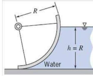
**Given:** Gate formed in the shape of a circular arc has width  $w$ . Liquid is water; depth  $h = R$
