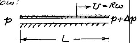
$$\Delta p = \frac{12\mu L}{a^3} \left( \frac{WRa}{2} - \frac{Q}{b} \right) = \frac{6\mu L R \omega}{a^2} \left( 1 - \frac{2Q}{abR\omega} \right)$$
