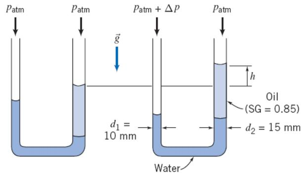
**Given:** U-tube manometer with tubes of different diameter and two liquids, as shown.
