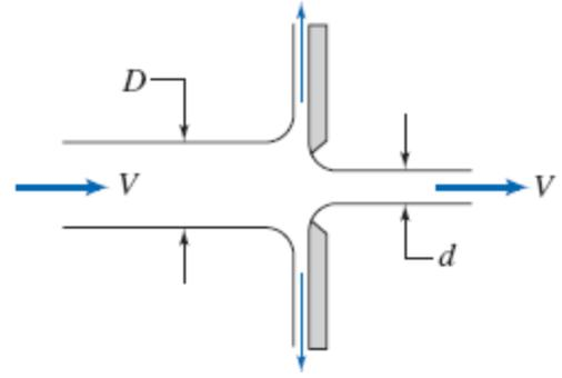
**Given:** Water jet hitting plate with opening
