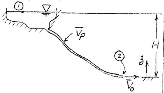
Solution: Apply the energy equation for steady, incompressible pipe flow.
