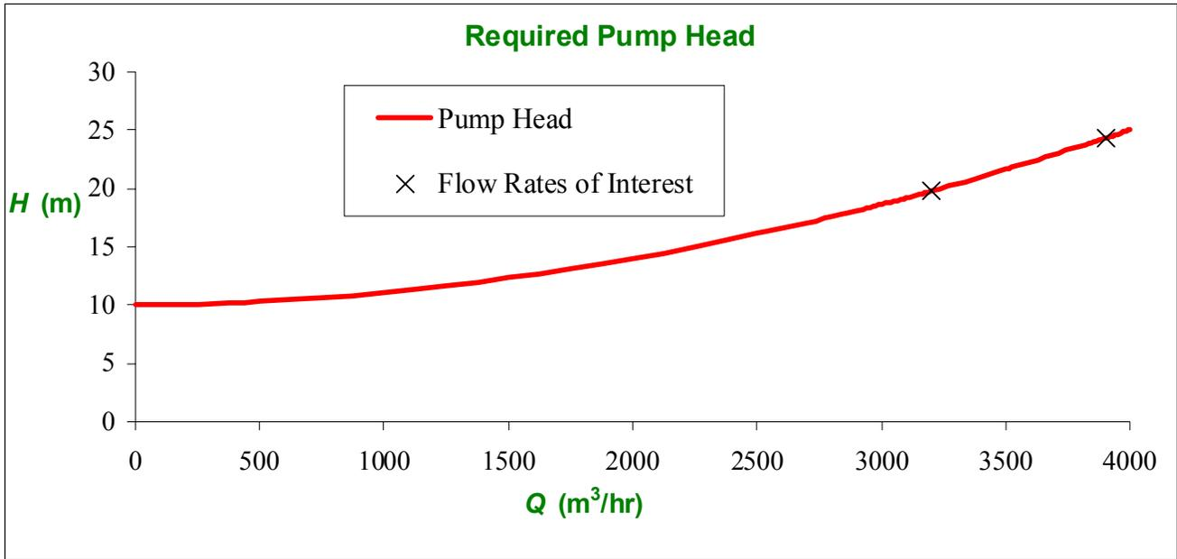
The maximum flow rate is: 17172 gpm
