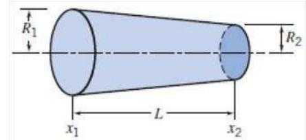
**Given:** One-dimensional, incompressible flow through circular channel.
