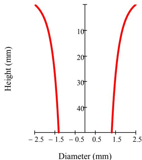
\*4.120 In ancient Egypt, circular vessels filled with water sometimes were used as crude clocks. The vessels were shaped in such a way that, as water drained from the bottom, the surface level dropped at constant rate,  $s$ . Assume that water drains from a small hole of area  $A$ . Find an expression for the radius of the vessel,  $r$ , as a function of the water level,  $h$ . Obtain an expression for the volume of water needed so that the clock will operate for  $n$  hours.
