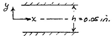
Solution: From Eq. 8.7, with  $a = h$ ,  $u = -\frac{h^2}{8\mu} \frac{\partial p}{\partial x} \left[ 1 - \left( \frac{2y}{h} \right)^2 \right]$ .
