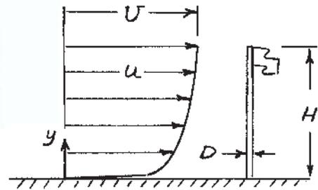
Solution: Apply definition of drag coefficient,  $C_D = \frac{F_D}{\frac{1}{2}\rho V^2 A}$
