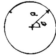
Obtain an expression for the pressure distribution along the streamline forming the cylinder surface,  $r = a$ . Determine the locations where the static pressure on the cylinder is equal to the freestream static pressure.
