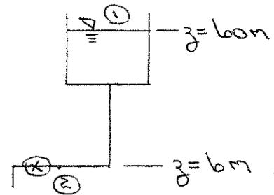
Calculate the initial instantaneous rate of change of volume flow rate.
