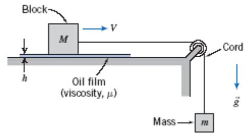
**Given:** Block on oil layer pulled by hanging weight
