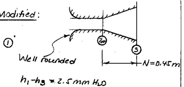
Solution: Apply the energy equation for steady, incompressible pipe flow.
