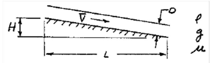
**Given:** Model the motion of a glacier using glycerine. Assume ice as Newtonian fluid with density of glycerine but one million times as viscous. In laboratory test the professor reappears in 9.6 hours.
