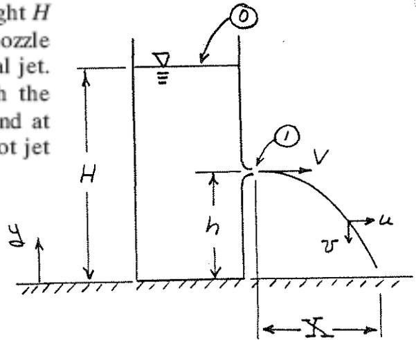
Apply Bernoulli equation between tank surface and jet.
