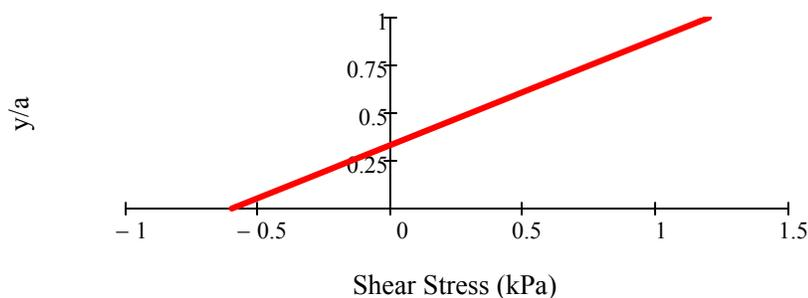
The pressure gradient is adverse, to counteract the flow generated by the upper plate motion
