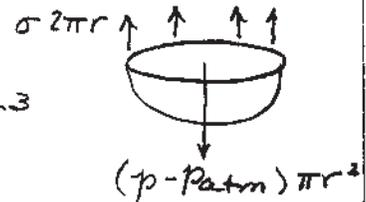
$$(p - p_{\text{atm}}) \pi r^2 = \sigma 2\pi r = k(4\pi r^2) 2\pi r = 8\pi^2 k r^3$$
