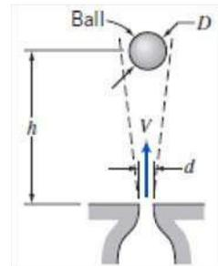
**Given:** Functional relationship between the height of a ball supported by a vertical air jet and other physical parameters
