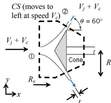
**Given:** Water jet striking moving cone
