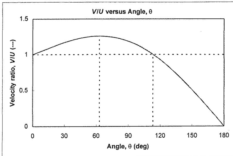
From the plot we see that  $V/U$  is a maximum at  $\theta = 63^\circ$  (also at  $\theta = 297^\circ$  from symmetry with respect to the  $x$  axis).
