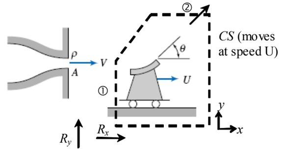
**Given:** Water jet striking moving vane
