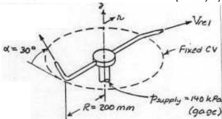
Solution: Apply moment of momentum using fixed CV enclosing sprinkler arms.
