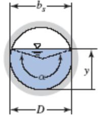
The area is (from simple geometry - a segment of a circle plus two triangular sections)
