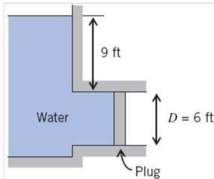
**Given:** Plug is used to seal a conduit.  $\gamma = 62.4 \frac{\text{lb}}{\text{ft}^3}$
