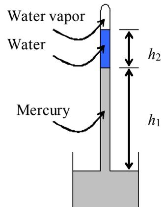
At the higher temperature, the vapor pressure of water increases to 0.60 psi. Therefore, if the atmospheric pressure were to remain constant, the length of the mercury column would have to decrease - the increased water vapor would push the mercury out of the tube!
