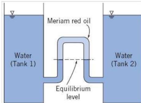
**Given:** Two fluid manometer, Meriam red oil is the second fluid  $SG_{oil} = 0.827$  from Table A.1
