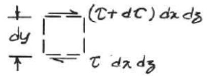
The net shear force on a fluid element is  $d\tau \, dx \, dz$ :  $d\tau = \frac{\partial \tau}{\partial y} \cdot dy = \frac{\mu \cdot U}{\delta} \cdot \left( -\frac{3}{8} \cdot \frac{2 \cdot y}{x^2} \right) \cdot dy = -\frac{3 \cdot \mu \cdot U \cdot y}{4 \cdot \delta \cdot x^2} \cdot dy$
