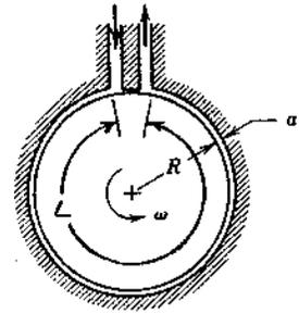
Solution: Since  $a \ll R$ , unwrap to form flow between parallel plates.
