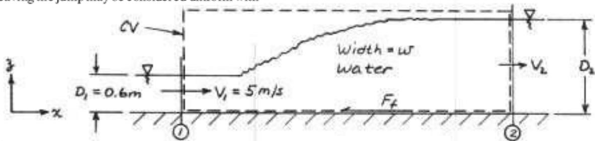
Evaluate the change in mechanical energy through the hydraulic jump. If heat transfer to the surroundings is negligible, determine the change in water temperature through the jump.
