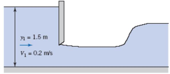
**Given:** Data on sluice gate
