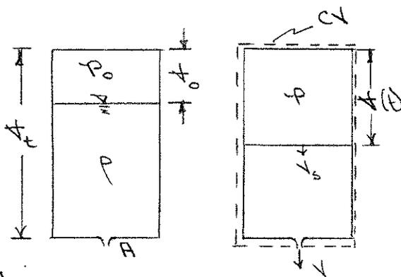
Apply Bernoulli equation between liquid surface and orifice:
