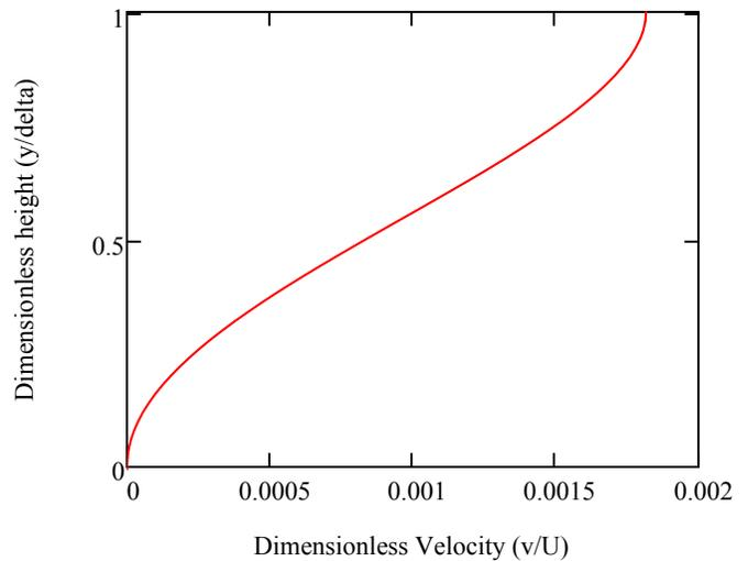
The maximum value of  $v/U$  is where  $y = \delta$ :  $v_{\text{ratmax}} = \frac{v}{U} = \frac{\delta}{\pi \cdot x} \cdot \left( \frac{\pi}{2} \cdot \sin\left(\frac{\pi}{2}\right) + \cos\left(\frac{\pi}{2}\right) - 1 \right) = \frac{\delta}{\pi \cdot x} \cdot \left( \frac{\pi}{2} - 1 \right)$
