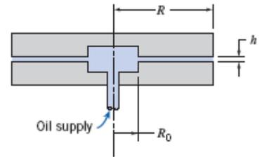
Solution: From the definition of mean velocity,  $Q = \bar{v} 2\pi r h$  so  $\bar{v} = \frac{Q}{2\pi r h}$   $\bar{v}(r)$
