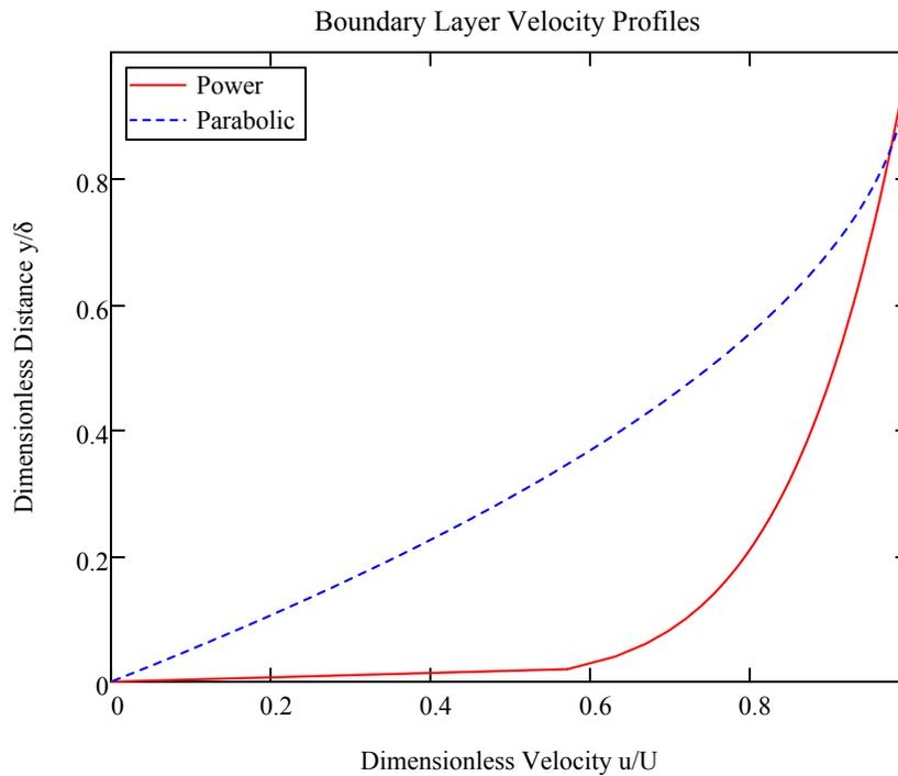
Note that the power law profile gives an infinite value of  $du/dy$  as  $y$  approaches zero:
