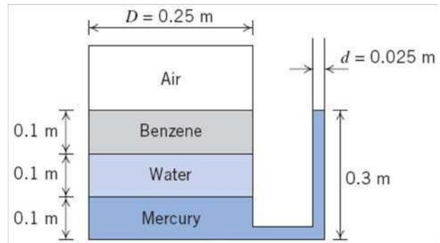
**Given:** Data on fluid levels in a tank
