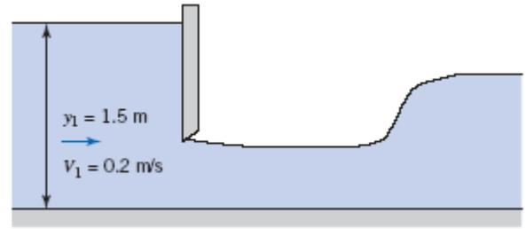
**Given:** Data on sluice gate
