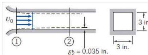
**Given:** Data on wind tunnel and boundary layers
