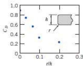
Drag coefficient v. radius ratio [37]
