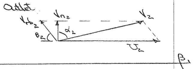
From the outlet diagram,  $v_{t2} = U_2 - v_{n2} \cot \beta_2 = 23.8 \frac{\text{m}}{\text{s}} - 4.24 \frac{\text{m}}{\text{s}} \times \frac{1}{\tan 40^\circ}$
