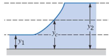
**Given:** Data on rectangular channel and hydraulic jump
