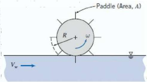
Solution: Computing equations  $F_D = C_D A \frac{1}{2} \rho V_{rel}^2$
