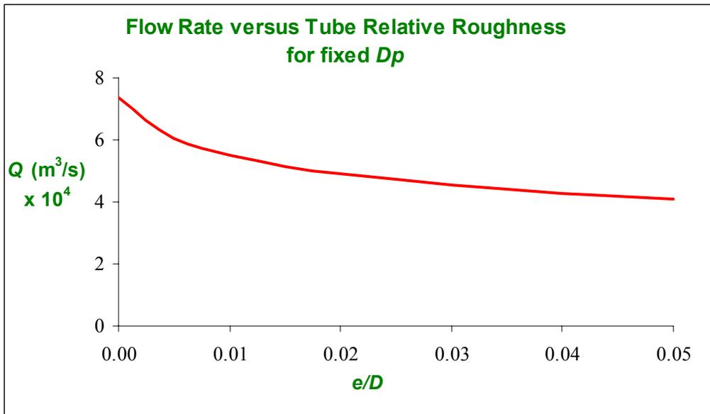
It is not possible to roughen the tube sufficiently to slow the flow down to a laminar flow for this  $\Delta p$ . Even a relative roughness of 0.5 (a physical impossibility!) would not work.
