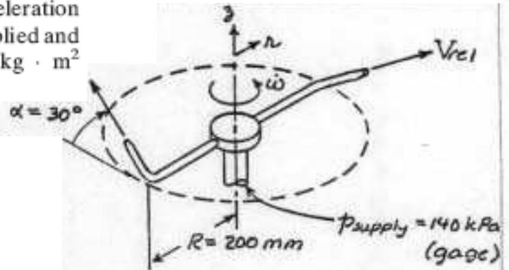
Solution: Apply moment of momentum using fixed CV enclosing sprinkler arms.
