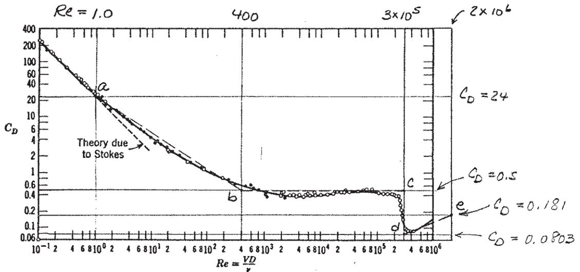
The maximum significant error occurs in the region where  $C_D$  is modeled as equal to the constant value,  $C_D = 0.5$ . The curve fit appears to be about 10 percent high in the region from  $Re \approx 10^3$  to  $Re \approx 10^4$ .
