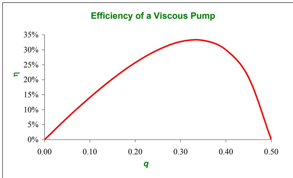
For the maximum efficiency point we can use *Solver* (or alternatively differentiate)
