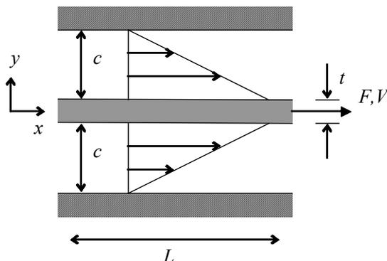
The given data is  $F_T = 25 \cdot \text{lbf}$      $c = 0.012 \cdot \text{in}$      $\mu = 0.02 \cdot \frac{\text{slug}}{\text{ft} \cdot \text{s}}$      $V = 3 \cdot \frac{\text{ft}}{\text{s}}$      $w = 1 \cdot \text{in}$
