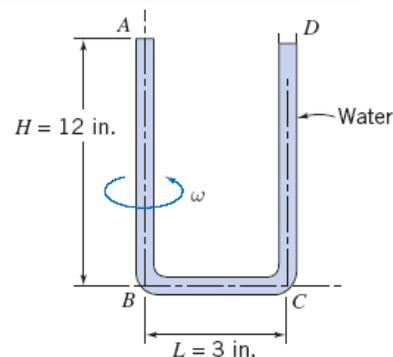
**Given:** Spinning U-tube sealed at one end
