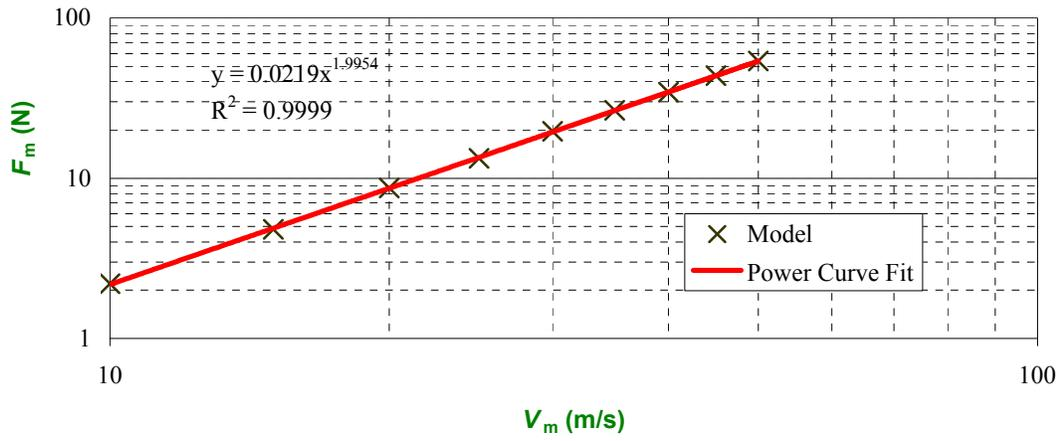
Lift vs Speed for an Airplane Prototype (Log-Log Plot)
