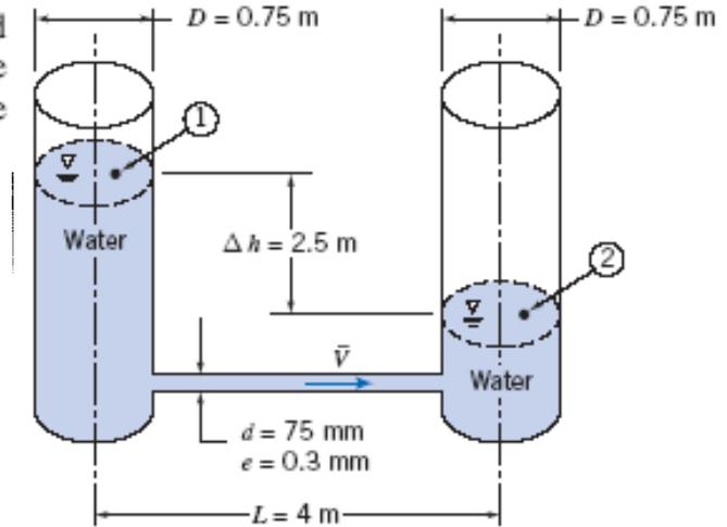
Solution: Apply the energy equation for quasi-steady, incompressible pipe flow.
