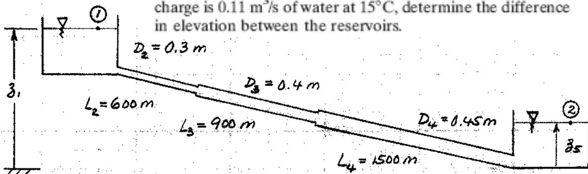
Solution: Apply the energy equation for steady, incompressible flow that is uniform at each section.
