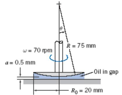
**Given:** Geometry of rotating bearing
