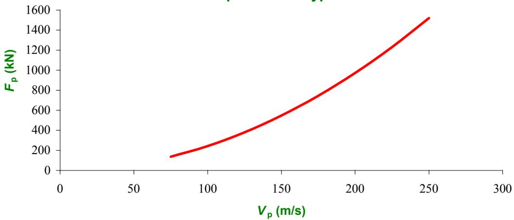
Lift vs Speed for an Airplane Model
