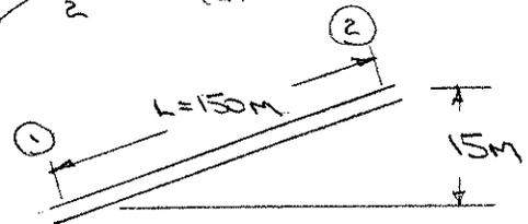
For cast iron pipe with  $D = 125 \text{ mm}$ ,  $\frac{e}{D} = 0.0021$  ( $e = 0.26 \text{ mm}$ , Table 8.1)
