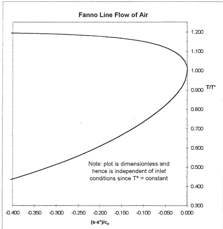
13.141 Air flows through a 40 ft length of insulated constant-area duct with  $D = 2.12$  ft. The relative roughness is  $e/D = 0.002$ . At the duct inlet,  $T_1 = 100^\circ\text{F}$  and  $p_1 = 17.0$  psia. At a location downstream,  $p_2 = 14.7$  psia, and the flow is subsonic. Is sufficient information given to solve for  $M_1$  and  $M_2$ ? Prove your answer graphically. Find the mass flow rate in the duct and  $T_2$ .
