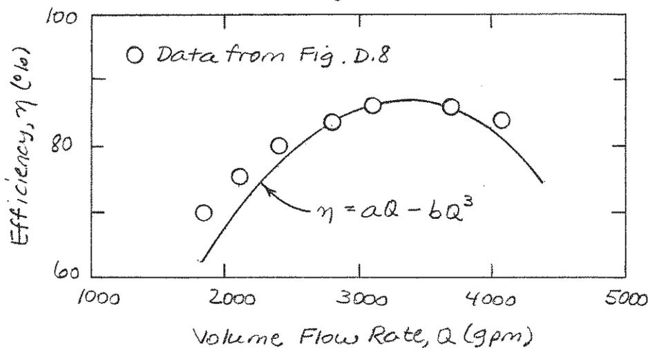
The curve-fit does a good job near peak efficiency, but tends to underestimate the measured data elsewhere.
