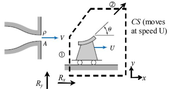
**Given:** Water jet striking moving vane
