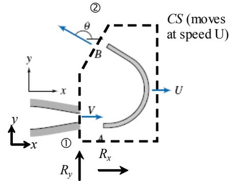
**Given:** Water jet striking moving vane
