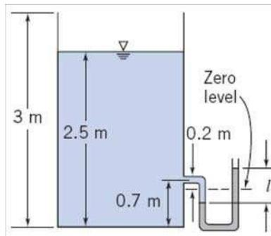
**Given:** Sealed tank is partially filled with water. Water drains slowly from the tank until the system attains equilibrium. U-tube manometer is connected to the tank as shown. (Meriam blue in manometer)
