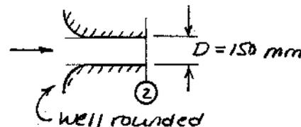
Solution: Apply the energy equation for steady, incompressible pipe flow.
