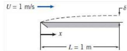
**Given:** Turbulent boundary layer flow of water, 1/7-power profile
