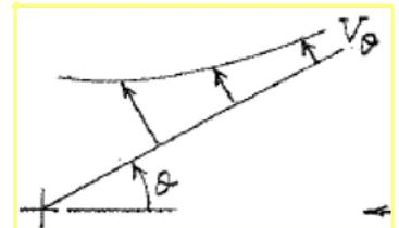
$Q = \int_{r_1}^{r_2} V_\theta dr = \int_{r_1}^{r_2} \frac{C}{r} dr = C \cdot \ln\left(\frac{r_2}{r_1}\right)$  Substituting known values:  $Q = 0.3 \cdot \frac{\text{m}^2}{\text{s}} \times \ln\left(\frac{0.24}{0.20}\right)$   $Q = 0.0547 \cdot \frac{\text{m}^3}{\text{s} \cdot \text{m}}$
