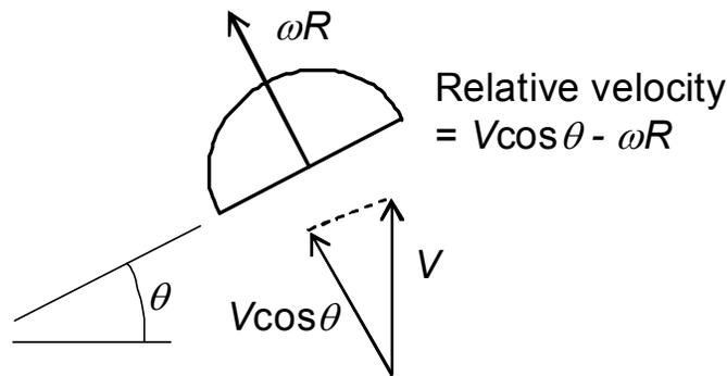
In this more sophisticated analysis we need to compute the instantaneous normal relative velocity. From the sketch, when a cup is at angle  $\theta$ , the normal component of relative velocity is
