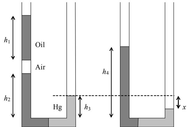
**Given:** Data on manometer before and after an "accident"
