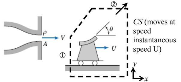
**Given:** Water jet striking moving vane/cart assembly
