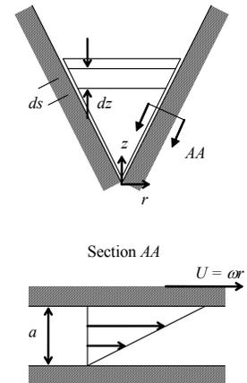
As we move up the device, shear stress increases linearly (because rate of shear strain does)
