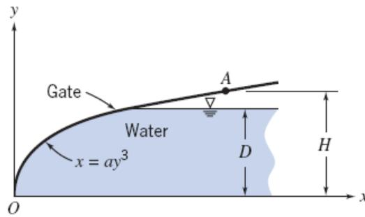
**Given:** Parabolic gate, hinged at  $O$  has a constant width.
