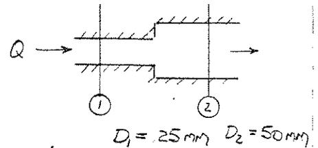
Solution: Apply energy equation for pipe flow.
