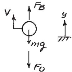
Then  $-\rho V g + \rho_{H_2O} V g - 3\pi\mu V_t D = 0$  at terminal speed,  $V_t$ .
