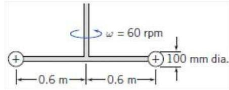
**Given:** Rotary mixer rotated in a brine solution
