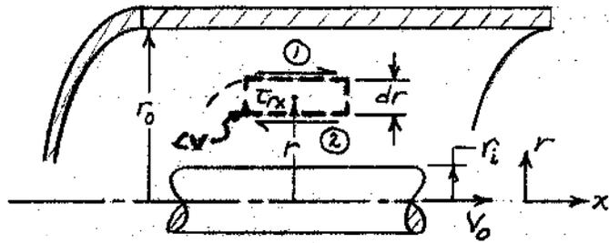
Solution: Apply  $x$  component of momentum equation, using annular CV shown.
