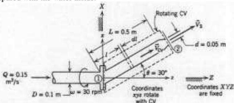
Find: (a) Torque required to drive the nozzle assembly
