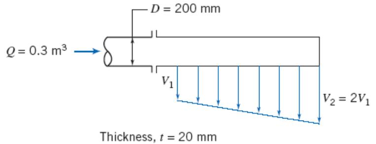
**Given:** Data on flow out of pipe device
