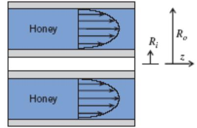
Show that the no-slip condition is satisfied by this expression. Find the location at which the shear stress is zero. Find the viscous forces acting on the inner and outer surfaces, and compare these to the force  $\Delta p \pi (R_o^2 - R_i^2)$ . Explain.
