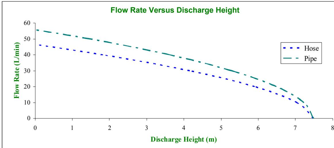
The results show that the 15% performance loss is an okay "ball park" guess at the lower flow rates, but not very good at flow rates above 30 L/min.
