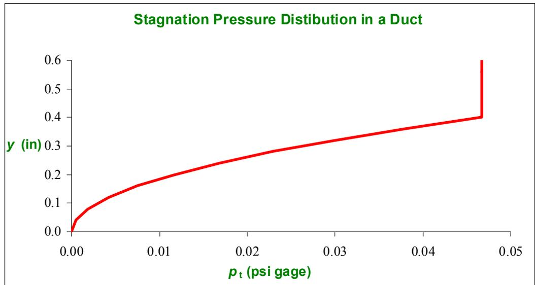
The stagnation pressure indicates total mechanical energy - the curve indicates significant loss close to the walls and no loss of energy in the central core.
