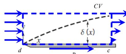
Assumptions: 1) Steady flow 2) No pressure force 3) No body force in  $x$  direction 4) Uniform flow at  $ab$
