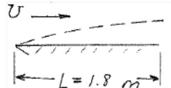
$$\frac{\delta_{\text{disp}}}{\delta} = \int_0^1 \left(1 - \frac{u}{U}\right) d\eta \quad (\text{Displacement thickness})$$
