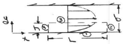
**Given:** Velocity field for pressure-driven flow between stationary parallel plates
