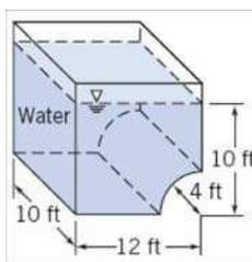
**Given:** Open tank as shown. Width of curved surface  $b = 10 \cdot \text{ft}$
