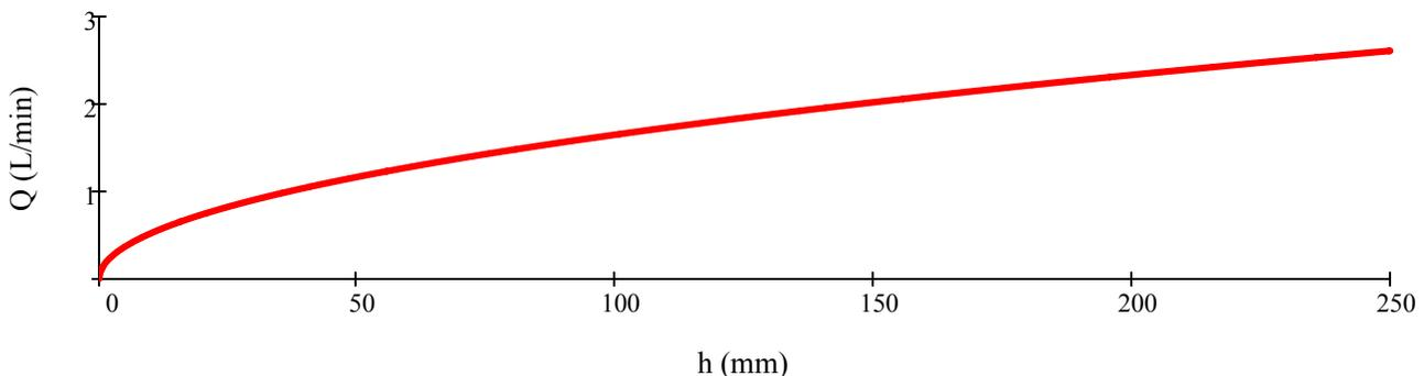
For a flow rate of  $Q = 2 \cdot \frac{\text{L}}{\text{min}}$   $Q = 3.33 \times 10^{-5} \frac{\text{m}^3}{\text{s}}$  solving for  $h$   $h = \frac{8 \cdot Q^2}{\pi^2 \cdot D^4 \cdot g}$   $h = 147 \cdot \text{mm}$
