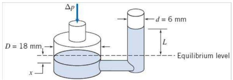
**Given:** Reservoir manometer with vertical tubes of known diameter. Gage liquid is Meriam red oil
