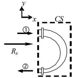
**Given:** Water flow through elbow
