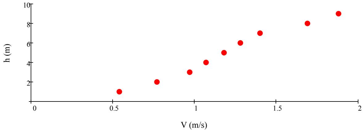
This does not seem like an unreasonable profile for the lowest portion of an atmospheric boundary layer - over cities or rough terrain the atmospheric boundary layer is typically 300-400 meters, so a near-linear profile over a small fraction of that distance is not out of the question.
