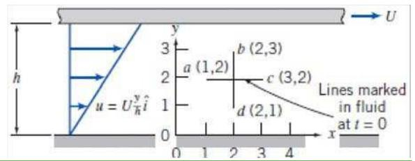
**Given:** Viscometric flow of Example 5.7,  $V = U(y/h)i$ , where  $U = 4 \text{ mm/s}$  and  $h = 4 \text{ mm}$
