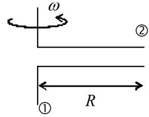
**Given:** Centrifugal manometer consists of pair of parallel disks that rotate to develop a radial pressure difference. There is no flow between the disks.
