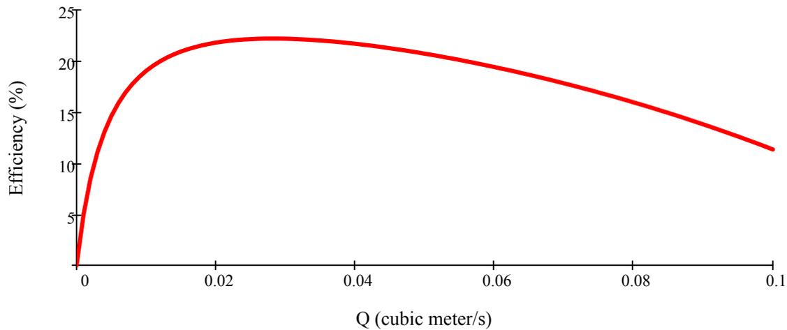
The above graph can be plotted in Excel. In addition, Solver can be used to vary Q to maximize  $\eta$ . The results are
