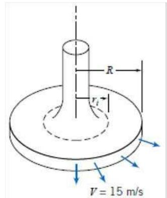
**Given:** Incompressible, inviscid flow of air between parallel disks
