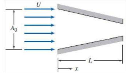
**Given:** Velocity field and nozzle geometry
