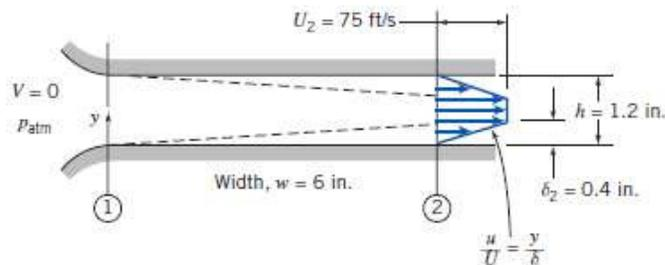
**Given:** Data on flow in a channel
