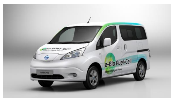
Figure 1: Ethanol on board reformer-fuel cell by Nissan being tested in Brazil. Source [12].
