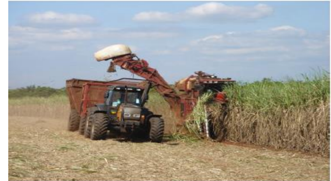
Fig. 3.12 Mechanical harvesting of green cane. (Photo courtesy of Agricef Soluções Tecnológicas Para Agricultura Ltda, Brazil; reprinted with permission)
