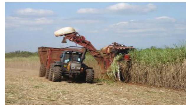
Fig. 3.12 Mechanical harvesting of green cane. (Photo courtesy of Agricef Soluções Tecnológicas Para Agricultura Ltda, Brazil; reprinted with permission)
