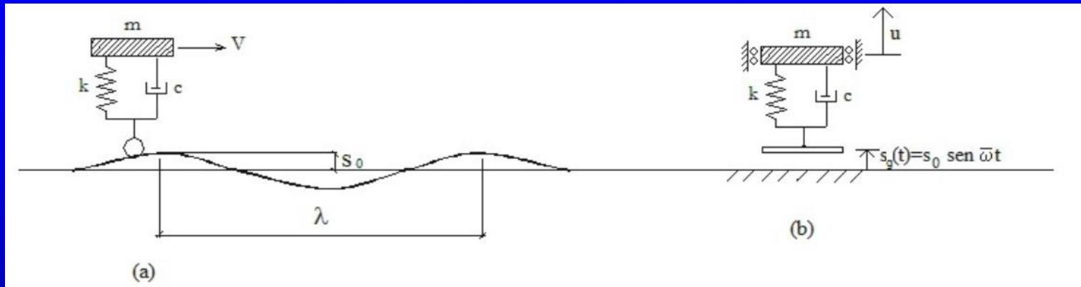
$$m = 1200 \text{ kg}, c = 10450 \text{ Ns/m} \text{ e } k = 148650 \text{ N/m}$$
