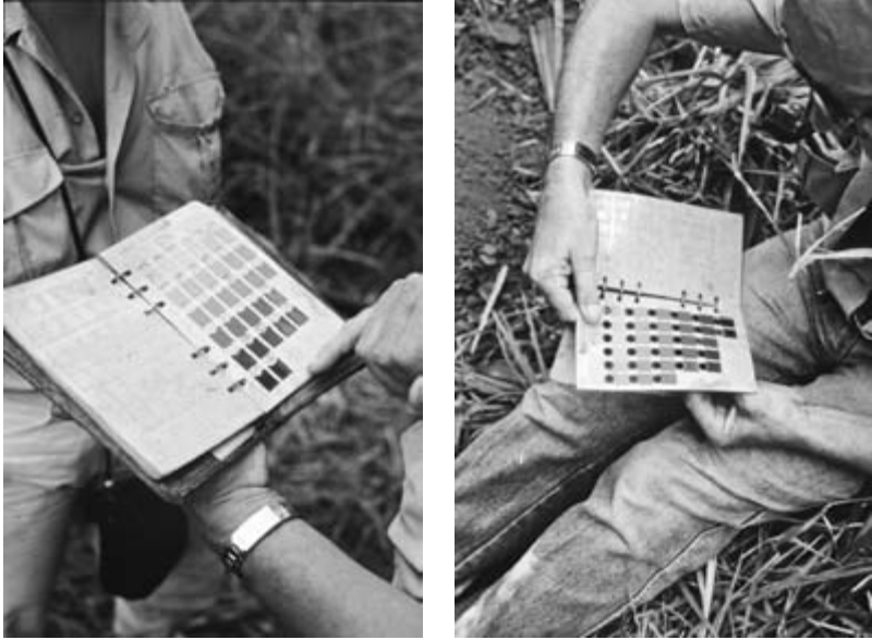
1.5-1.6 Use in the field of Munsell's charts to identify the color of a soil sample. Latour (1995) argues that this is one of the ways in which pedologists practically establish references between their final soil report and the original encounter with the forest. Courtesy of Bruno Latour.
