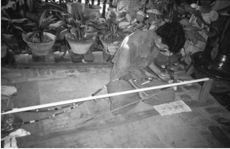
2.3 Preparing yarn for resist dyeing, Amarapura, central Burma (Myanmar). In Burmese textile workshops this is a skilled job, usually undertaken by men. Note the use of a paper pattern. Photo: Sandra Dudley, 1996.
