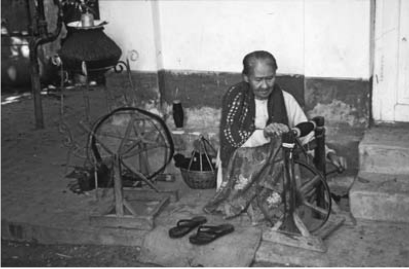
2.2 Winding yarn onto a spool, Amarapura, central Burma (Myanmar). Photo: Sandra Dudley, 1996.
