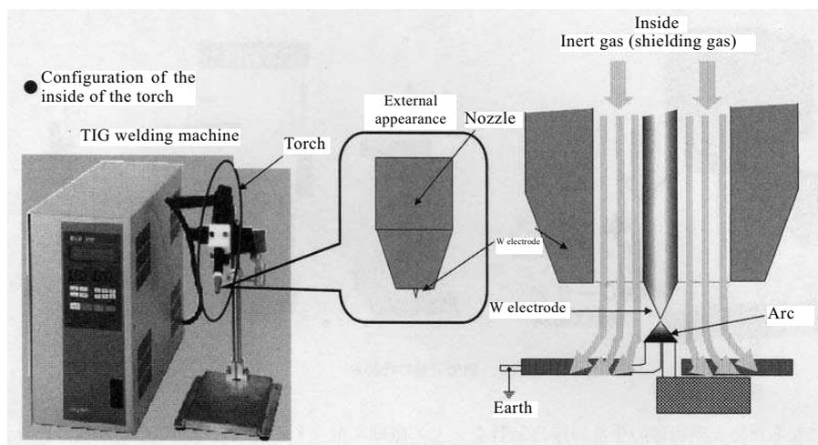
Figure 3. Principle of TIG welding.
