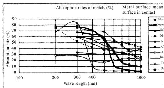
Figure 1. Absorption rates of metals.
