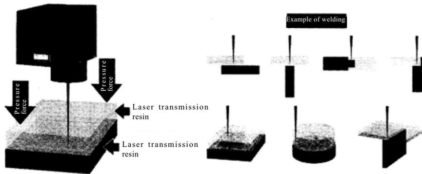
Figure 2. How resin welding works.
