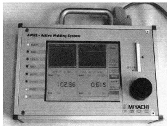
Photo 5. Process control unit (enables all together the setting and judging of checking conditions, the setting of pressurising process and the setting of the conditions for welding power).
