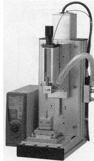
Photo 4. Motor driven welding pressure mechanism [MH-110A].
