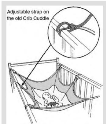
**Figure 11.13** (Consumer Product Safety Commission) The “Crib Cuddle” was recalled after reports of infant injuries and death. It is similar to a hammock that attaches to the side rails of a crib by six adjustable straps. A plastic heart-shaped battery-operated box pulsates and vibrates to simulate a heartbeat and is inserted into a soft pad in the hammock.
