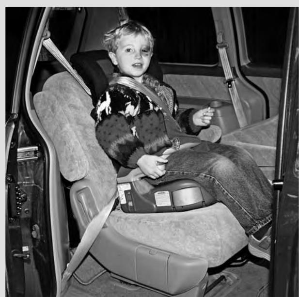
**Figure 17.23** (Ursy Potter Photography) Children should start using booster seats when they grow out of their child safety seats. When used properly, these raise the child so that the combined lap and shoulder belt fit correctly.
