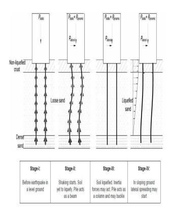
Different stages of loading in the pile during earthquake (after Bhattacharya, 2008)
