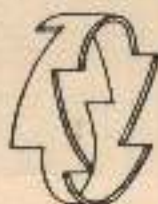
Better: Staggered teeth give more even section.
