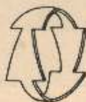
Wrong: uneven section if teeth are opposite.
