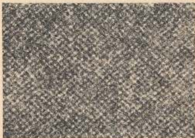
Fig. 21.9 (b) Structure is mainly fine untempered martensite with a few spheroids of cementite
