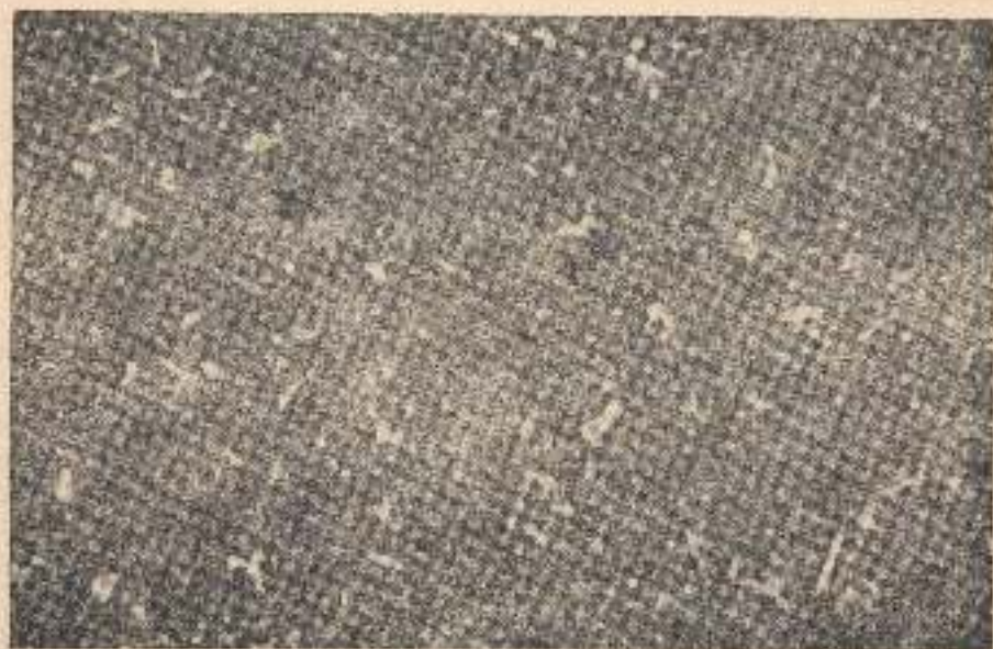
Fig. 22.39(f) Same steel tempered again at 550°C for 1 h. The structure consists of large and small alloy carbide particles in a matrix of tempered martensite (Courtesy: Speed Steel, Sweden)
