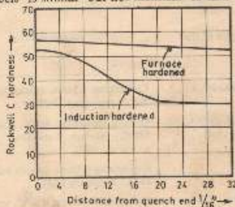
Fig. 15.19. Comparison of transformation characteristics of steel AISI 4340, as developed by end-quenched specimens that are induction and flame hardened
