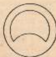
Wrong: sharp corners and big differences in section.
