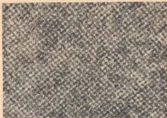
Fig. 21.9 (b) Structure is mainly fine untempered martensite with a few spheroids of cementite
