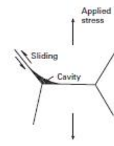
Fig. 8.7 w-type cavitation at a grain-boundary triple point.
