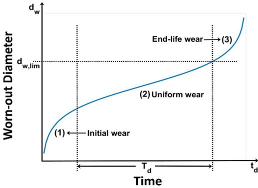
Figure 1. Tool wear during a grind wheel life
