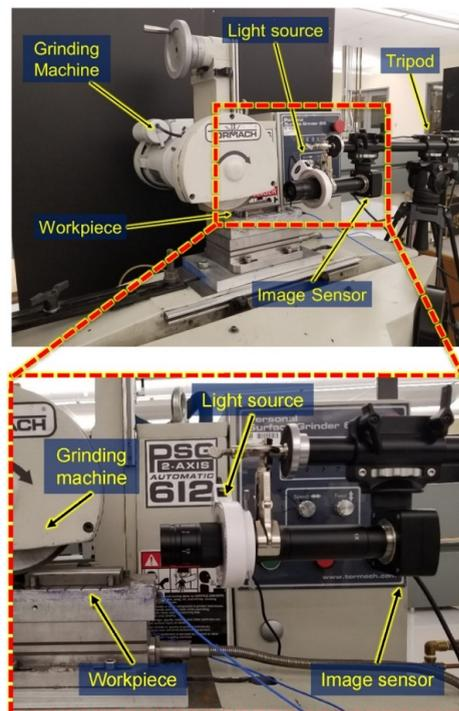
Figure 4. Experimental setup
