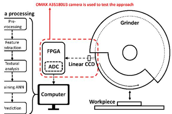
Figure 2. Proposed 1D image sensing system for tool wear monitoring
