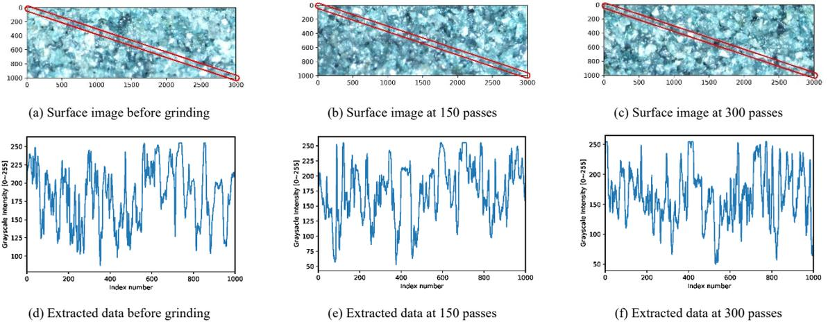
Figure 5. Pre-processing for the feature extraction at before grinding, 150 passes, 300 passes of grinding process
