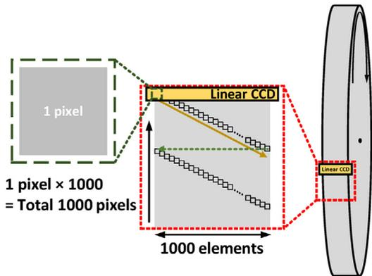
Figure 3. Capturing surface images from the grinding wheel
