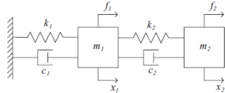
$$m_1\ddot{x}_1 + (c_1 + c_2)\dot{x}_1 - c_2\dot{x}_2 + (k_1 + k_2)x_1 - k_2x_2 = f_1(t)$$
