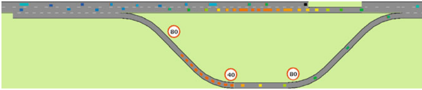
Fig. 21.5 Screenshot of the “routing game” developed with the open-source traffic simulator MovSim. The player can reroute the drivers on the right lane of the main-road over a deviation on the secondary network to prevent a breakdown at the lane-closing bottleneck. Here, the player adopted a sub-optimal strategy and caused jams on both routes
